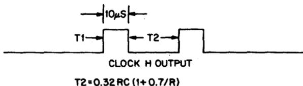
$T2$  is in seconds,  $R$  is in ohms, and  $C$  is in farads. The internal potentiometer varies between 5.1K and 50K ohms.
