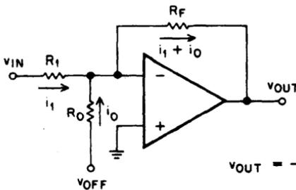
$$V_{OUT} = -V_{IN} \left( \frac{R_F}{R_1} \right) + \underbrace{\left[ -V_{OFF} \left( \frac{R_F}{R_O} \right) \right]}_{\text{OFFSET}}$$
