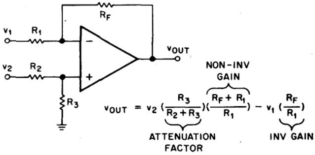
Fig. 9, Differential Gain
