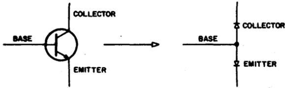
Figure 2 Two Diode Model For Transistor
