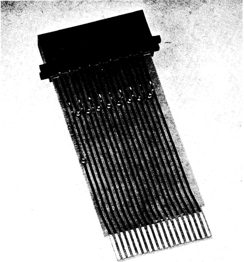
The W980 Module Extender allows access to the module circuits without breaking connections between the module and mounting panel wiring.
