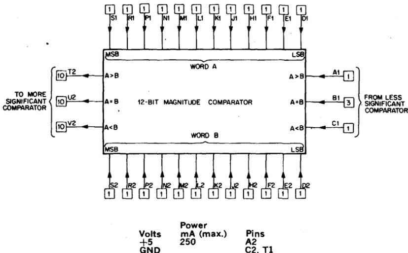
The M168 12-Bit Magnitude Comparator performs magnitude comparison of two 12-bit words. When the comparison inputs are not connected to the comparison outputs of another M168, the "A=B" input must be connected to a logical "1". The A>B and A<B inputs may individually be made a logic "1" or logic "0". However, connecting both these inputs to GND, a logic "0" is recommended.
