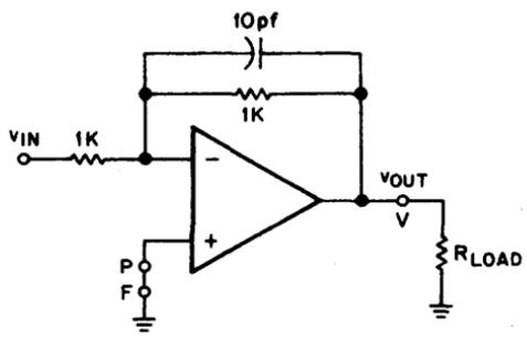
$$\frac{V_{OUT}}{V_{IN}} = - 1$$
