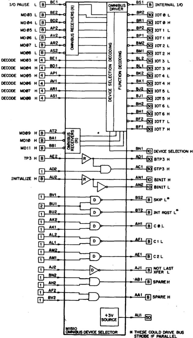
The M1510 Bus Device Selector is designed for use with the PDP-8/e and PDP-8/m computers. It provides a convenient and efficient method of decoding the device code for an interface system. The M1510 decodes the six device selection bits to produce a device selection level. It also decodes the three function selection bits to produce a one-of-eight function level output.
