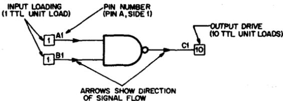
Figure 1. Logic Diagram Input Loading and Output Drive Symbols
