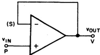
$$\frac{V_{OUT}}{V_{IN}} = + 1$$
