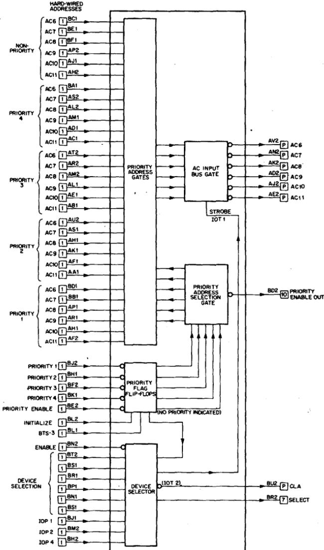
The M736 is used in conjunction with the PDP8/I or 8/L to provide the capability of assigning priorities to various I/O devices connected to the I/O bus of the computer. The M736 can be used to assign priorities for one thru four external devices. Priority assignment may be provided for more than four devices by using additional M736 modules for each additional group of four devices. All M736's in a particular priority system would utilize the same device code.
