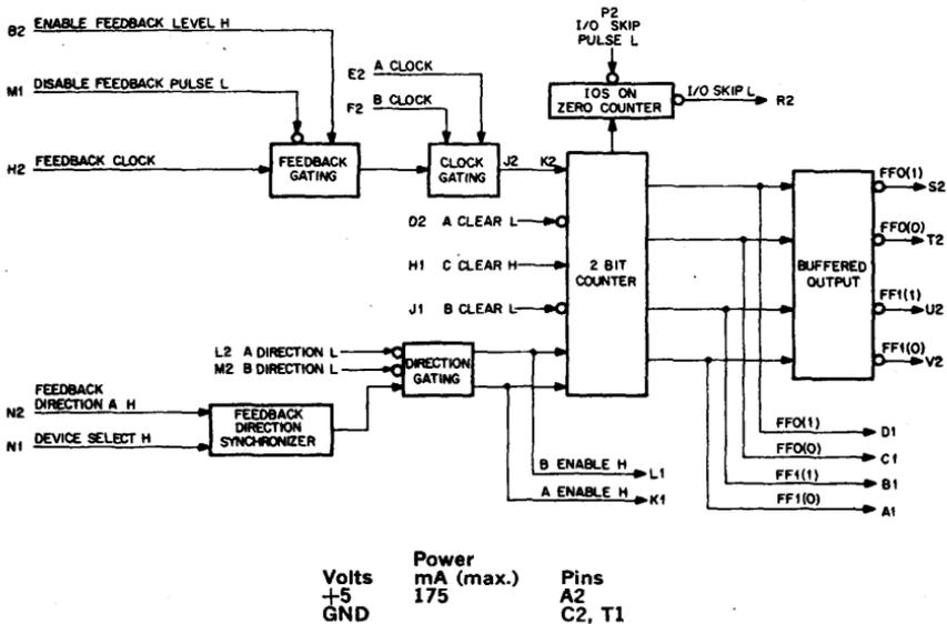
The M261 motor translator will develop the sequence of patterns necessary to step a Sigma or Superior Electric type stepping motor (4 winding). It is a 2-bit switch-tail ring counter which, if initially cleared, would be in state 1. (Fig. 1)
