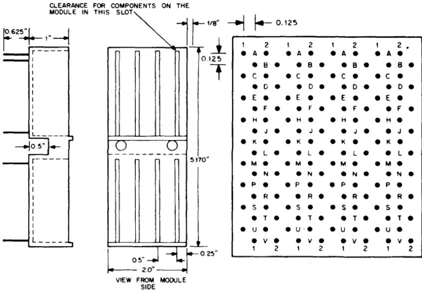
The H803 is the 8-module molded Connector Assembly used in the H911 mounting panels. For each of the eight modules, it provides a 36-pin connector with the wirewrap pins forming a 0.125-inch staggered grid as shown above. This connector is designed to be used with M Series modules; however, it can also be used with all other series listed in this handbook.
