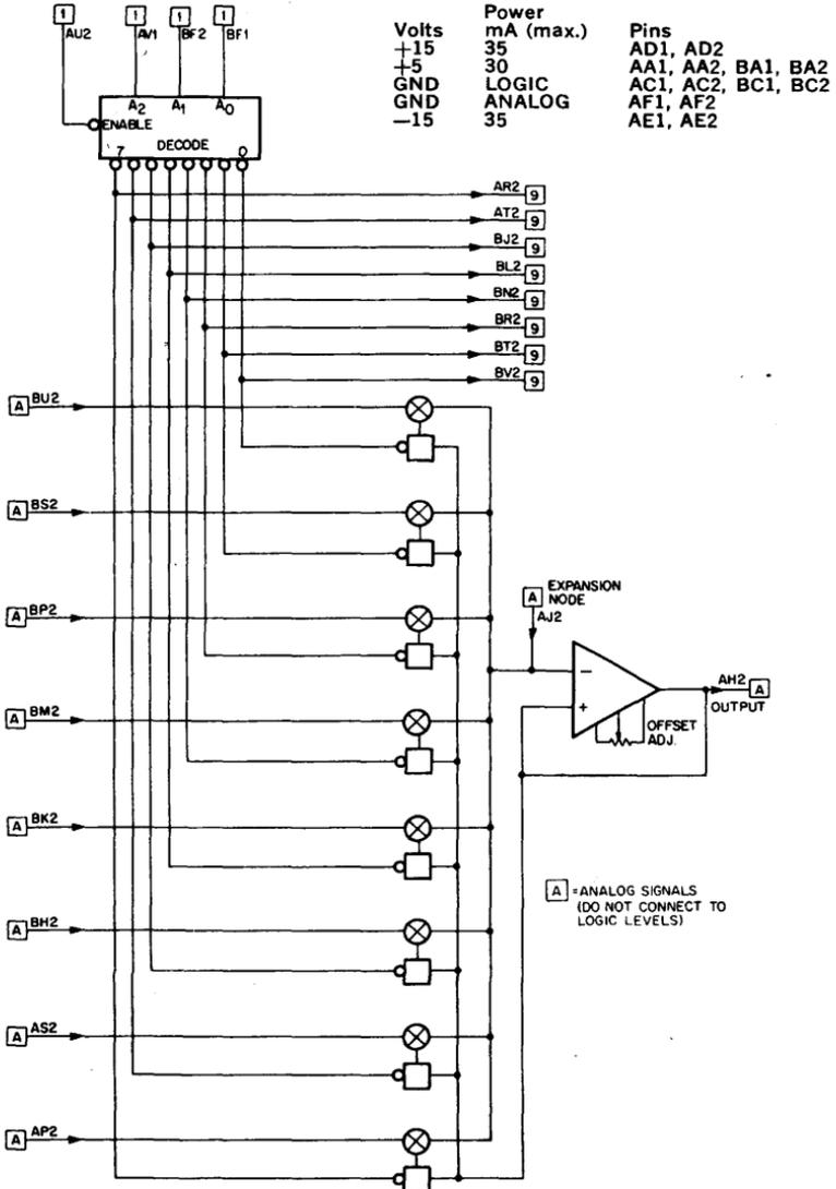
The A163 is a high impedance multiplexer consisting of 8 FET switched channels, a noninverting unity gain follower amplifier, and an 8 bit binary to octal decoder for channel selecting.
