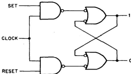
Figure 13 Clocked NAND Gate Flip-Flop
