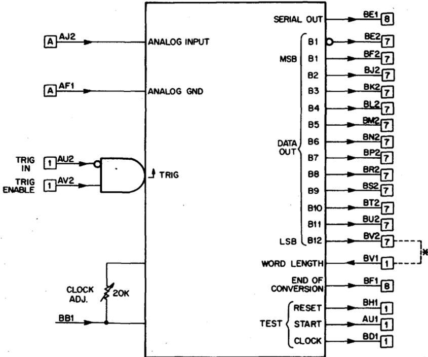
\* = MUST BE CONNECTED TO ONE OF THE DATA OUT BITS.
