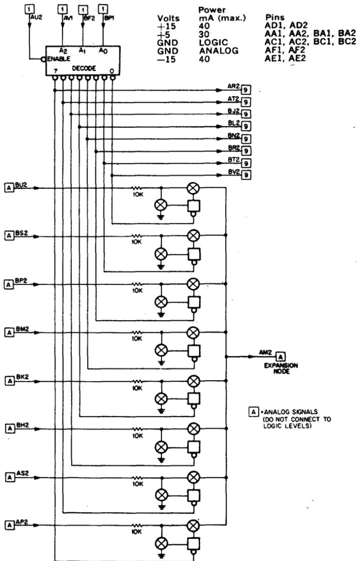
The A166 is a constant impedance eight channel multiplexer with decoder.
