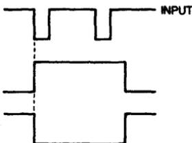
This circuit is insensitive to input transitions during its timeout period as shown in the example above.
