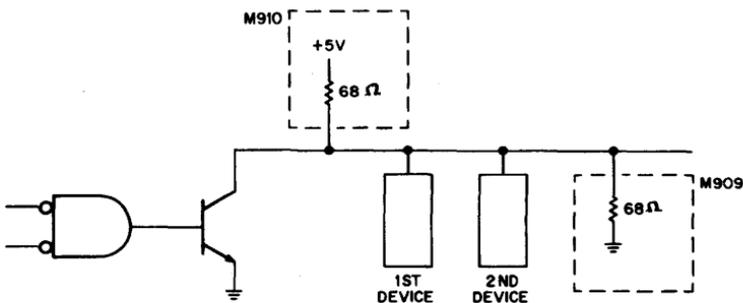
Pull-up resistors of 68 ohms to +5.0 V (supplied on M910) must be tied to the output and the last device should terminate all lines to ground with a 68-ohm resistor (supplied on M909).
