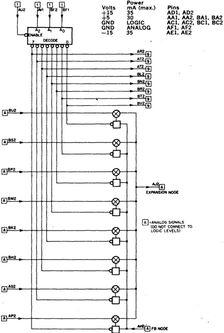
The A162 is a high impedance multiplexer with decoder consisting of 8 independent FET switched channels. Included on this module is a gated binary to octal decoder for selecting any of the eight high speed channels.
