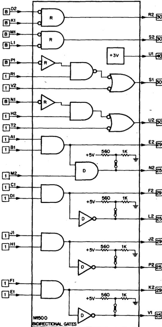
This module provides gating arrangements useful for interfacing to the PDP-8/e, PDP-8/m and PDP-11 computers. It is designed specifically to provide additional gating and output drive when using the M1501-M1502 Input/Output modules. Examples are shown in Figures 1 and 2.
