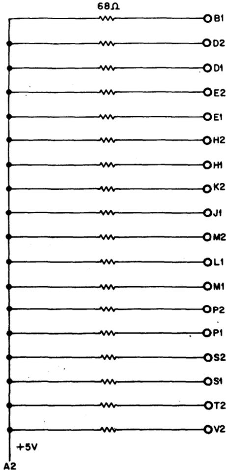
The M910 module contains eighteen 68-ohm resistors tied to a common +5 volt bus.
