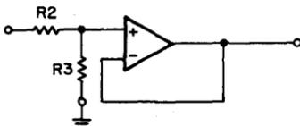
$$\frac{E_O}{E_{IN}} = \frac{R_3}{R_3 + R_2}$$
