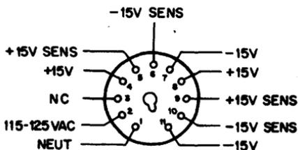
The H704 and H707 contain two 15 Volt floating power supplies. To get  $\pm 15$  Volt supply, connect pins 7 and 8 and use this point as ground. Pin 4 will now be at positive 15 Volts and pin 11 will be negative 15 Volts.
