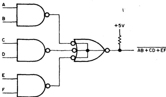
By using one of the two inverters provided, a true AND/OR function can be realized. A maximum of four groups of gates can be connected together. Connection is made by merely connecting output pins together.
