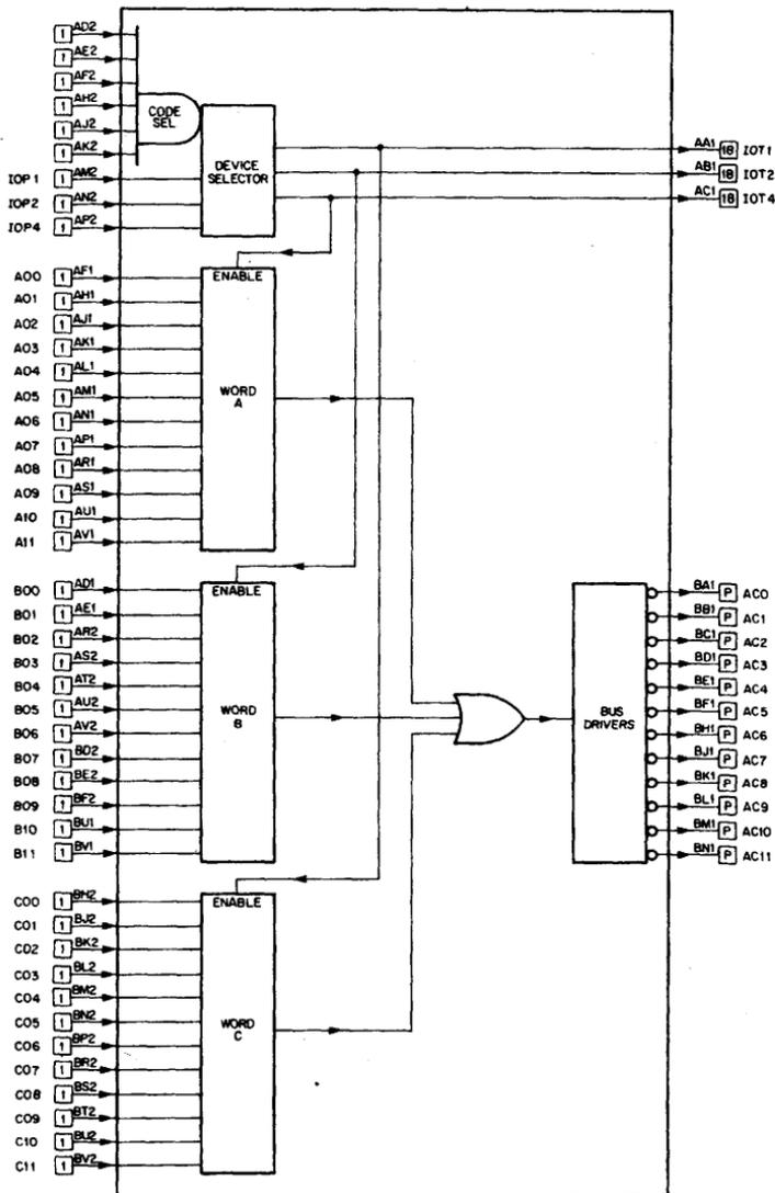
The M734 is a three-word multiplexer used for strobing 12-bit words on a positive voltage input bus, usually the input of the PDP-8/I or the PDP-8/L. Device selector gating is provided. The data outputs of the M734 Multiplexer consist of open collector NPN transistors which allow these outputs to be directly connected to the bus.
