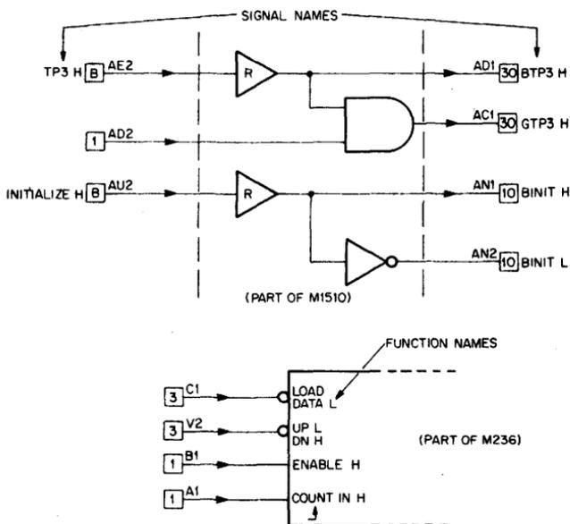
Figure 5. Signal and Function Names
