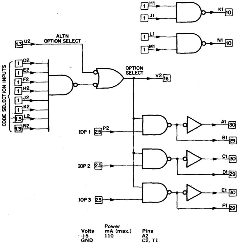
The M103 is used to decode the six device bits transmitted in complement pairs on the positive bus of the PDP8/1 and PDP8/L. Selection codes are obtained by selective wiring of the bus signals to the code select inputs D2, E2, F2, H2, J2, and K2. This module also includes pulse buffering gates for the IOP signals found on the positive bus of the above computers. Two two-input NAND gates are also provided for any additional buffering that is required.
