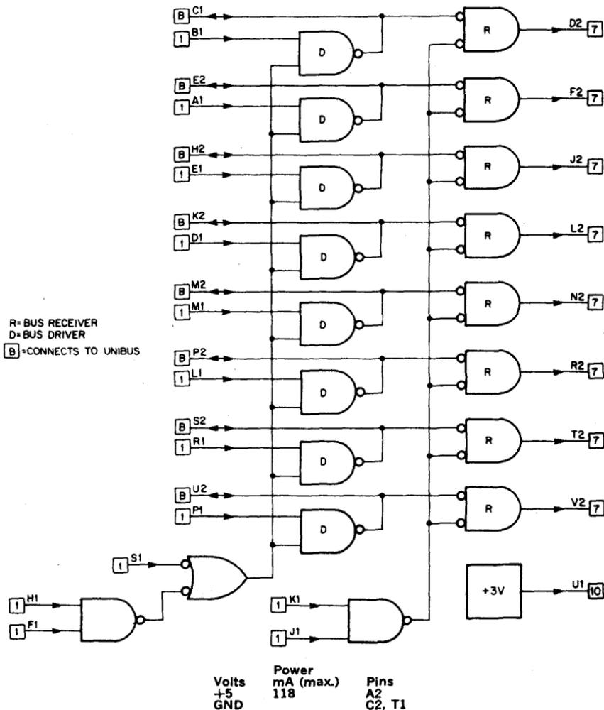
The M785 consists of eight drivers and eight receivers for use as a device interface with the PDP-11 UNIBUS. Pin U1 provides +3 volts and has an output capability of 10 TTL loads. Driver gates have open collectors and are capable of sinking 50 mA with a collector voltage of less than 0.8 volts.
