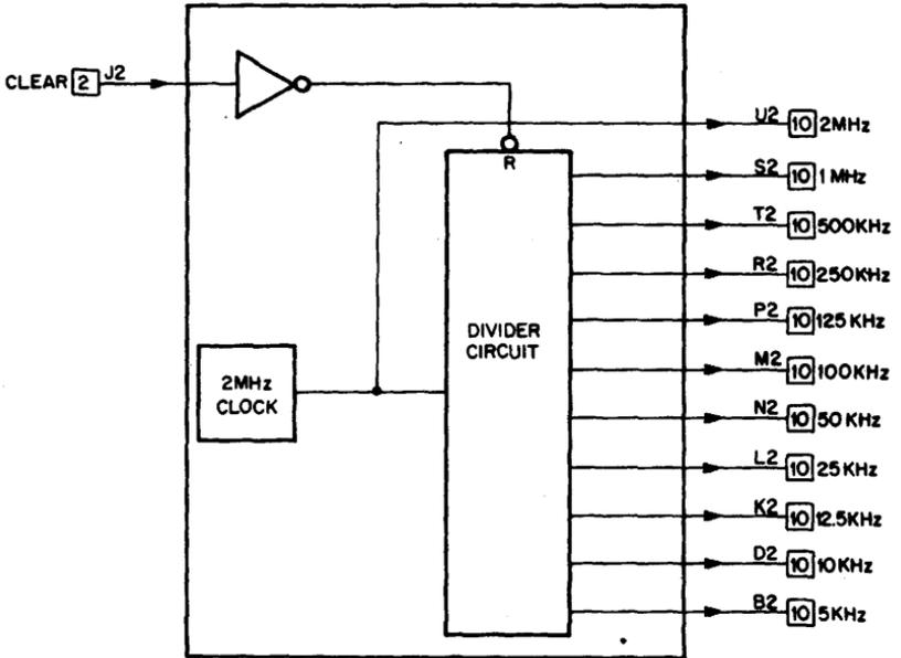
The M404 clock contains a 2 MHz crystal oscillator and frequency dividers.
