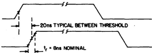
The M502 contains two non-inverting high-speed signal converters which interface standard negative (-3 volts and ground) logic levels or pulses with M and K Series positive logic modules. These converters provide sufficient current drive at a low output impedance for system interconnections by means of terminated 92-ohm coaxial cable.
