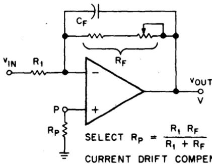
$$\frac{V_{OUT}}{V_{IN}} = -\frac{R_F}{R_1}$$
