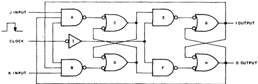
Figure 15. Master-Slave J-K Flip-Flop
