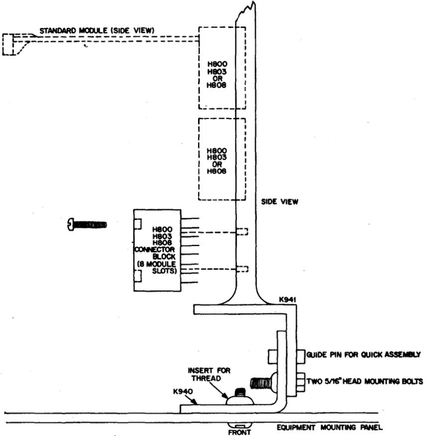
This convenient mounting hardware permits logic connector pin wiring to be done before logic is installed in the enclosure.
