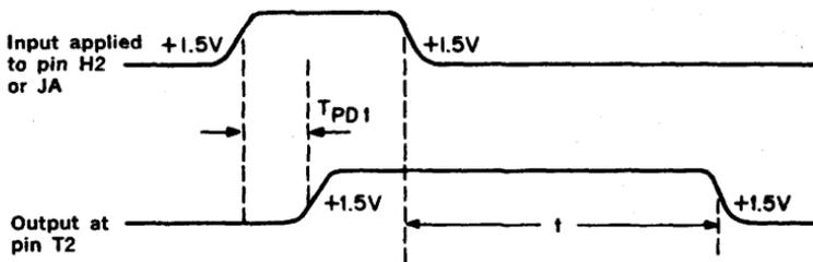
The integration period is measured from the trailing edge of the input pulse to the trailing edge of the output pulse. The approximate integration time may be calculated by the following:
