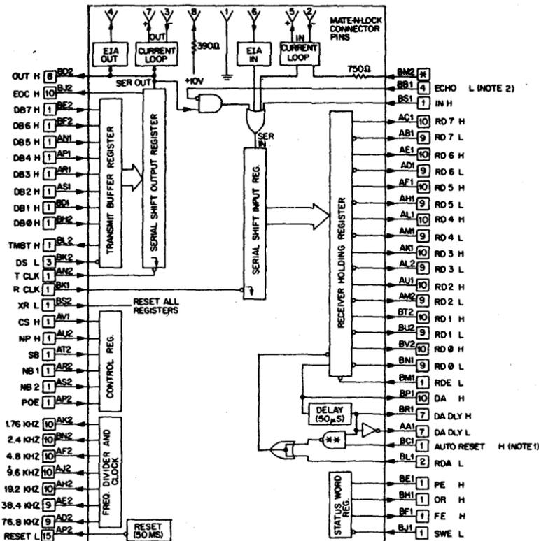
NOTES: \*\*TIED TO -15V WHEN M7390 USED TO DRIVE CURRENT LOOP
