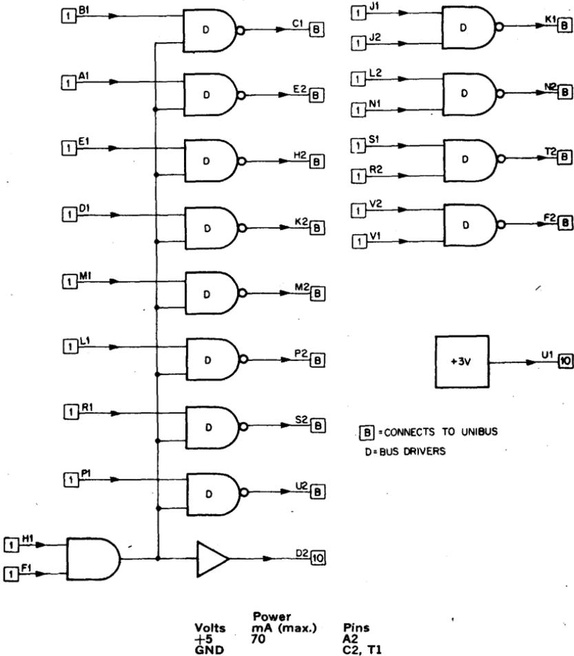
The M783 consists of 12 drivers to be used as an input interface to the UNIBUS of the PDP-11. Pin U1 provides +3 volts as a source of logic HIGH for 10 TTL loads.
