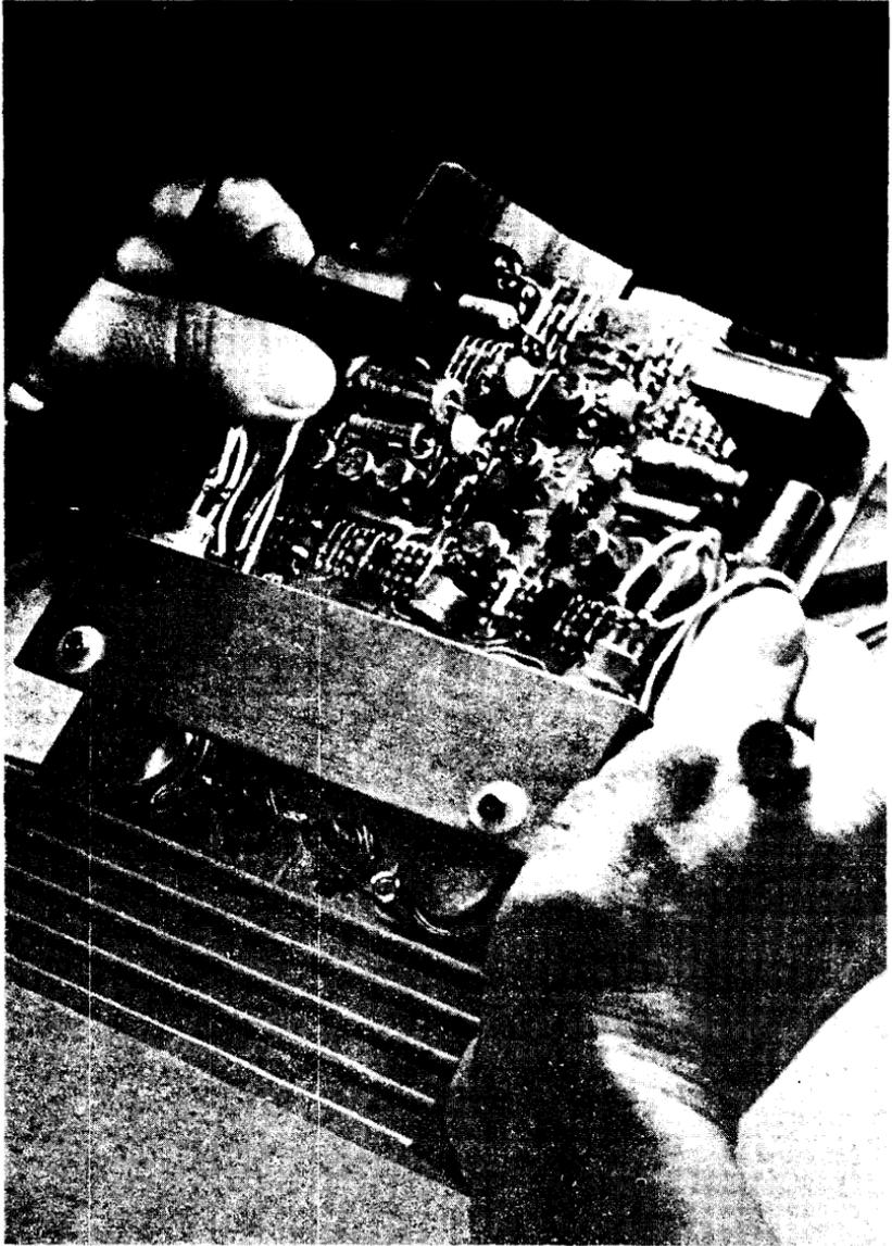
All DEC modules are exhaustively inspected and tested, both visually and electronically. A typical module undergoes a printed circuit board inspection procedure that consists of over 70 individual steps.
