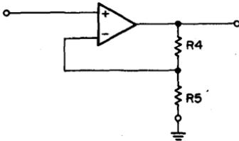
$$\frac{E_O}{E_{IN}} = \frac{R_4 + R_5}{R_5}$$
