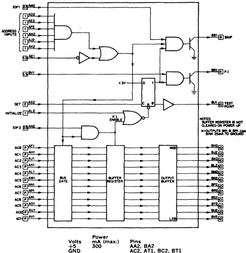
The M737 12-Bit Bus Receiver Interface is completely contained on a double height, single width module.
