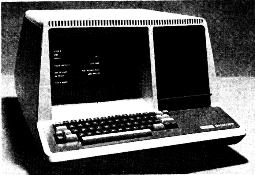
The VT50 DECscope is an alphanumeric video display ideally suited for either quantity usage as remote data terminals in a large timesharing network or as a single station for local I/O applications. The extremely low cost of the VT50 benefits the user by providing a fast video capability at a price comparable to conventional teletypewriters.
