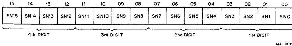
Figure 2-7 Serial Number Register Format
