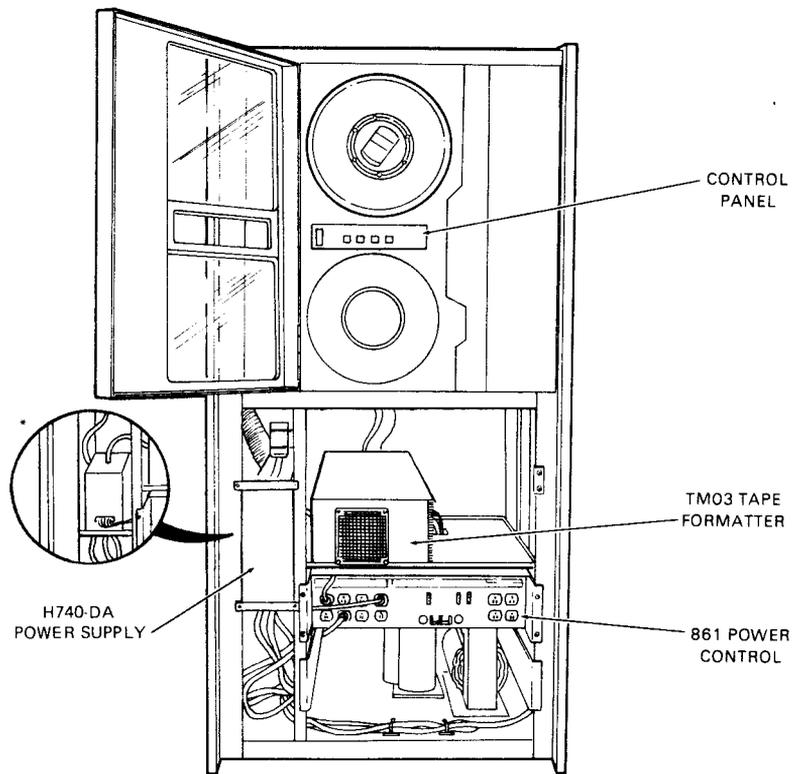
\* NOTE: EARLY TU77/TM03 CONFIGURATIONS HAVE H740-DA MOUNTED IN THE REAR OF THE CABINET
