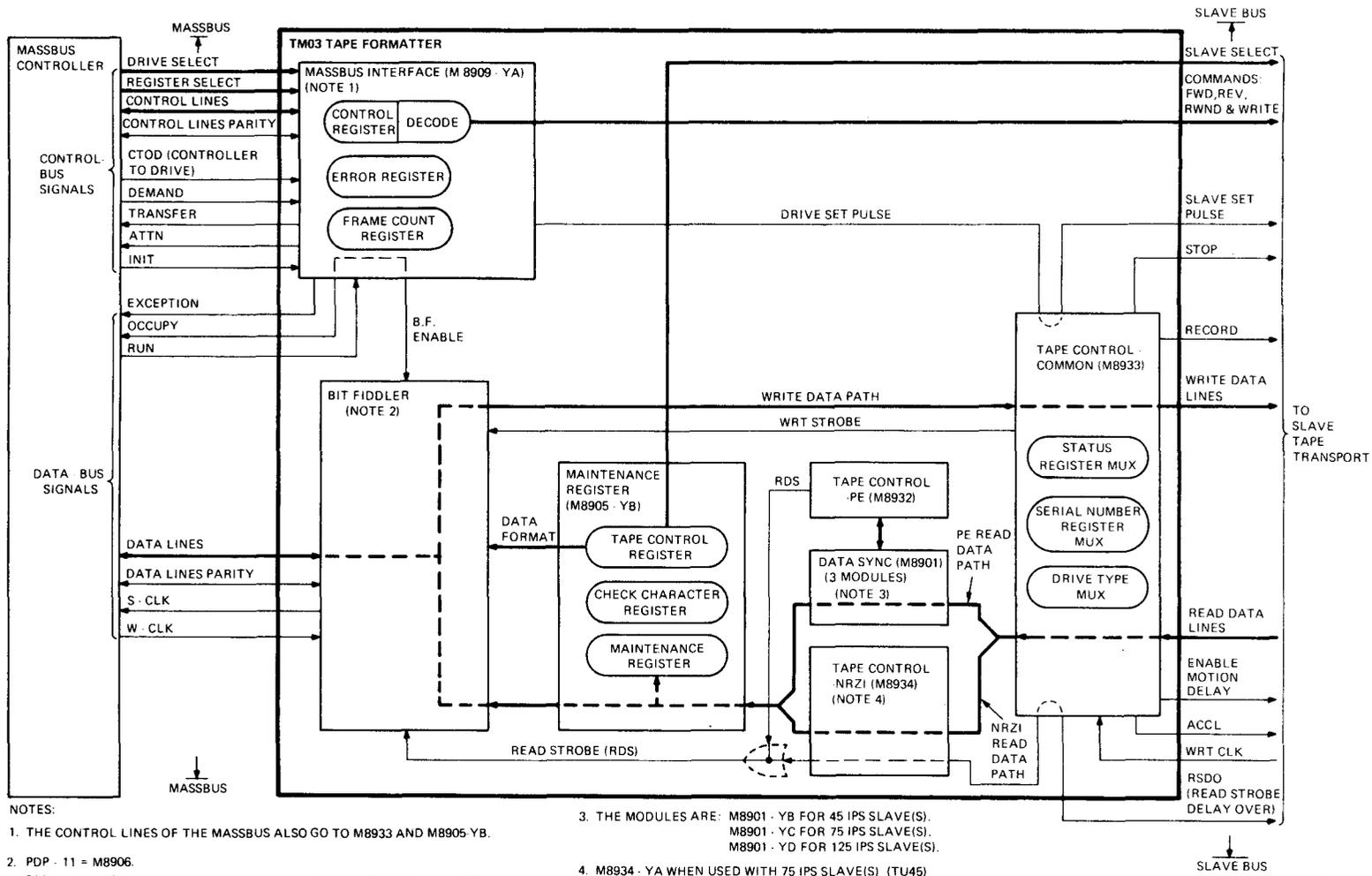
Figure 1-7 TM03 Basic Block Diagram
