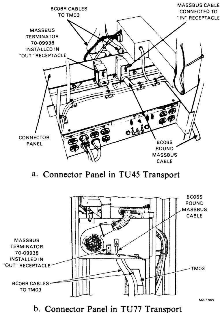
Figure 3-5 External Cabling to Massbus Connector Panel in H9500 Corporate Cabinet
