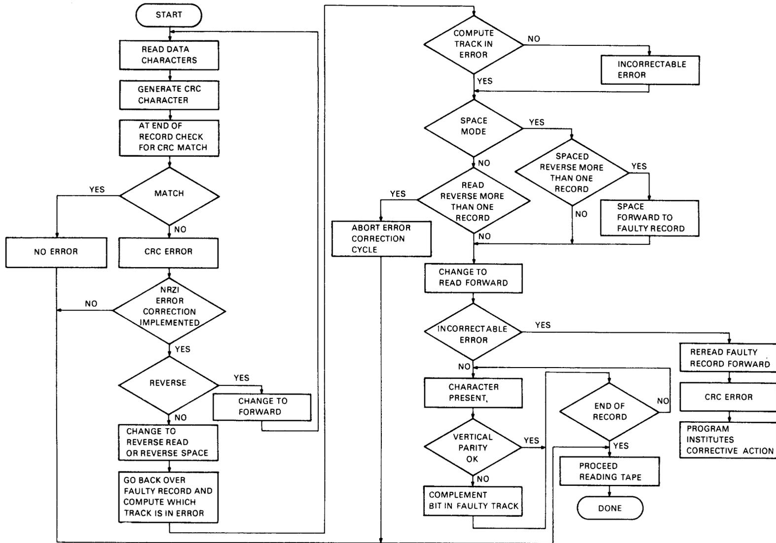
Figure 2-10 NRZI Error Correction Flow Diagram
