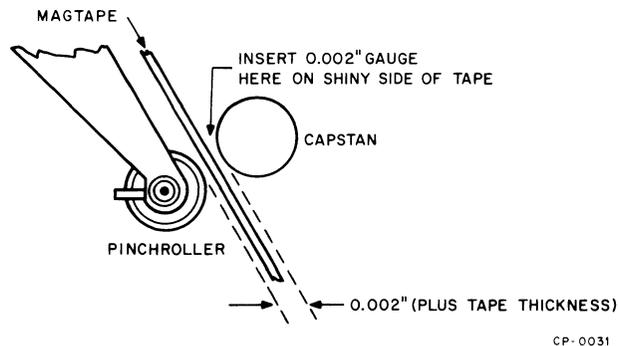
Figure 5-3 Pinchroller – Capstan Clearance
