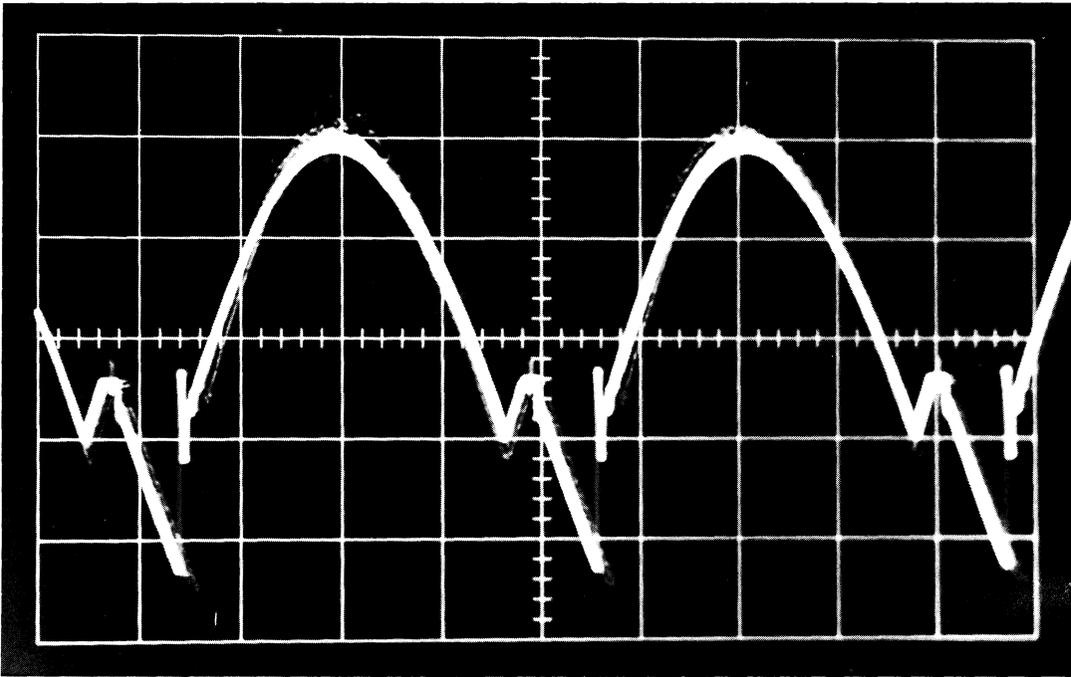
Figure 5-16 REEL SERVO BOARD, Non-Standard 80 Vac Waveform
