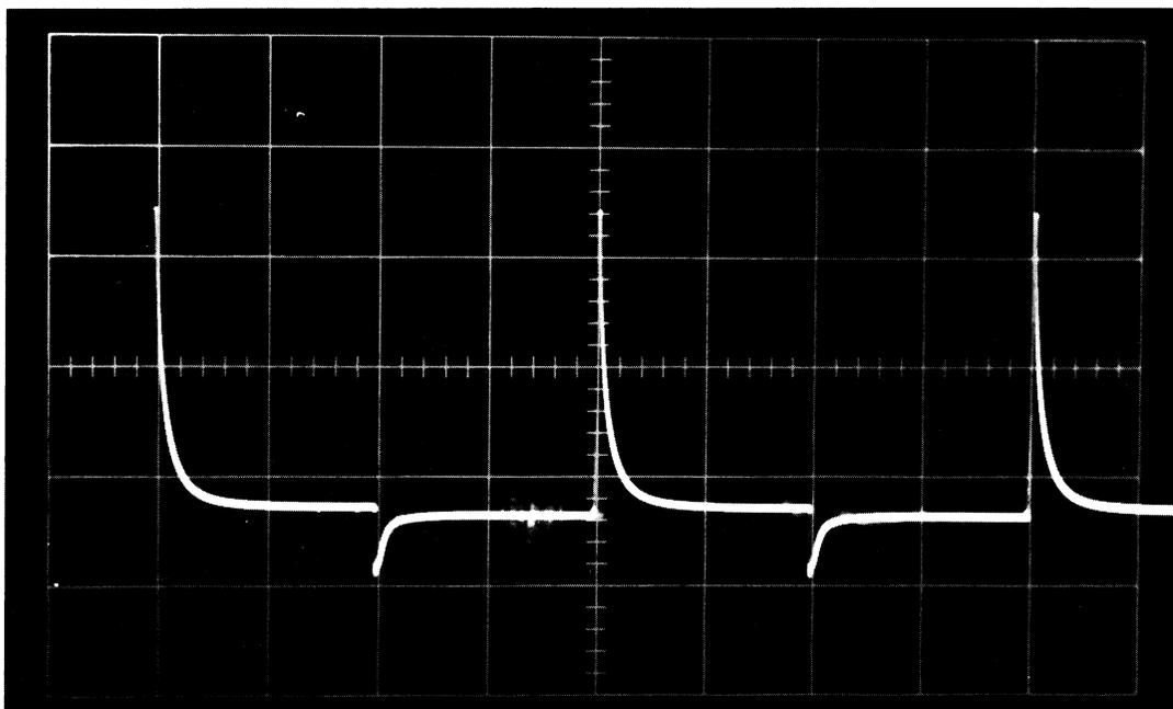
Figure 5-5 Write Driver Output
