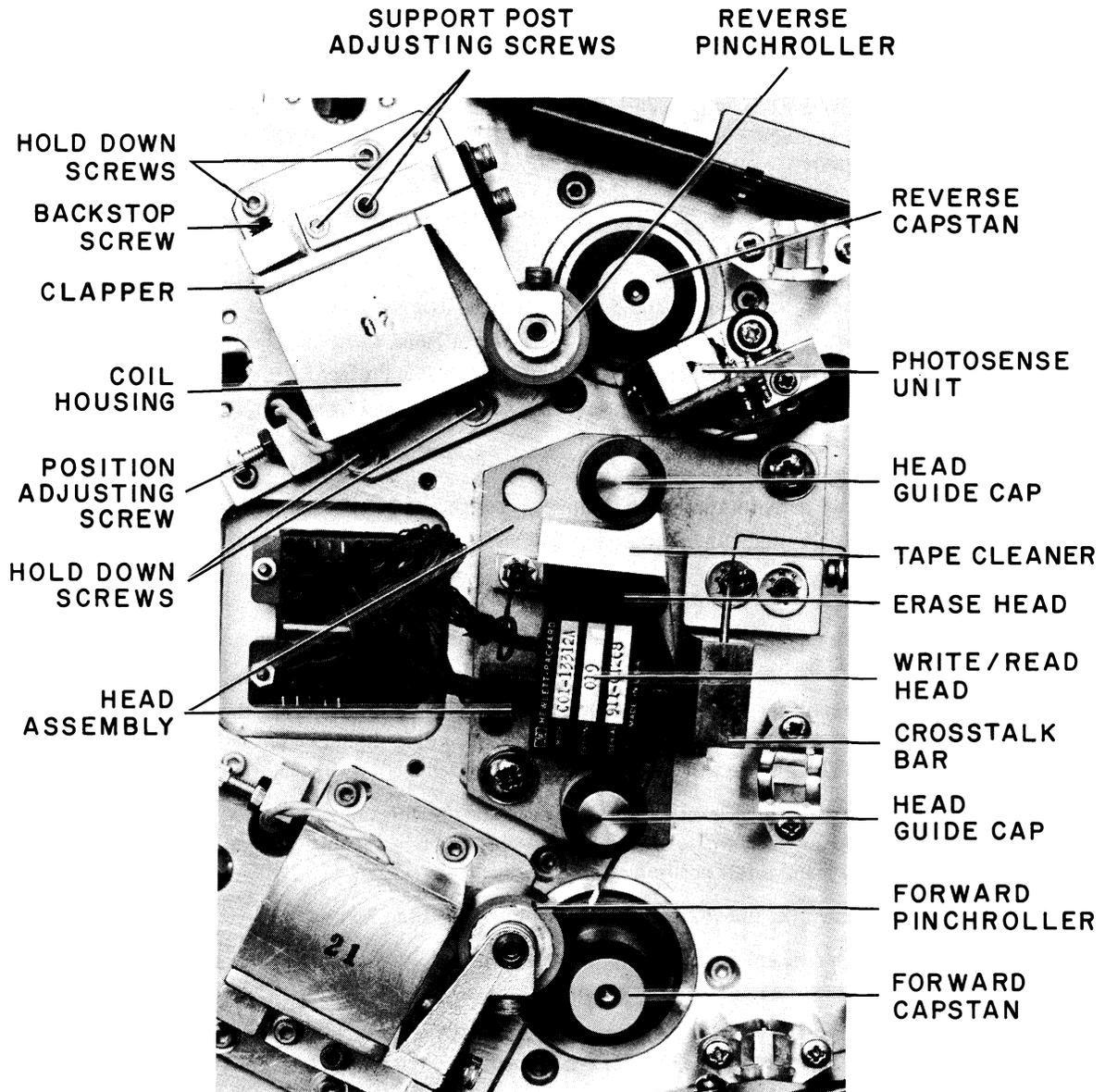
Figure 5-2 Transport Mechanism
