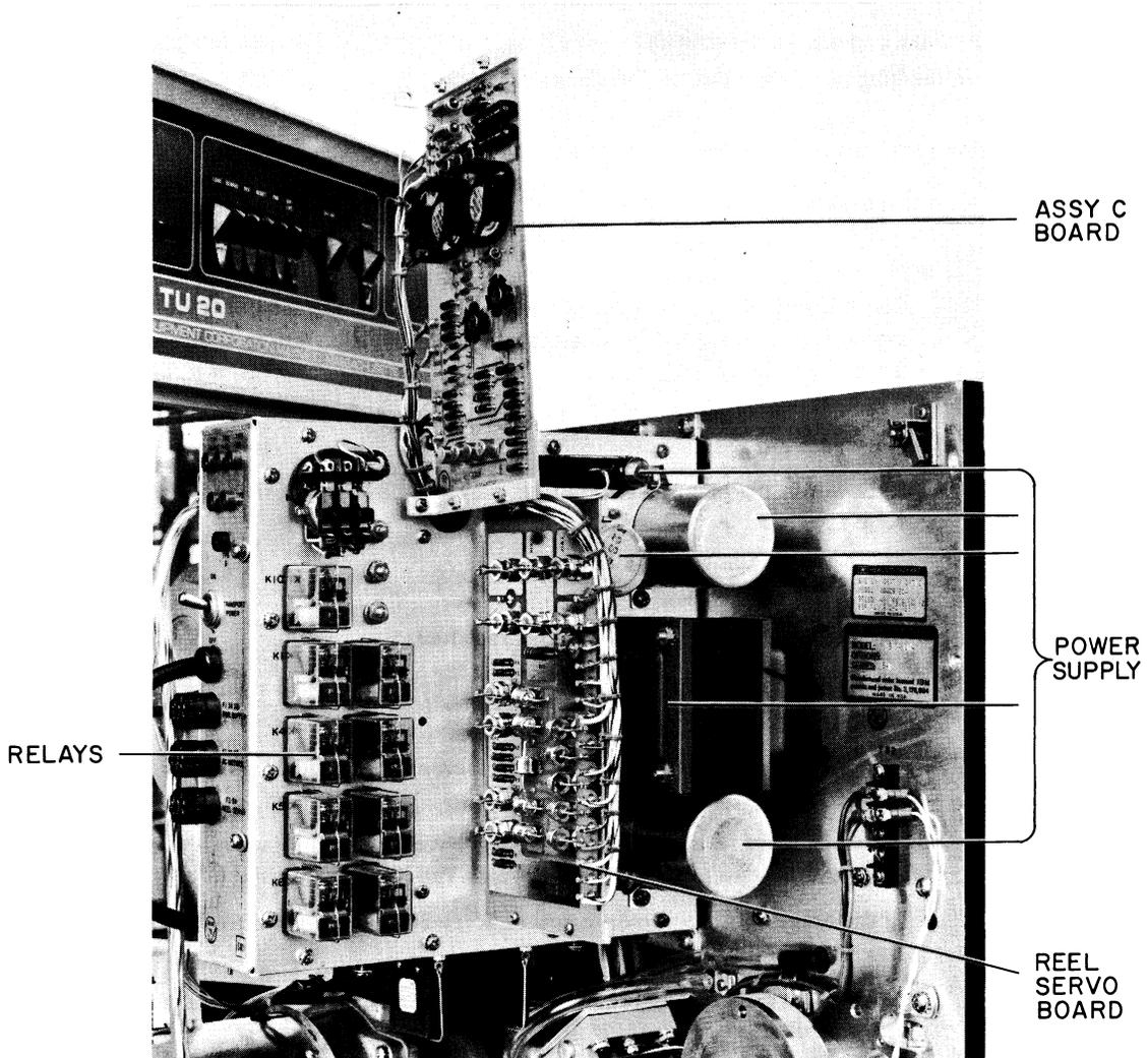
Figure 5-13 REEL SERVO BOARD and ASSY C BOARD
