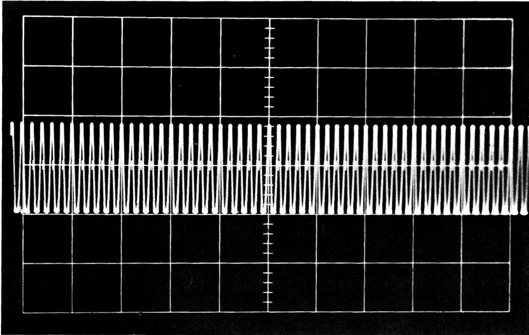
Figure 5-9 Read Amplifier Output
