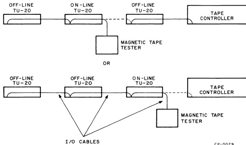
Figure 5-1 Mag Tape Tester Connections
