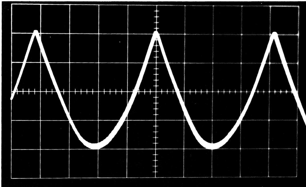
Figure 5-15 REEL SERVO BOARD, Standard 80 Vac Waveform
