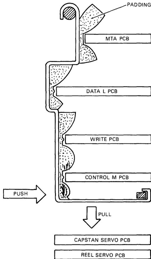
Figure 2-6 PCB Shipping Bracket
