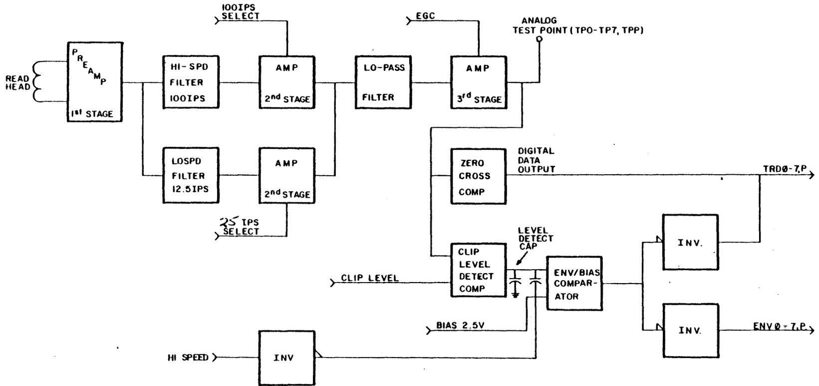
Figure 15 Read Circuits Block Diagram (11/10/75, 11/20/75 (c))
