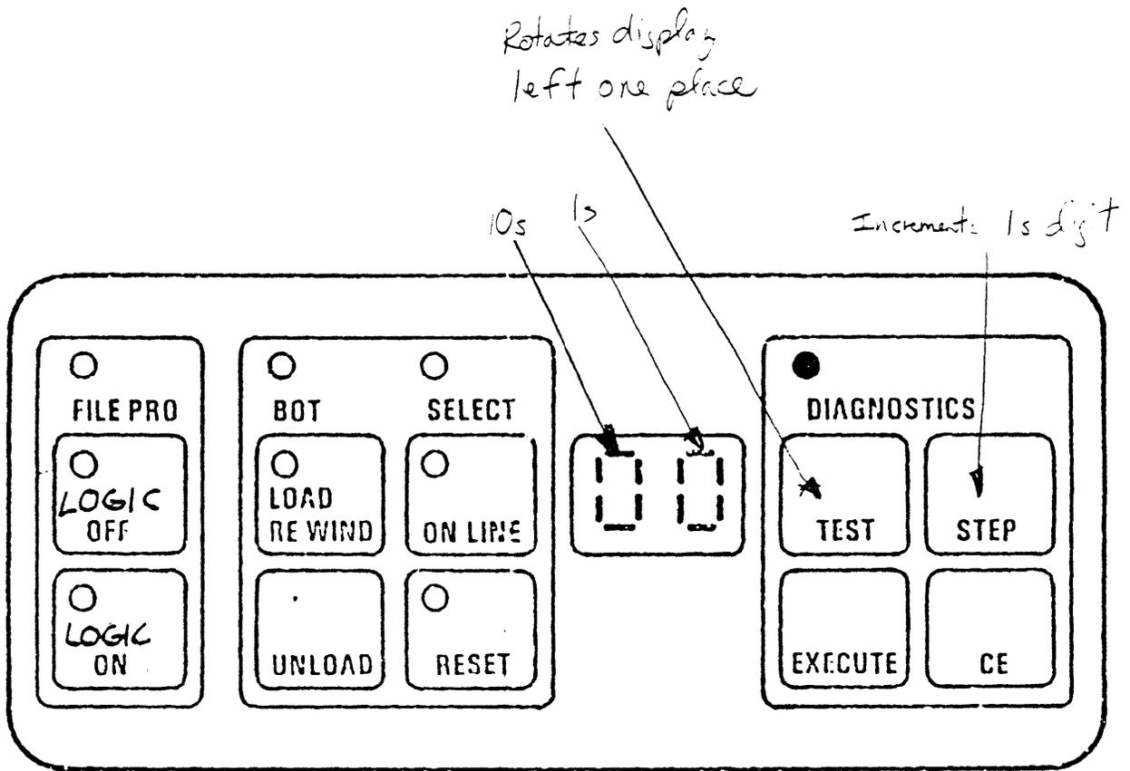
Figure 7 Control Panel With Field Service Diagnostics Loaded
