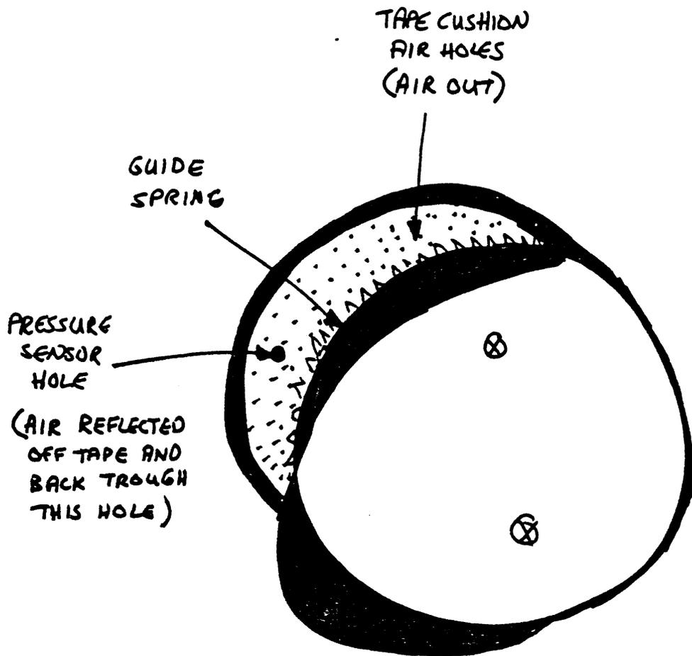
Figure 5 Air Bearing
