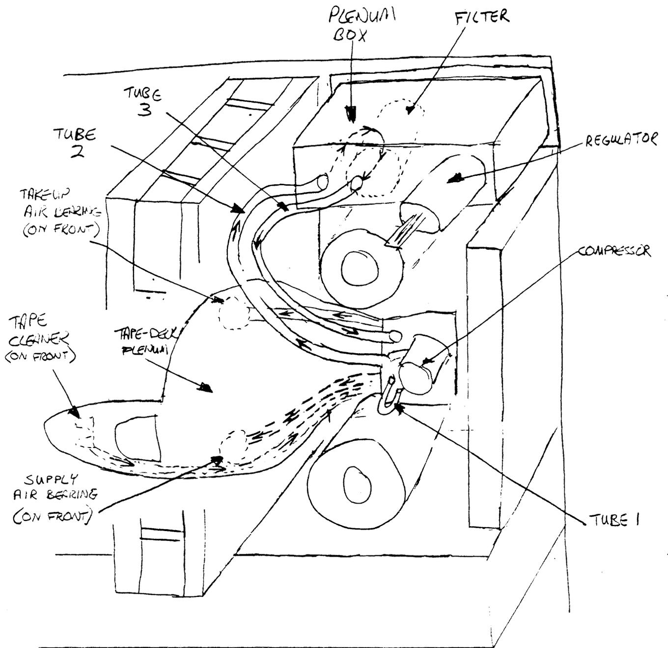
Figure 14 Vacuum/Pressure Air System
