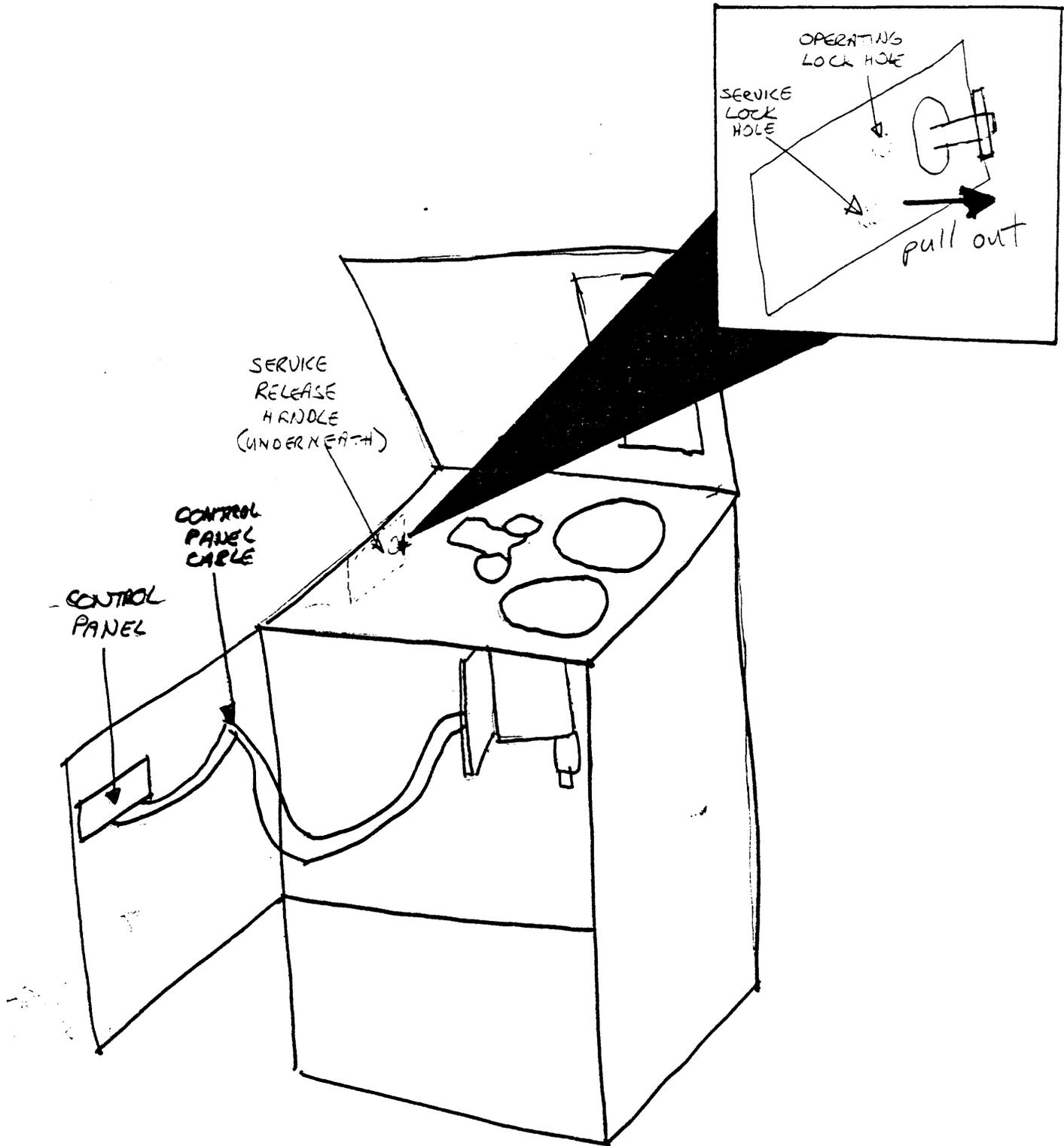
Figure 6 Service Release Handle Access
