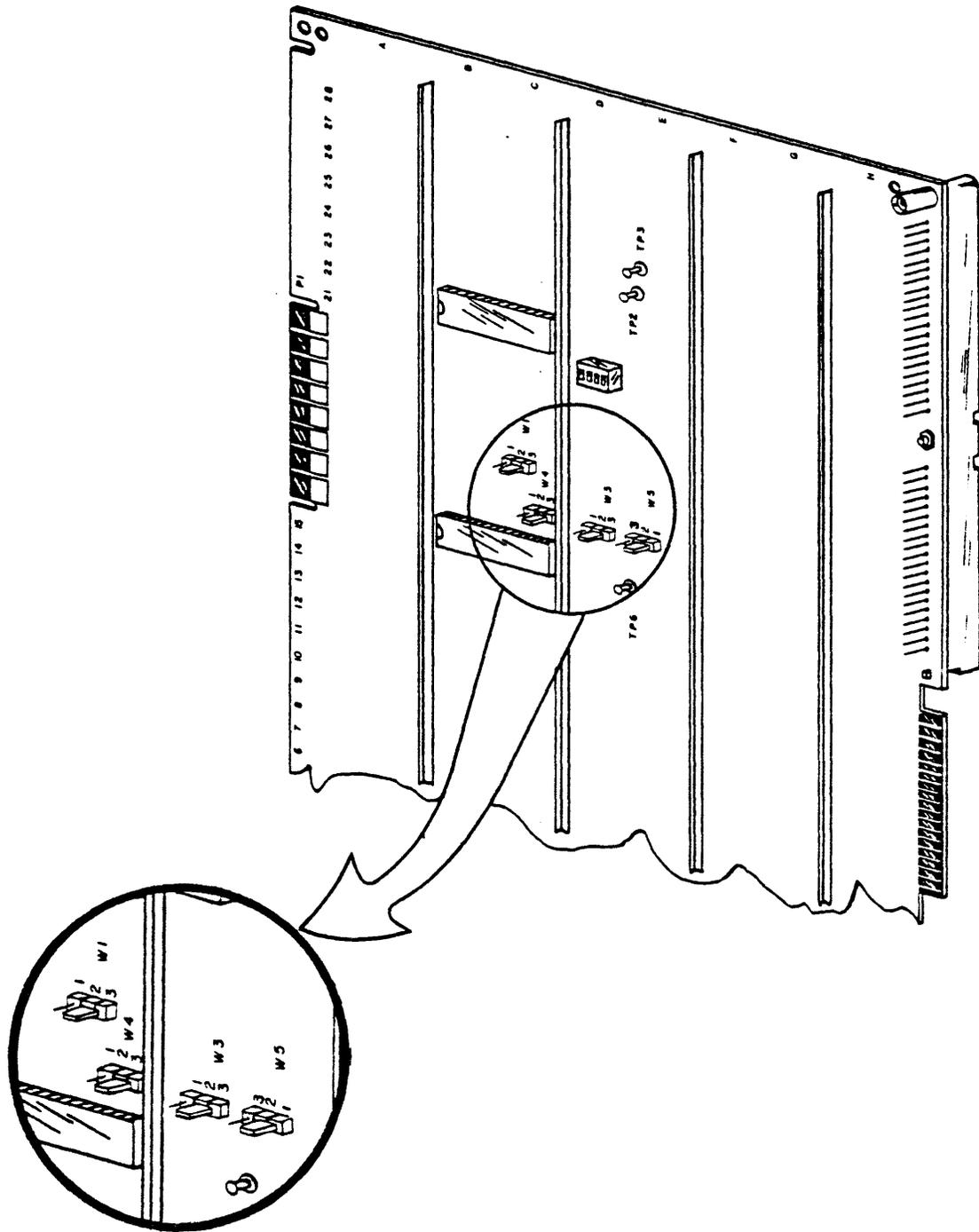
Figure 1-3. Jumper Plug Locations
