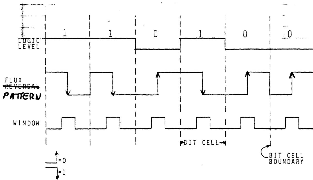
Figure ~~1~~ 1 Phase Encoded (PE) Recording
