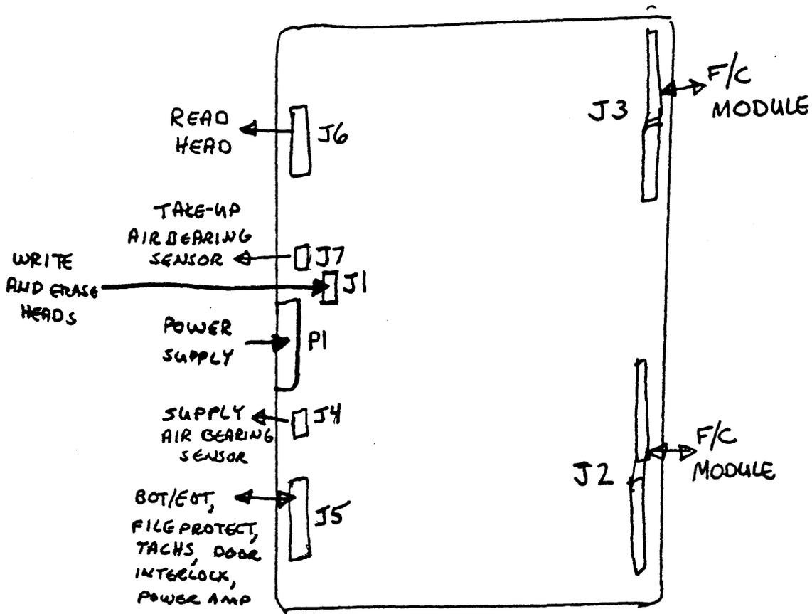
Figure 9 Read/Write/Servo (R/W/S) Module
