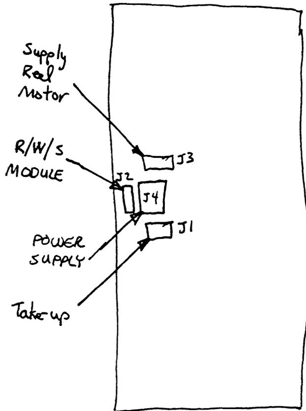
Figure 13 Power Amplifier Module
