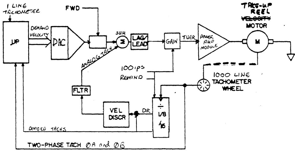
Figure 13 VELOCITY SERVO
