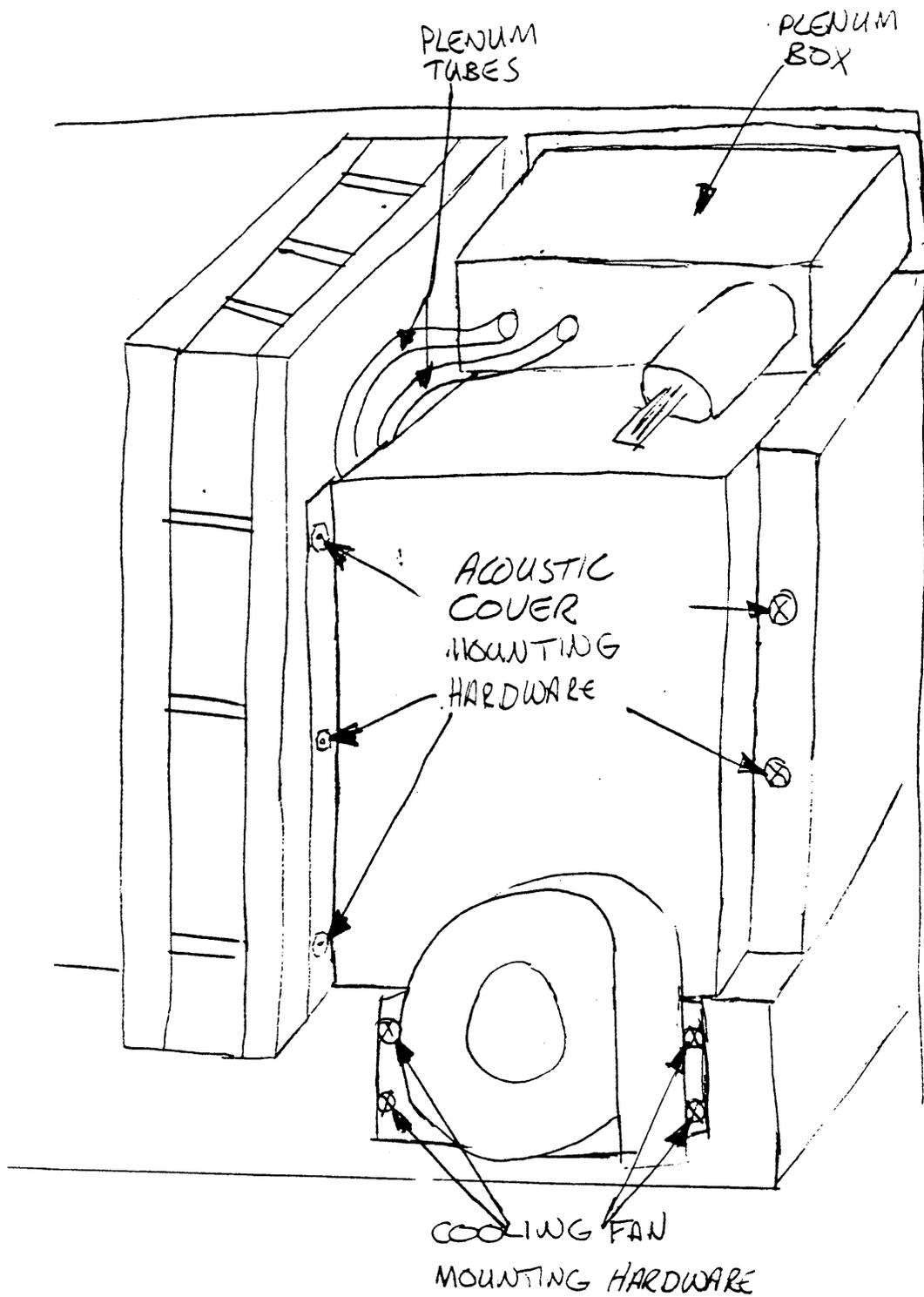
Figure # FCC Shield Removal
