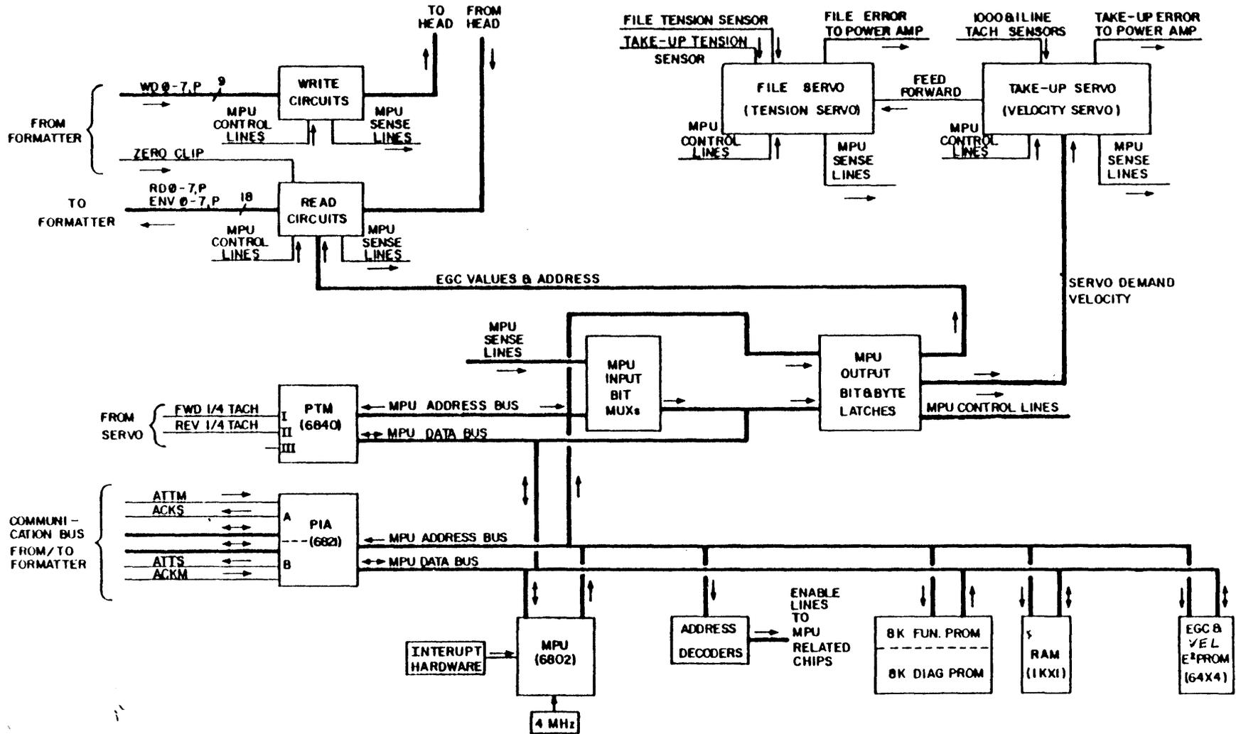
Figure 12 Read/Write/Servo Module Block Diagram
