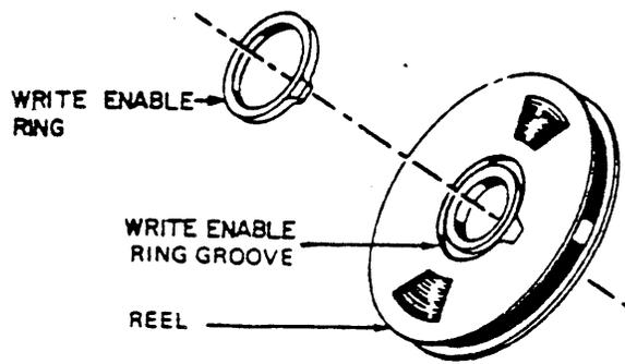
Figure 3 Write Enable Ring
