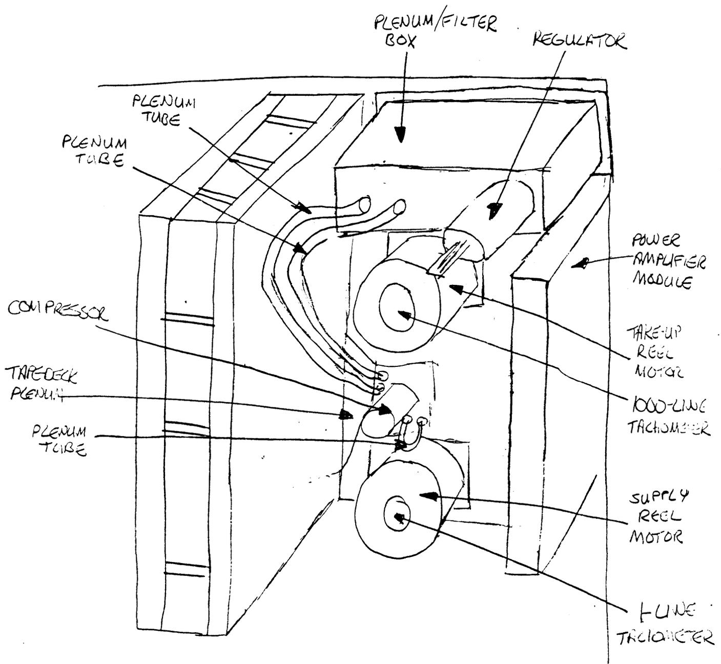
Figure 12 STU Components (Shield Removed)
