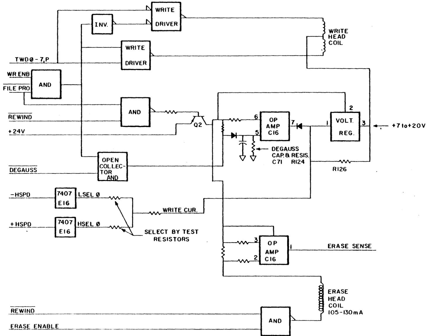
Figure 16 Write/Erase Block Diagram (R104/S. H. 11/20/64)
