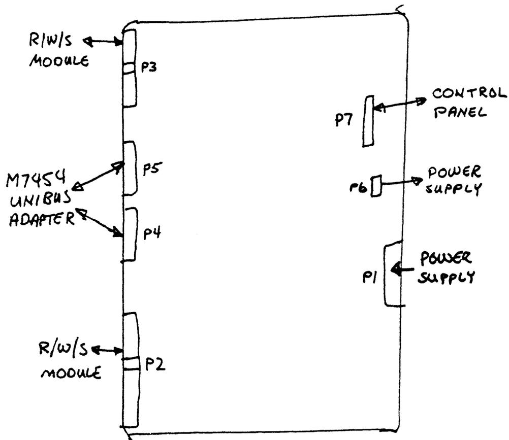
Figure 10 Formatter/Control (F/C) Module
