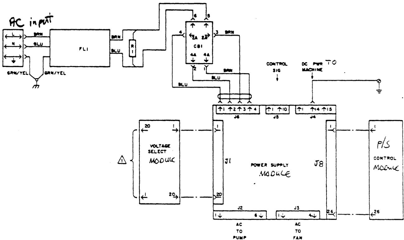
⚠ BOARD FLIPS FOR 120V, 60HZ, OR 220V, 50HZ
