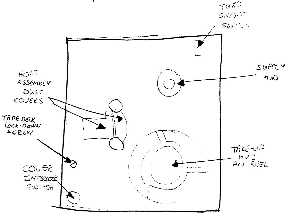
Figure 3 STU Components (Top)
