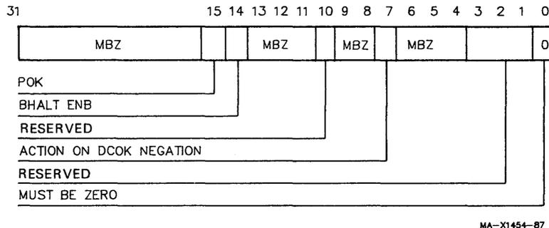
**Figure 3-39 System Configuration Register**
