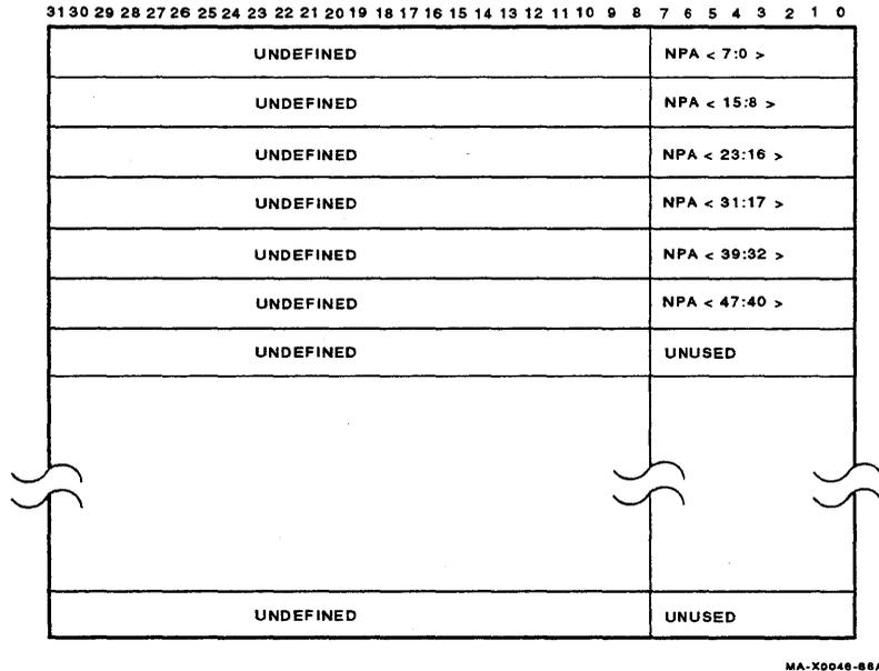
**Figure 3-44 Network Interface Station Address ROM Format**
