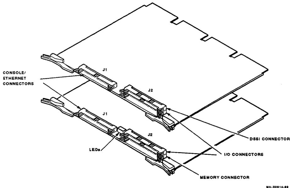
Figure 2-3 KN210 Connector and LED Orientation
