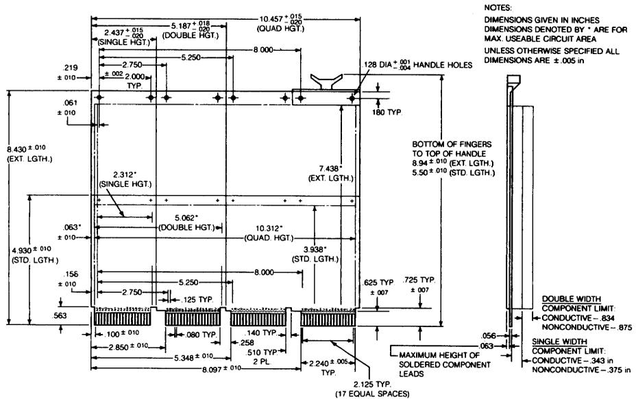
Figure C-20 Typical Q22-bus Module Dimensions
