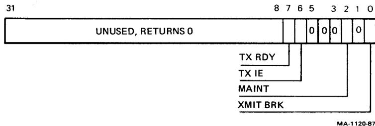
**Figure 3-24 Console Transmitter Control/Status Register**
