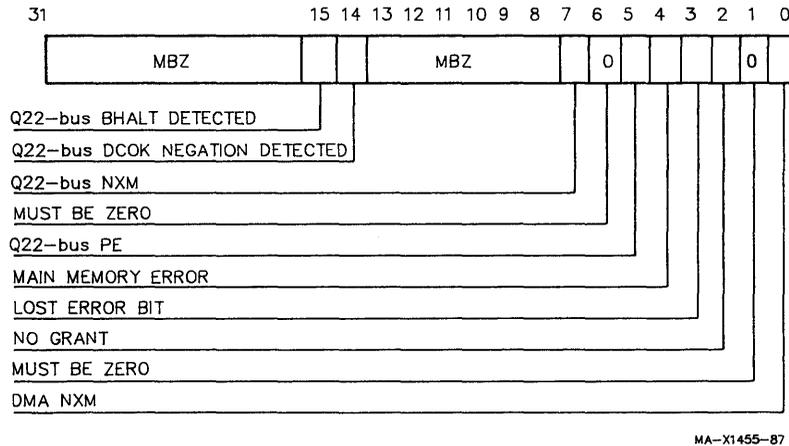
**Figure 3-40 DMA System Error Register**
