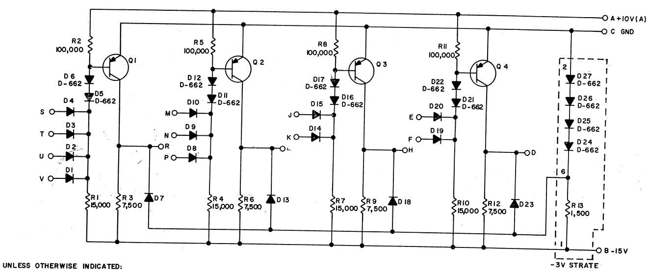
TRANSISTORS ARE DEC 3639B DIODES ARE D-664 RESISTORS ARE 1/4 W, 5%
