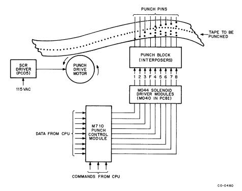
Figure 1-2 Punch Functional Block Diagram
