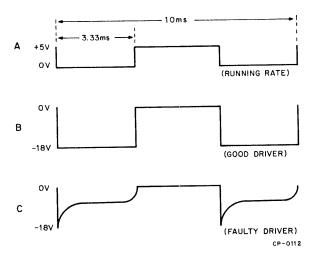
Figure 5-7 M040 Input and Output Waveforms
