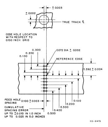
Figure 5-10 Specifications for 1-In. Paper Tape
