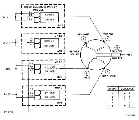
Figure 4-1 Tape Feed Operation
