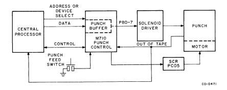
Figure 4-2 Simplified Block Diagram, Punch Operation
