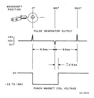
Figure 5-12 Electrical Parameters
