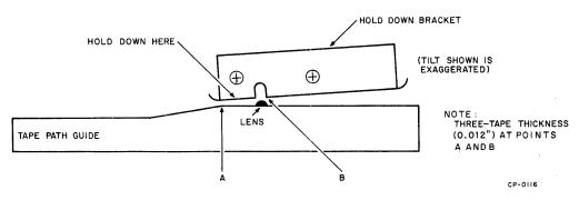
Figure 5-4 Tape Hold-Down Bracket
