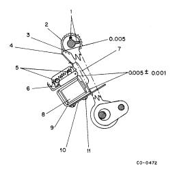
Figure 5-14 Forward Index Magnet Armature
