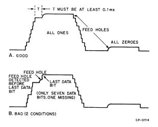
Figure 5-9 Summation Waveform, G918 Test Point
