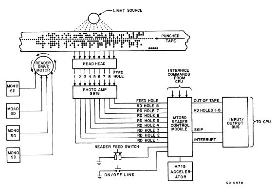
Figure 1-1 Reader Functional Block Diagram
