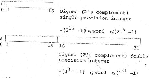
The address of a double precision quantity is the address of the high-order word. This address must be even (i.e.  $EFA_{15} = 0$ ).
