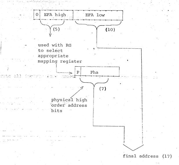
A maximum of 64<sub>10</sub> protection/mapping registers, each one byte long, may be accommodated. One map (32 mapping registers) is provided for priority level 0 (user mode) which will be referred to as the user map. Another map is provided for the other seven levels (monitor mode) which will be referred to as the monitor map since the monitor program normally runs at priority level 1 and the monitor controlled IO routines run at levels 2-7.
