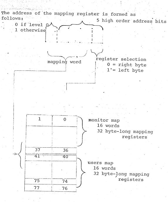
If the P bit is set and PHA is nonzero, then the specified memory page is taken to be read only and no user mode program may write into that page. An instruction executed in user mode that attempts to write into a read only page causes a read only violation which: (a) raises priority to level 1, (b) sets bit 5 of the PSW, and (c) initiates a trap sequence (see section 2.5.1).
