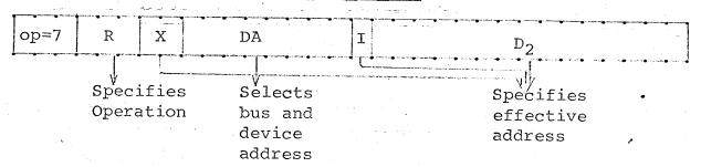
The IOD instruction is used to change the state of the IO system. The DA field is used to decode specific functions, unused DA codes lead to no operation.
