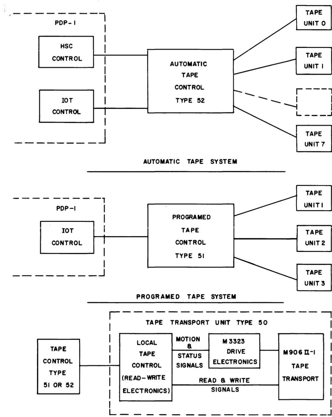
Figure 2-1 Tape System Configuration Diagram
