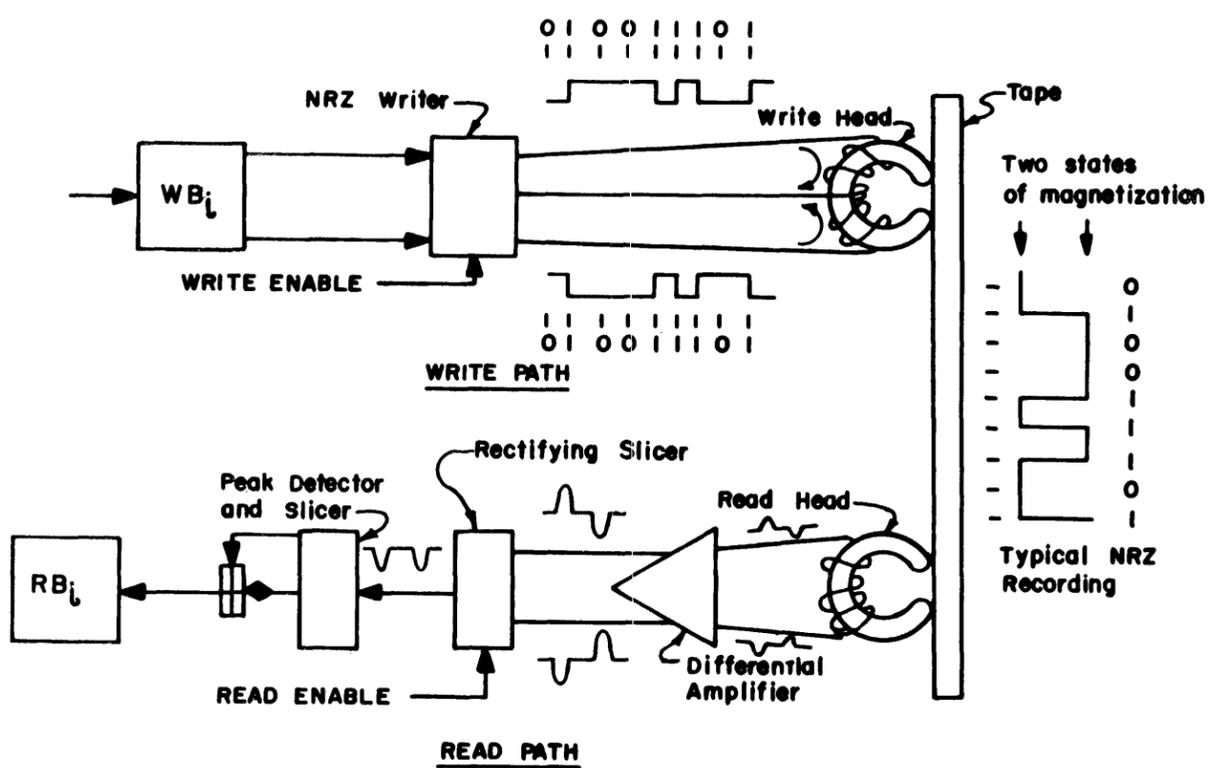
Figure 4-3 Tape Write and Read Signal Flow
