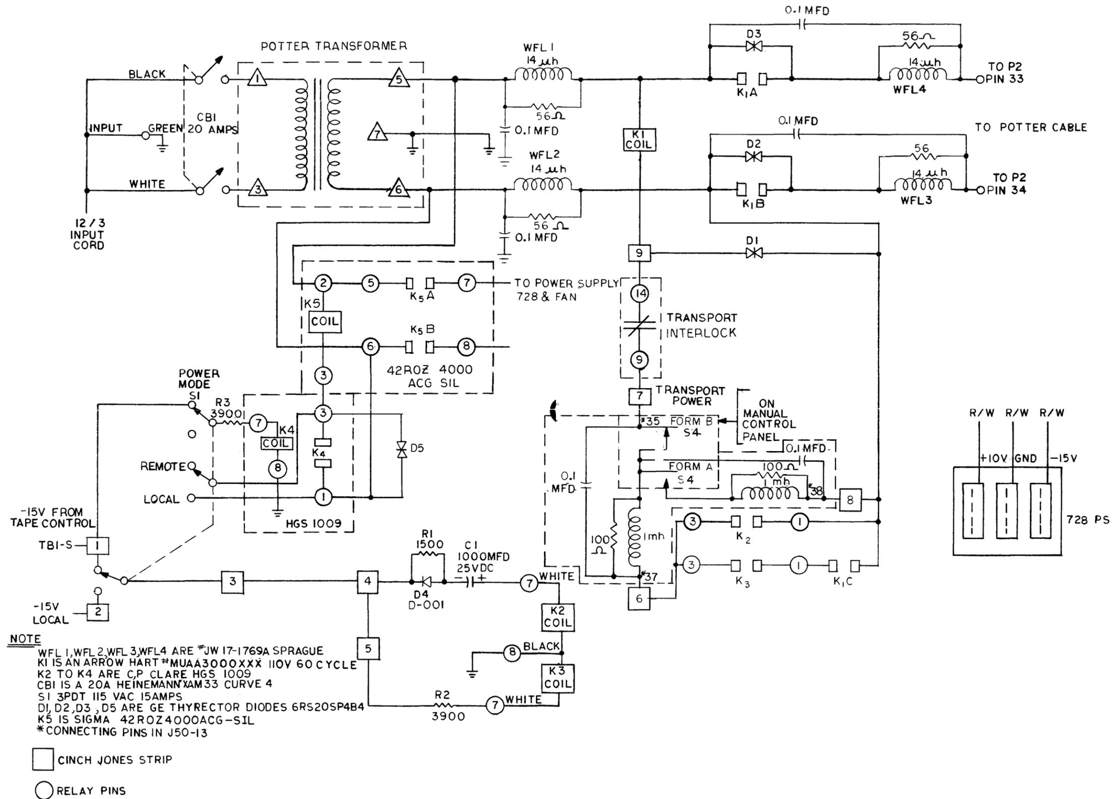
Figure 7-3 Power Control Wiring for Tape Unit 50
