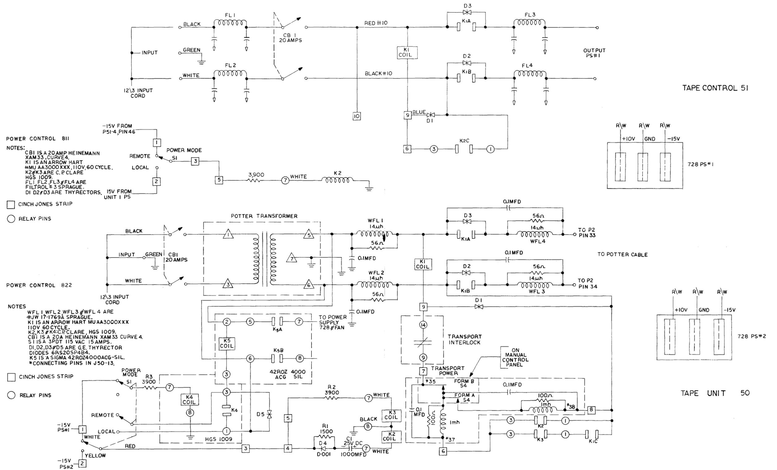
Figure 7-1 Power Control Wiring for Types 50 and 51 Combination
