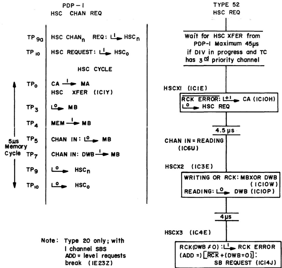
Figure 6-6 Flow Chart: High Speed Channel Access
