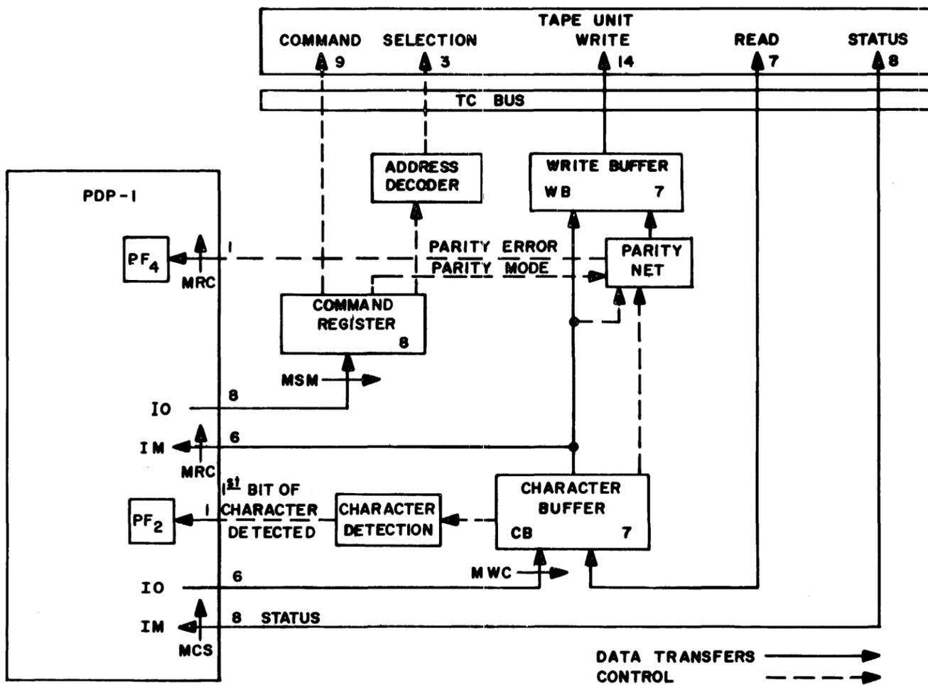
Figure 4-7 Programmed Tape Control 51 Block Diagram
