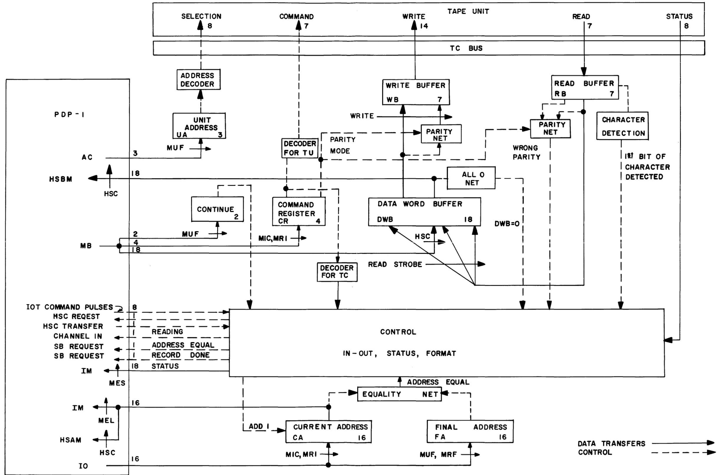
Figure 4-4 Automatic Tape Control 52 Block Diagram
