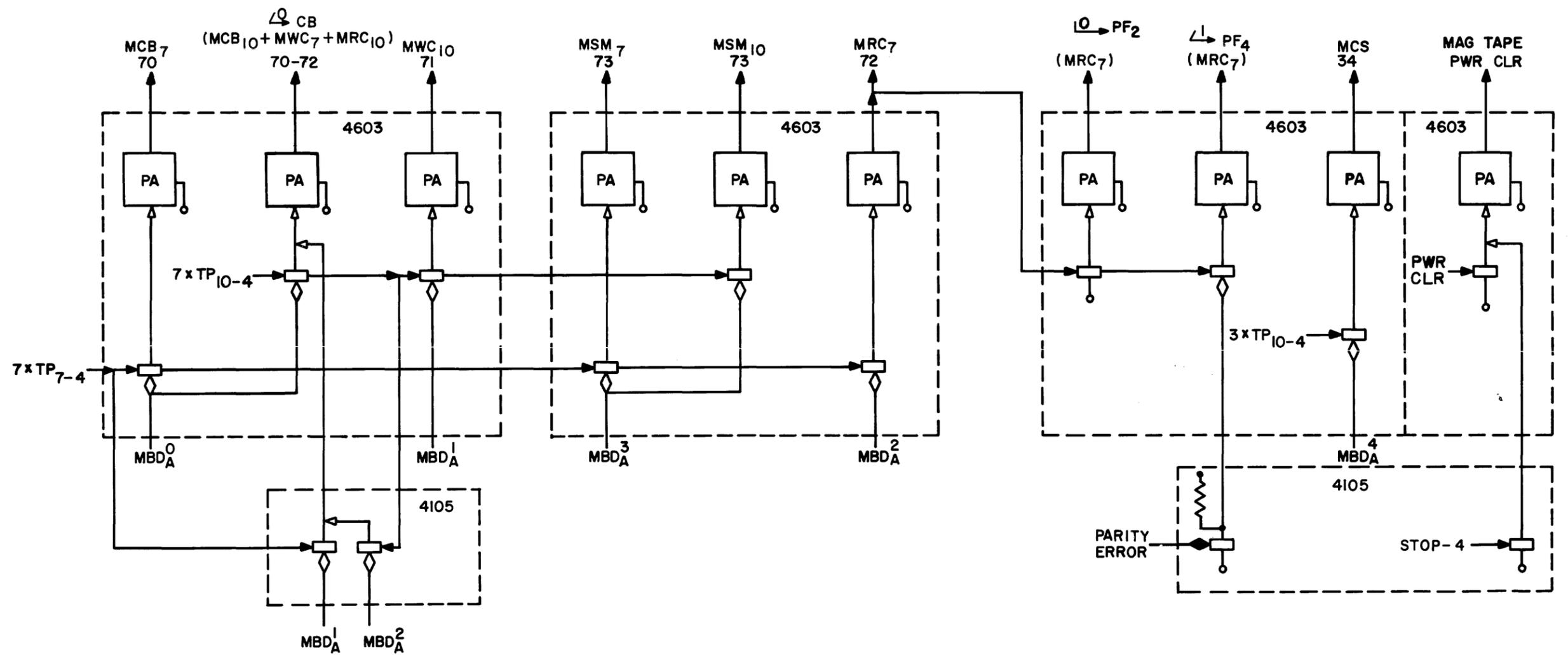
Figure 6-8 IOT Control for Type 51 Tape System
