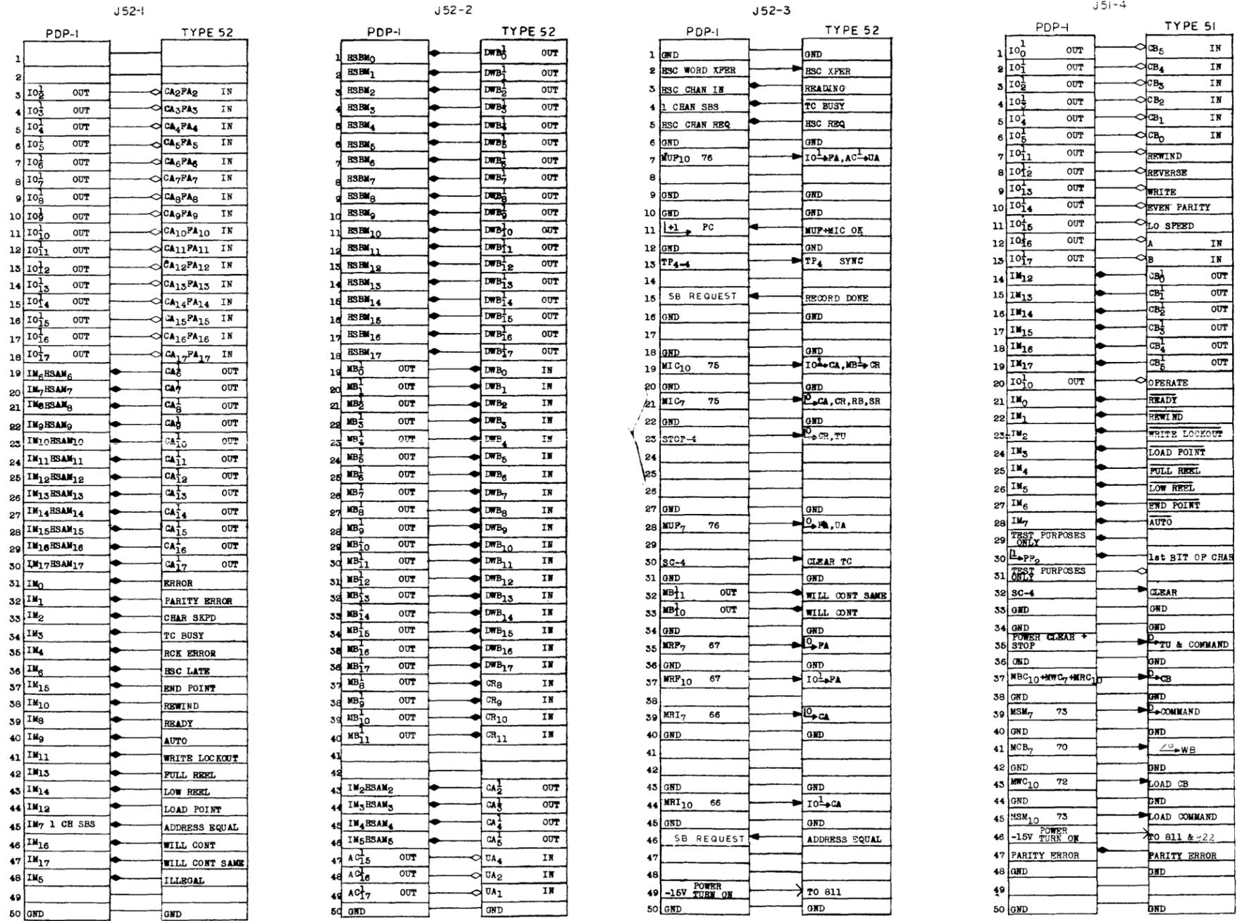
Figure 6-9 Signal Connections: PDP-1 to Magnetic Tape System
