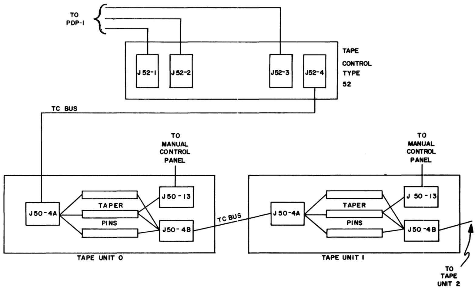
Figure 3-2 Type 52 System Bus Connections
