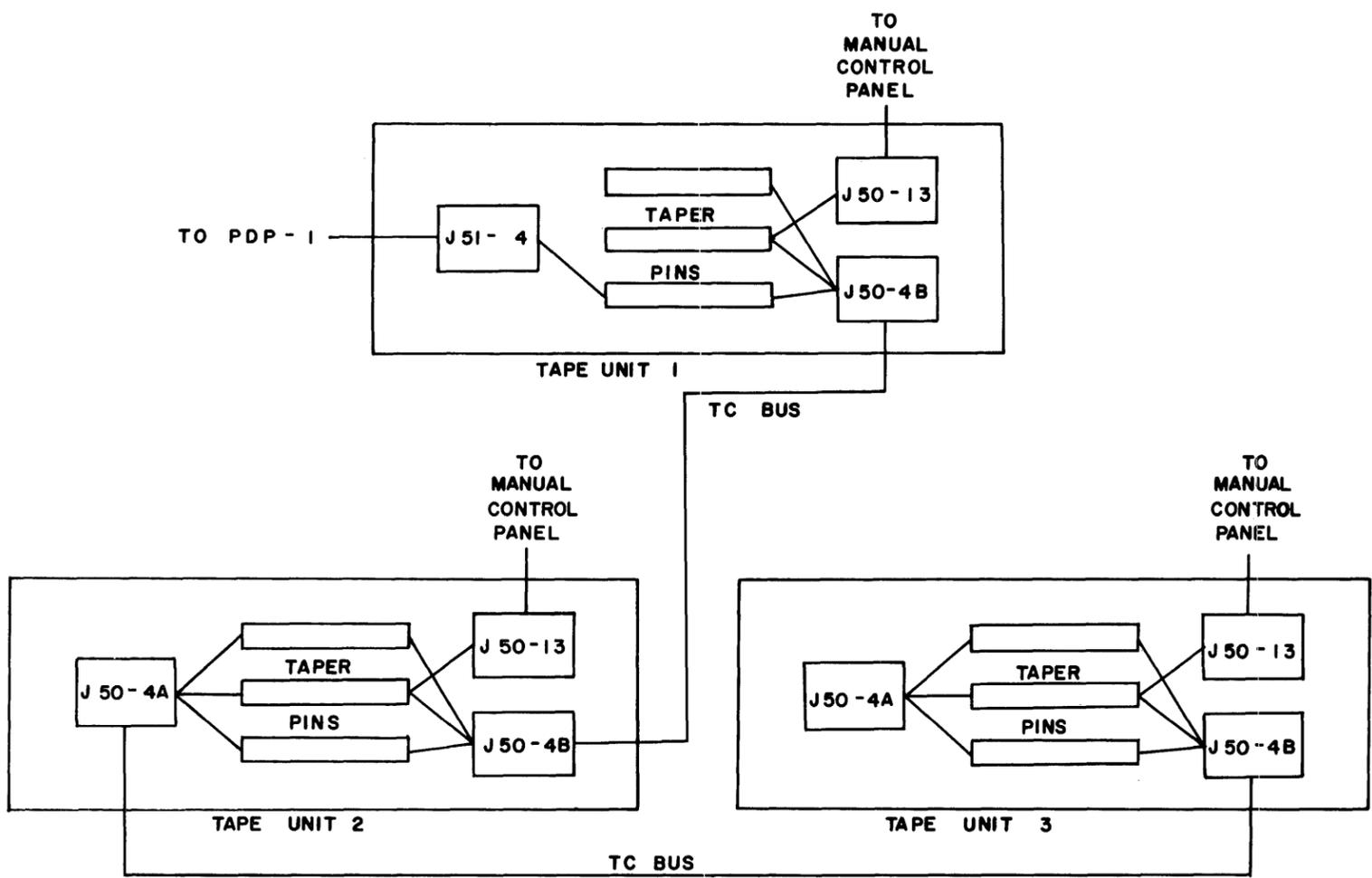
Figure 3-3 Type 51 System Bus Connections
