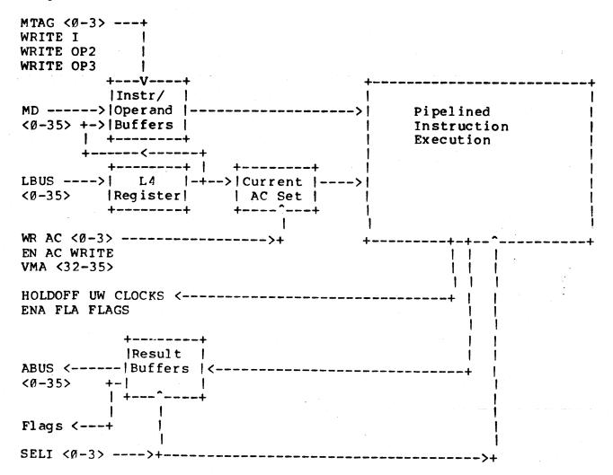
The FPA receives Operand and AC data on MD or LBUS. The data is written into buffers maintained in the FPA. Instruction, OP2, and the AC set are redundant with other buffers in the IBOX and
