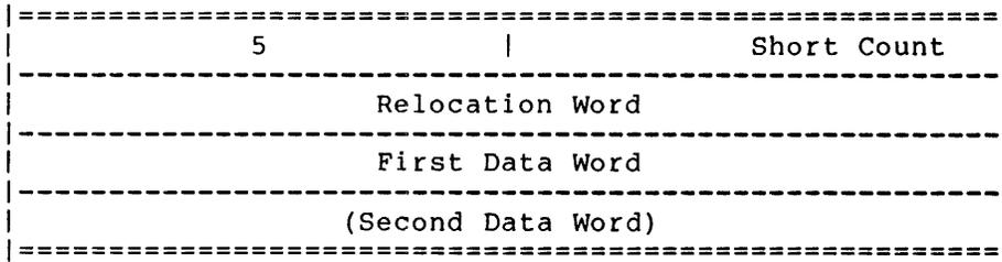
Block Type 5 ends a program module. A Block Type 6 must be encountered earlier in the module than the Type 5 block.
