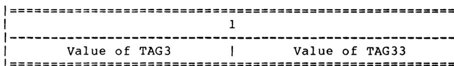
Suppose we load MOD0 first. The .LNKEND statement for MOD0 generates a negative chain number. LINK sees the negative chain number (-1) and recognizes this as the result of a .LNKEND statement for chain number 1. LINK remembers the store address (value of TAG0) as the base of the chain.
