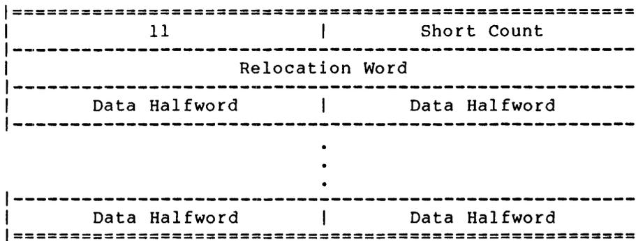
Block Type 11 defines Polish fixups for operations on relocatable values or external symbols. Only one store operator code can appear in a Block Type 11; this store operator code can be either a symbol fixup code or a chained fixup code. The store operator code appears at the end of the block.
