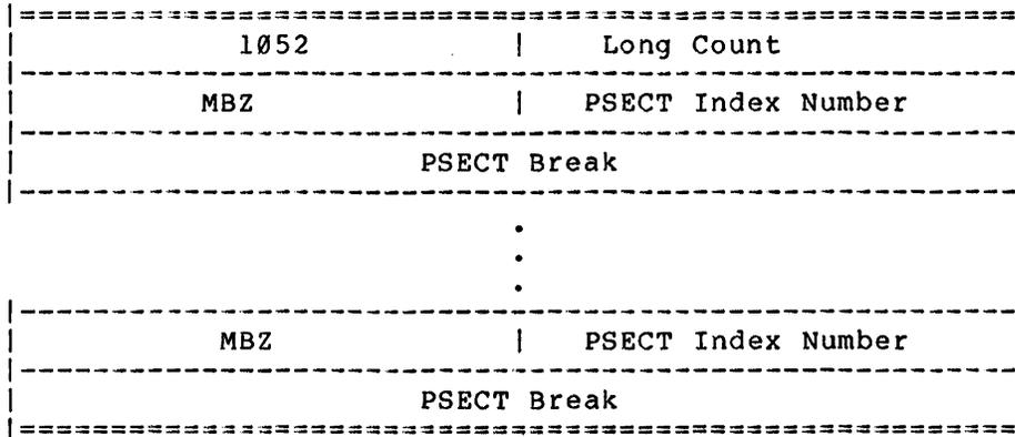
Block Type 1052 allocates additional space for a given PSECT. This space is located between the last address in the PSECT containing data and the address given by the PSECT break. A block of Type 1052 can contain more than one pair of PSECT indexes and breaks.
