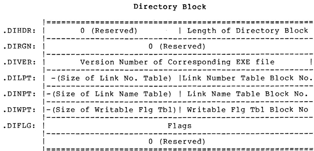
In the fourth word above, the size of the Link Number Table (in words) is half the number of links (rounded upward); the Link Number Table Block No. is the number of the 128-word disk block containing the Link Number Table. (There are four disk blocks per disk page.)
