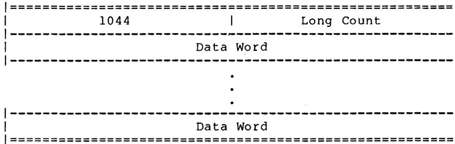
Block Type 1044 contains a debugging symbol table for ALGDDT, the ALGOL debugging program.
