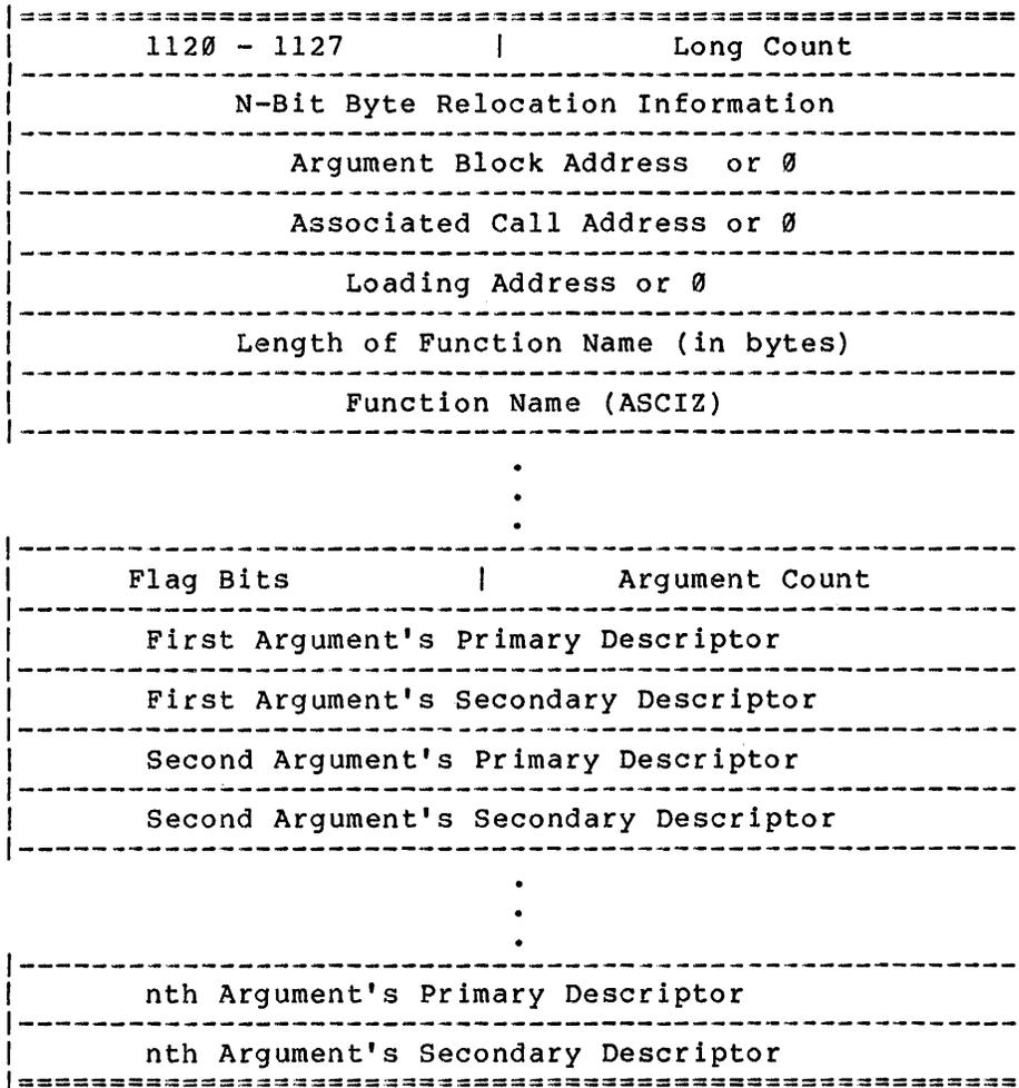
A block of this type is generated for the argument list to each subroutine call. The subroutine entry point also specifies one block with this format, though for the callee the argument block address is zero. If a descriptor block is associated with an argument list it must always follow the loading of the argument list.
