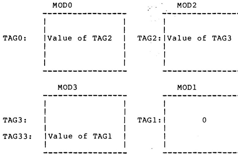
Note that the order of loading for modules with .LINK statements is critical. (A module containing a .LNKEND statement can be loaded any time; its treatment is not affected by the order of loading.)
