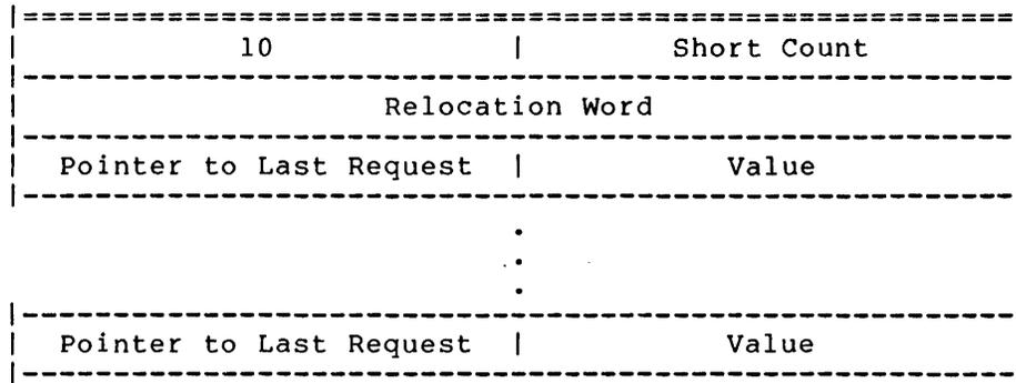
Block Type 10 is generated by one-pass compilers to resolve requests caused by forward references to internal symbols. The MACRO assembler also generates Type 10 blocks to resolve requests for labels defined in literals; a separate chain is required for each PSECT in a PSECTed program.
