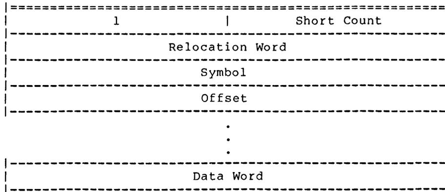
In this alternate format, the first four bits of the first data word (Symbol) are 1100 (binary), and the word is assumed to be a Radix-50 symbol of type 60. The load address is calculated by adding the value of the global symbol to the offset given in the following word. The third and following data words are loaded beginning at the resulting address. The global symbol must be defined when the Type 1 Block is found.
