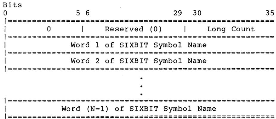
The first six bits of a long symbol are always 0. This distinguishes a long symbol name from a single word symbol name. N is the length of the symbol name including the header word. The remaining words contain the symbol name in SIXBIT, six characters to a word, left justified.
