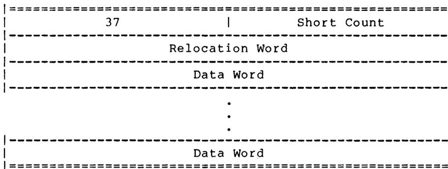
Block Type 37 contains a debugging symbol table for COBDDT, the COBOL debugging program. If local symbols are being loaded, the table is loaded.
