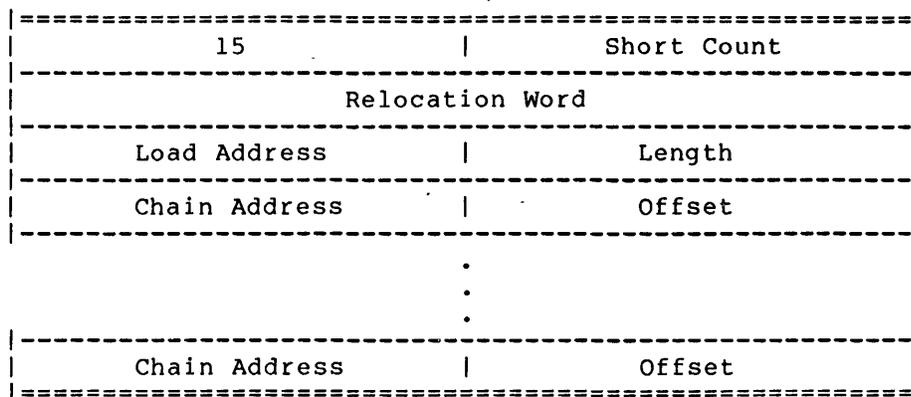
Block Type 15 is used to build the special ALGOL OWN block.
