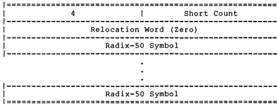
Block Type 4 lists the entry name symbols for a program module. If a Type 4 block appears in a module, it must be the first block in the module. A library file contains a Type 4 block for each of its modules.
