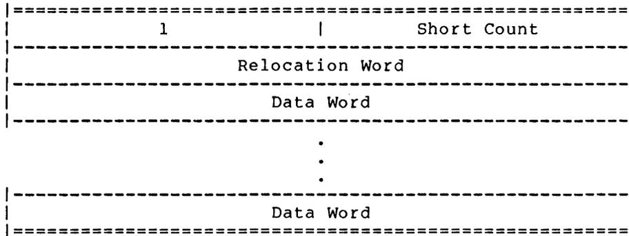
Block Type 1 contains data and code. The first data word gives the address at which the data is to be loaded. This address can be relocatable or absolute, depending on the value of bit 1 of the relocation word. The remaining data words are loaded beginning at that address.
