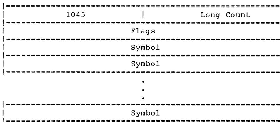
Block type 1045 declares as writable either the link containing the current module or the links containing the definitions of the specified symbols or both. This block type must follow any common block declarations (Types 20 or 6) in a module.
