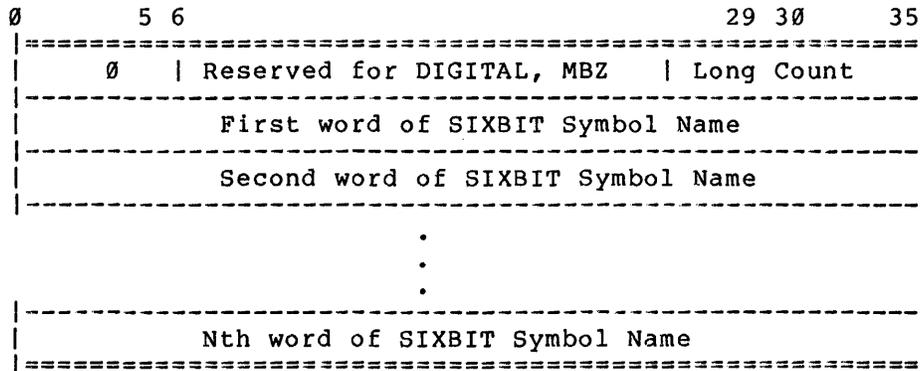
Block Type 1050 creates a PSECT with the given name, if none currently exists. It also assigns a unique index number to the PSECT. This index is binding only in the current module. LINK clears PSECT indexes at the end of each module. PSECT indexes in any given module must be declared in consecutive order starting at index 1.
