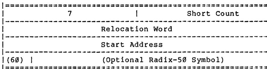
Block Type 7 contains the start address for program execution. LINK uses the start address in the last such block processed by the load, unless /START or /NOSTART switches specify otherwise.
