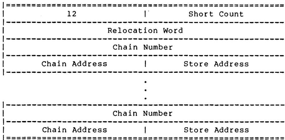
Block Type 12 chains together data structures from separately compiled modules. (The MACRO pseudo-ops `.LINK` and `.LNKEND` generate Type 12 blocks.) Block Type 12 allows linked lists that have entries in separately compiled modules to be constructed so that new entries can be added to one module without editing or recompiling any other module.
