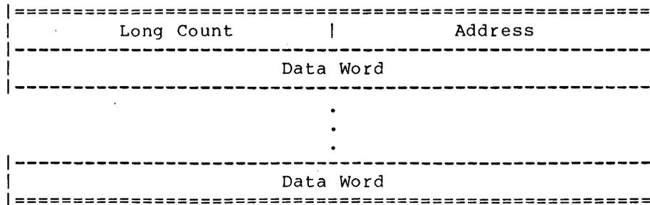
Block Type 21 contains data to be loaded sparsely in a large area. The first word of each sub-block contains the long count for the sub-block in the left half, and the address for loading the data words in the right half.
