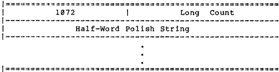
Long Polish Blocks of Type 1072 define Polish fixups for operations on relocatable long external symbols. This Block Type is interpreted as a string of 18-bit operators and operands. The block is in Polish prefix format, with the store operator at the end of the block. Each halfword can contain one of the following:
