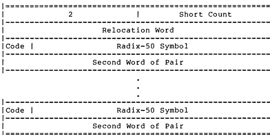
The first word of each pair has a code in bits 0 to 3 and a Radix-50 symbol in bits 4 to 35 (decimal). The contents of the second word of a pair depends on the given code. The octal codes and their meanings are:
