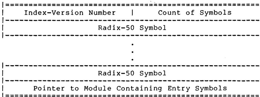
Block Type 14 contains a list of all entry points in a library produced by MAKLIB. The block contains 177 (octal) data words (with no relocation words); if the index requires more entries, additional Type 14 blocks are used. If 177 data words are not needed, zero words pad the block to a length of 177. -1 indicates the end of the sub-block information.
