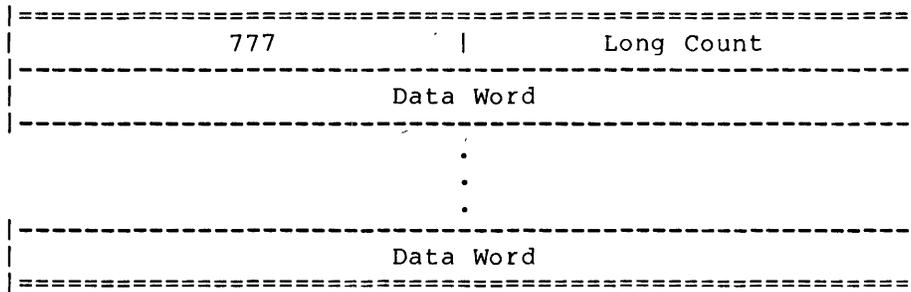
Block Type 777 is included in a universal (UNV) file that is produced by MACRO so that LINK will recognize when a UNV file is being loaded inadvertently. When a Block Type 777 is encountered, LINK produces a ?LNKUNS error.
