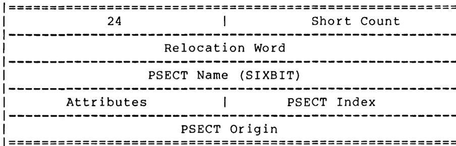
Block Type 24 contains information concerning a specified PSECT. The first word contains the block type number and the number of words associated with the block. The second word contains the relocation information. The third word contains the PSECT name in SIXBIT. The fourth word is the PSECT origin specified for this module.
