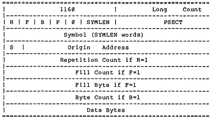
Block Type 1160 supports the loading of data into different PSECTs and sections. This REL block allows separate program units to load data into different bytes in the same word of memory at different times during the loading process.
