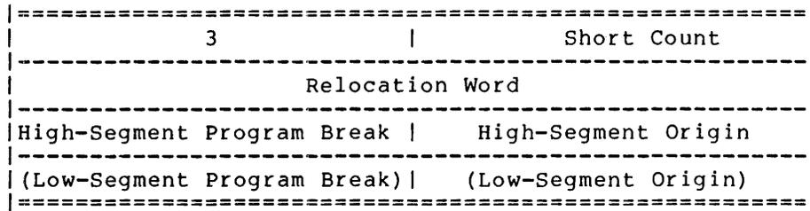
Block Type 3 tells LINK that code is to be loaded into the high segment.
