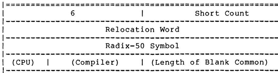
Block Type 6 contains the program name, and must precede any Type 2 blocks. (A module should begin with a Type 6 block and end with a Type 5 block.)
