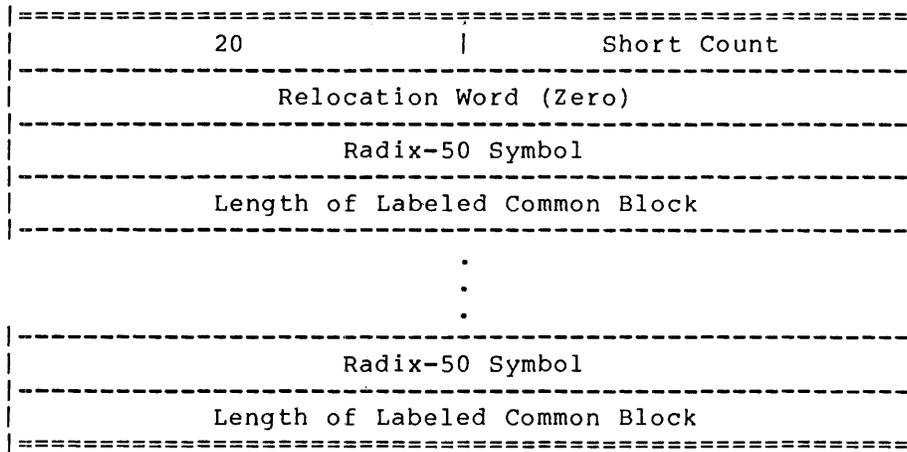
Block Type 20 allocates labeled COMMON areas. The label for unlabeled COMMON is ".COMM.". If a Block Type 20 appears in a REL file, it must appear before any other block that causes code to be loaded or storage to be allocated in the core image.
