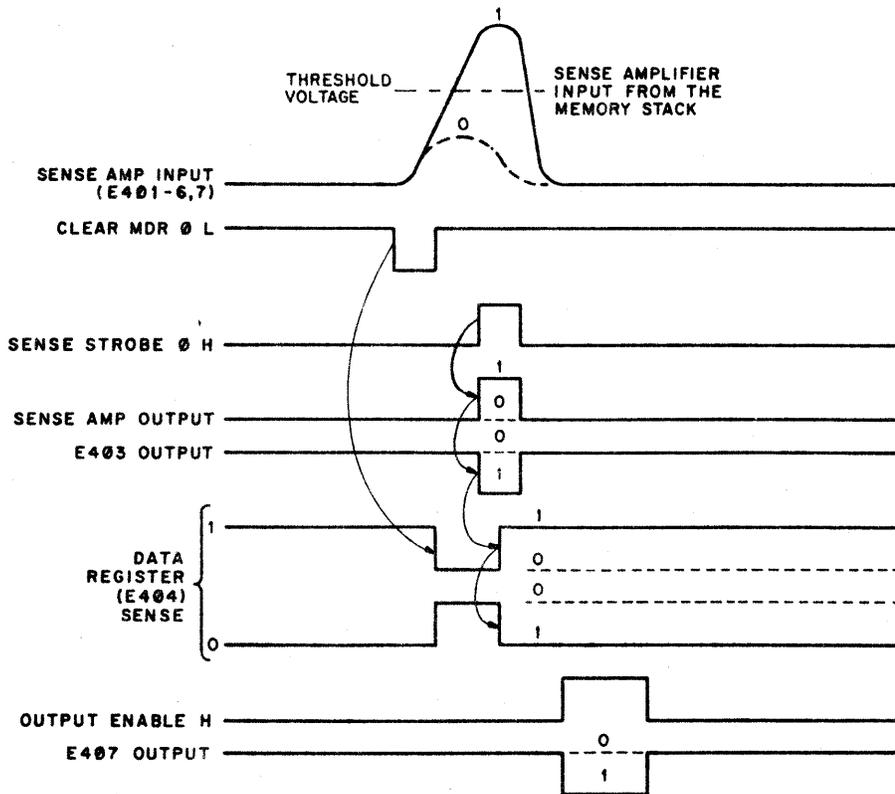
Figure 4-18 Timing Diagram for the Sense Portion of a Read Operation
