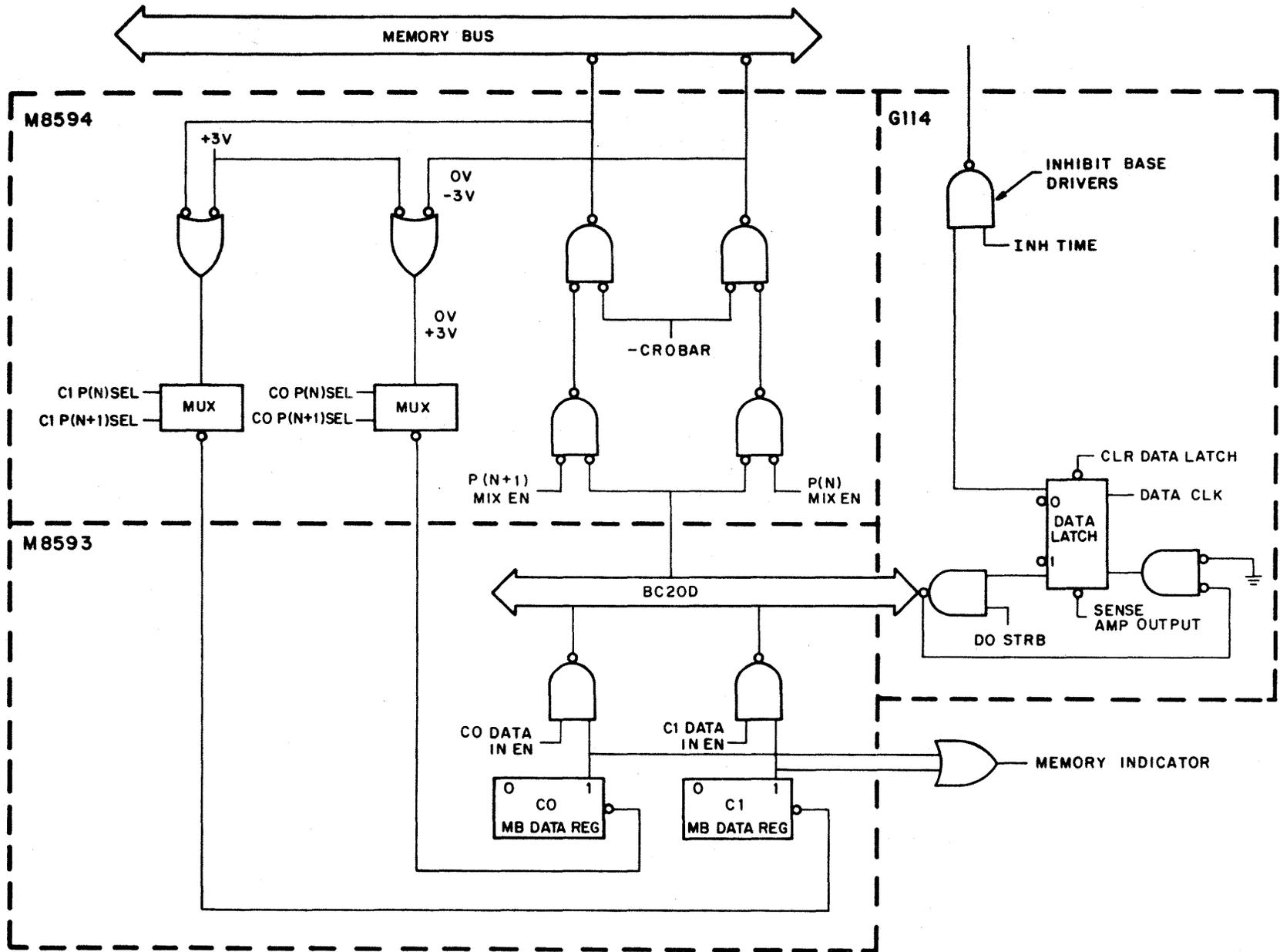
Figure 4-5 Data Path Diagram
