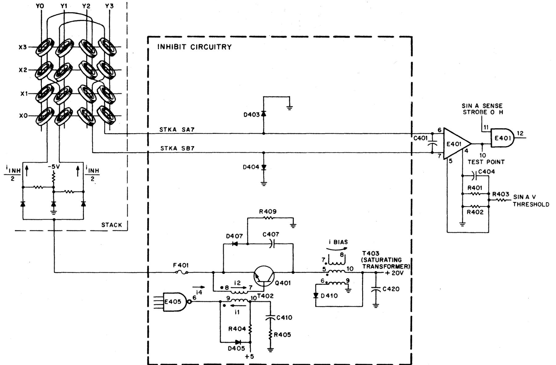
Figure 4-20 Sense Amplifier and Inhibit Driver
