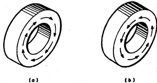
Figure 4-8 Magnetic States of Ferrite Cores
