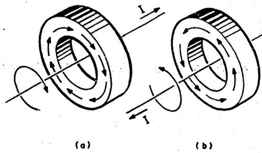
Figure 4-9 Switching Magnetic State of Ferrite Cores
