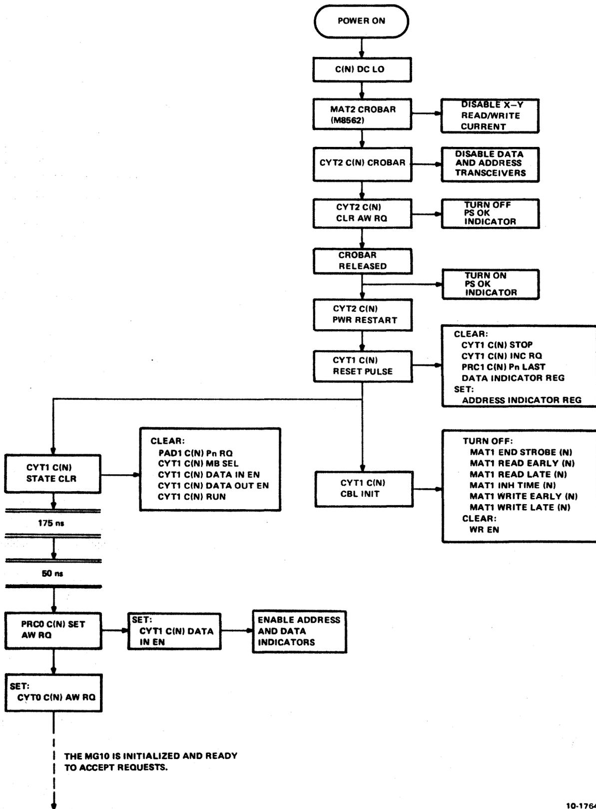
Figure 4-4 MG10 Power-Up Flow Diagram
