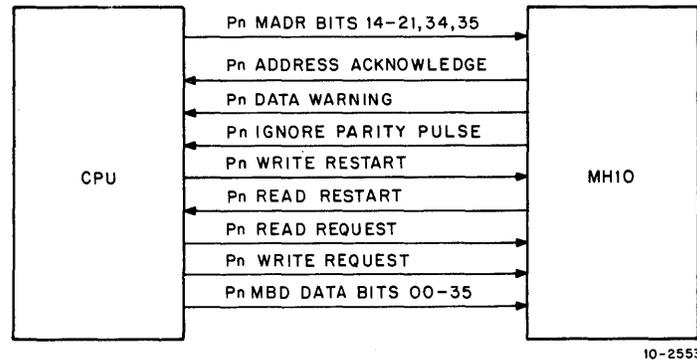
Figure 4-1 Memory Processor Interface
