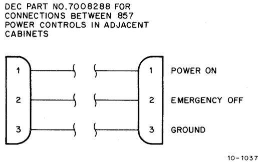
Figure 2-3 Remote Power Control Cable
