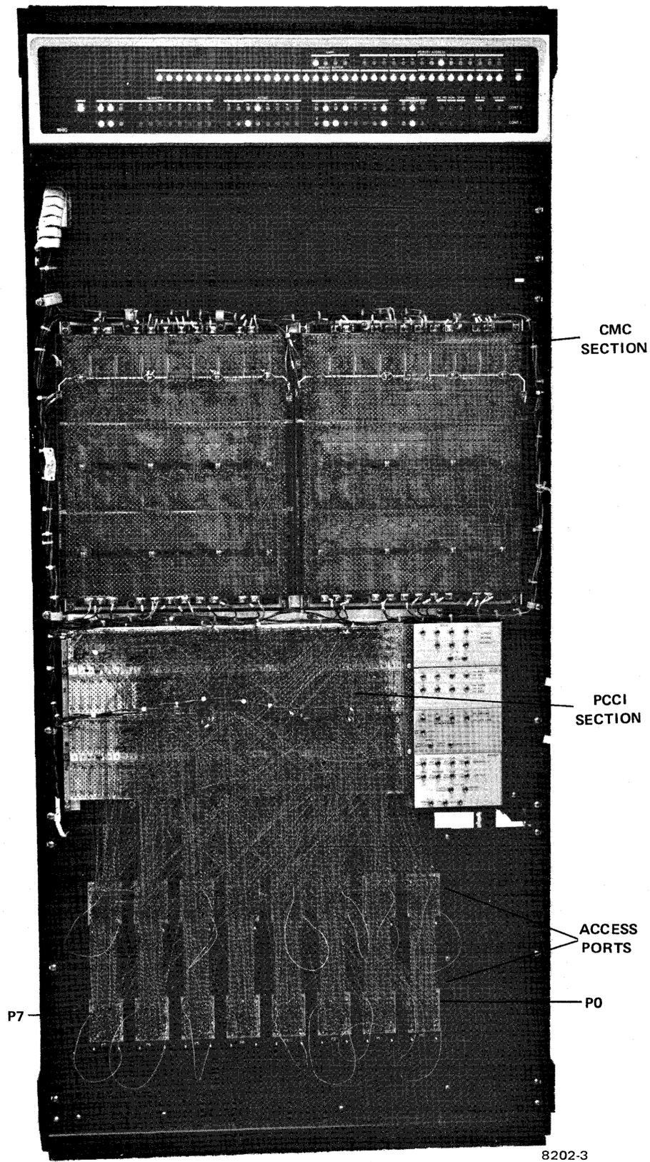
Figure 1-4 MH10 Core Memory, Front View (Door Off)
