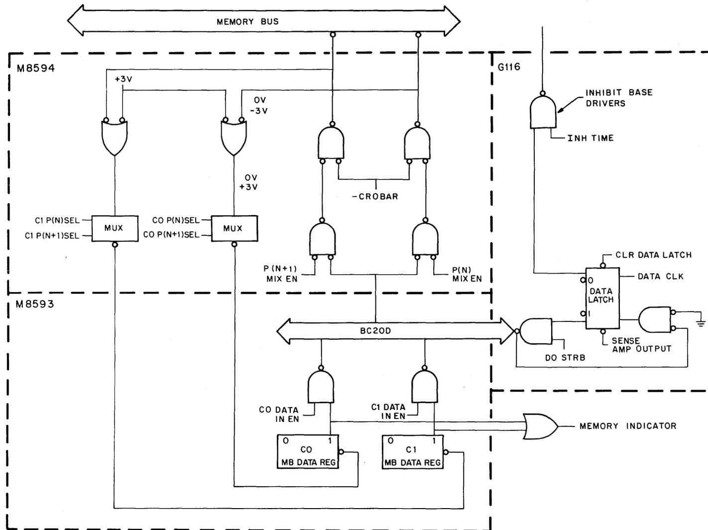
Figure 4-5 Data Path Diagram
