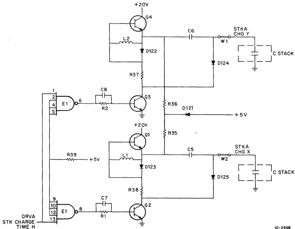
Figure 4-22 Stack Charge Circuit
