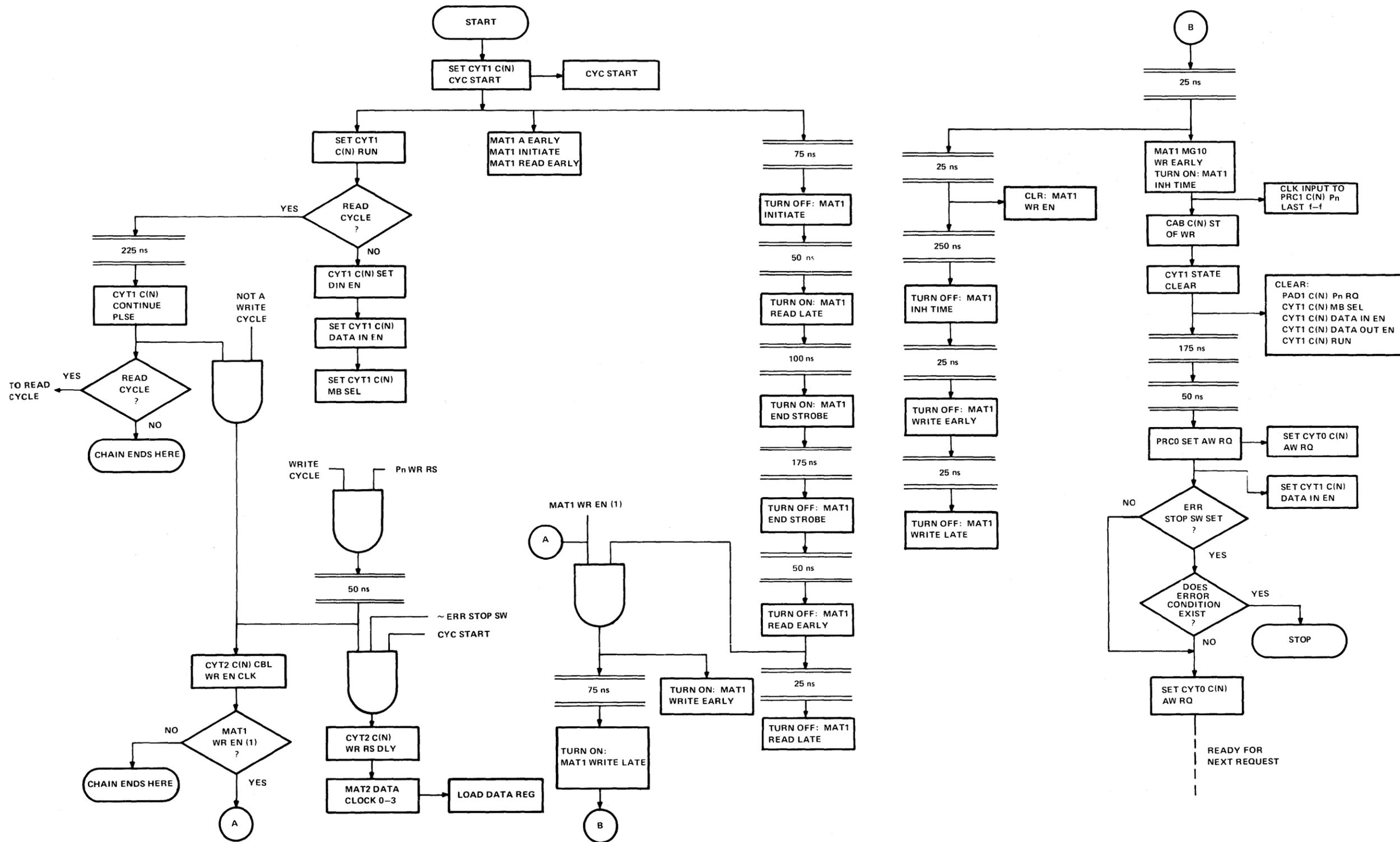
Figure 4-6 Clear Write Timing Flow Diagram
