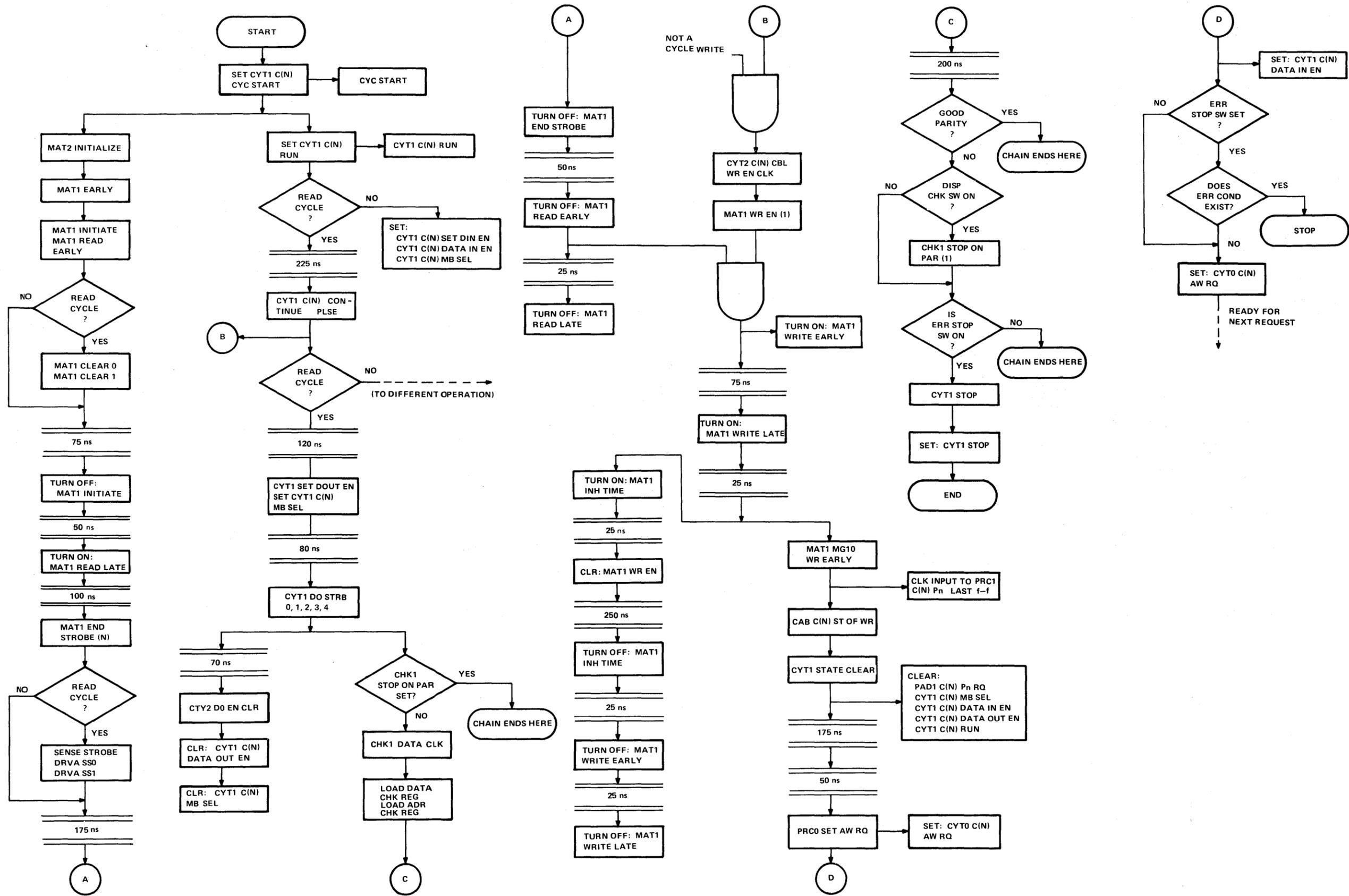
Figure 4-7 Read Restore Timing Flow Diagram
