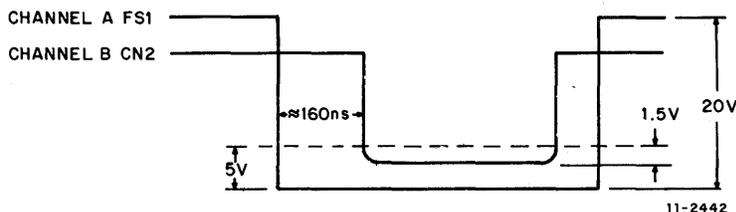
Figure 5-1 Sense Strobe Delay Waveform
