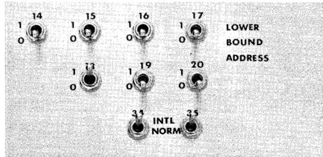
**Figure 3-3 Memory Address Switches**
