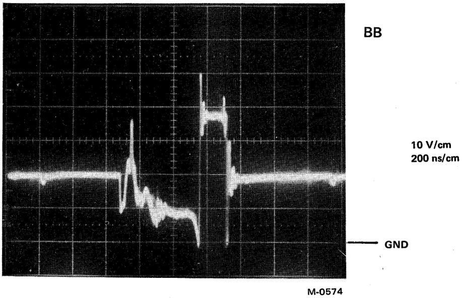
Figure 5-6 Drive Module Waveforms (Sheet 1 of 5)
