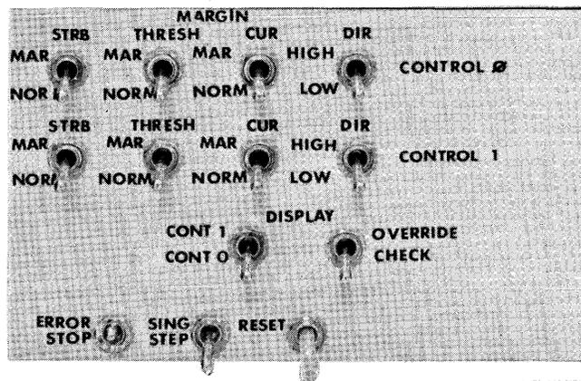
**Figure 3-4 Maintenance Panel (Maintenance Section)**
