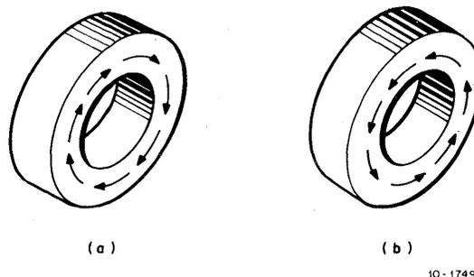
Figure 4-8 Magnetic States of Ferrite Cores
