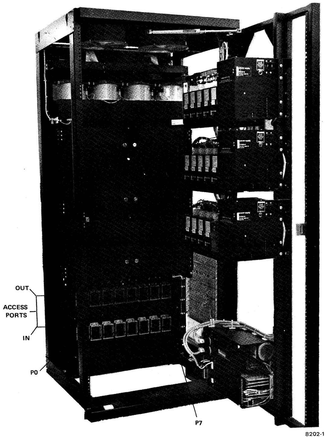
Figure 1-3 MH10 Rear View (Access Ports)
