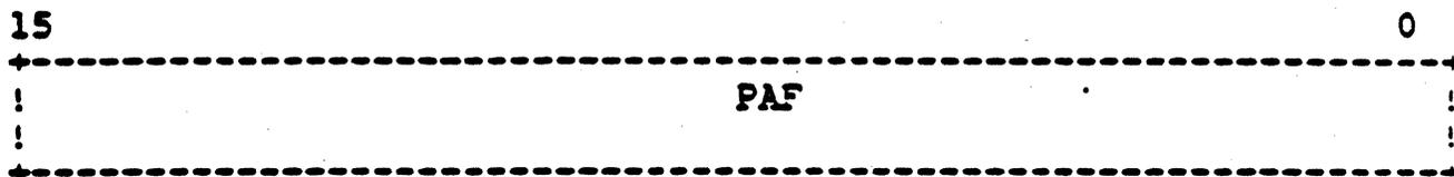
All bits are read/write. These registers are not affected by console start or a RESET instruction. Their state at power up is UNDEFINED.
