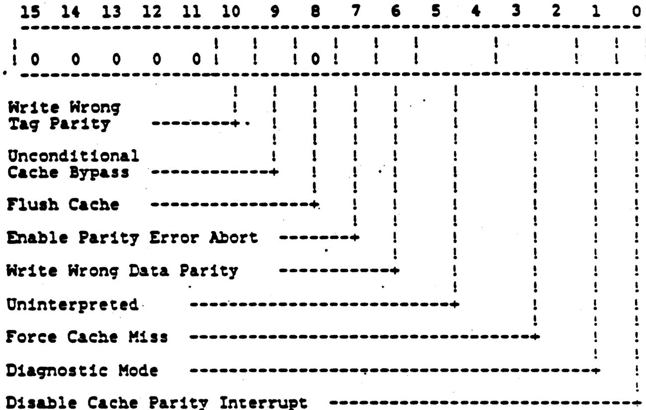
Bits <15:11> always read as zeros. Bits<5:4,1> are read/write but are not interpreted by the KDJ11-B.
