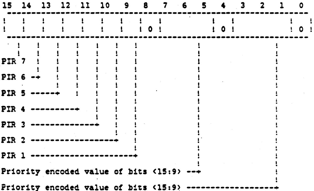
PIRQ bits <15:9> are read/write, bits <7:5,3:1> are read-only and the remaining bits always read as zeroes. PIRQ is cleared at power up, by a console start and by the RESET instruction.
