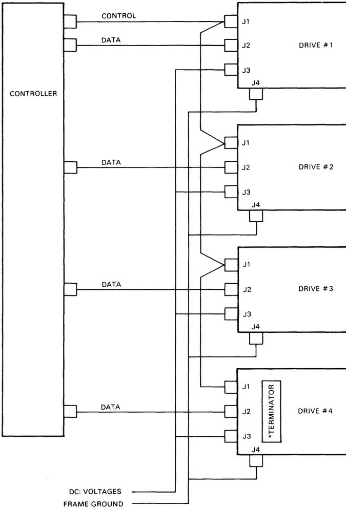
\*THE LAST OR ONLY DRIVE IN THE CONTROL CABLE STRING MUST HAVE THE TERMINATOR RESISTOR PACK INSTALLED. ALL OTHER DRIVES MUST HAVE THEIR TERMINATORS REMOVED.
