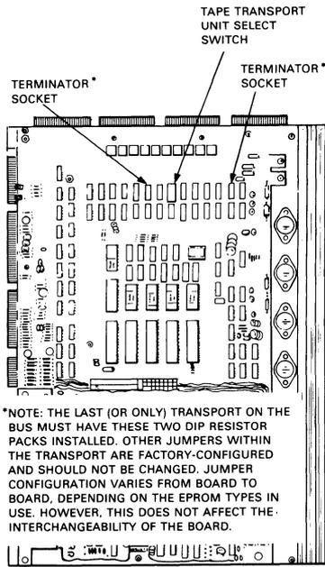
\*NOTE: THE LAST (OR ONLY) TRANSPORT ON THE BUS MUST HAVE THESE TWO DIP RESISTOR PACKS INSTALLED. OTHER JUMPERS WITHIN THE TRANSPORT ARE FACTORY-CONFIGURED AND SHOULD NOT BE CHANGED. JUMPER CONFIGURATION VARIES FROM BOARD TO BOARD, DEPENDING ON THE EPROM TYPES IN USE. HOWEVER, THIS DOES NOT AFFECT THE INTERCHANGEABILITY OF THE BOARD.
