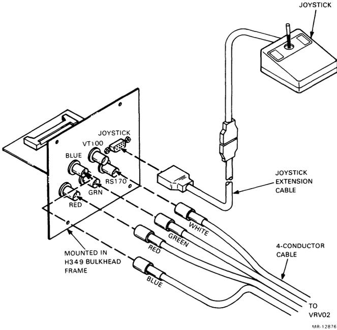
Joystick Installation and 4-Conductor Cable Connection
