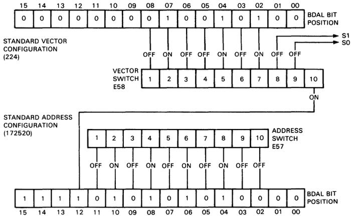
S0 = EXTENDED FEATURES (MUST BE "ON" FOR 22 BIT ADDRESSING)
