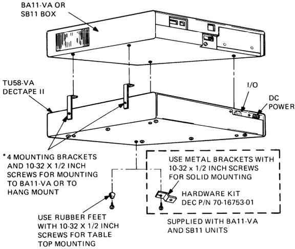
\* TO ATTACH BRACKETS TO BA11-VA OR SB11, MOUNT BRACKETS TO BA11-VA (SB11) FIRST.
