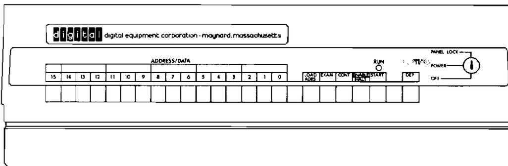
Figure 1-4 The PDP-11/10 Console
