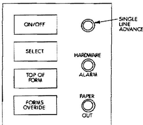
Figure 1-9 LS11 Operator Panel
