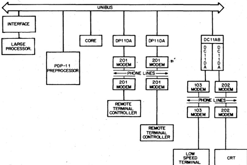
Figure 2-1 Front End Processor
