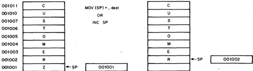
Figure 5-6: Byte Stack used as a Character Buffer
