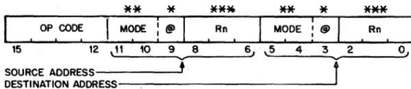
\* = DIRECT/DEFERRED BIT FOR SOURCE AND DESTINATION ADDRESS
