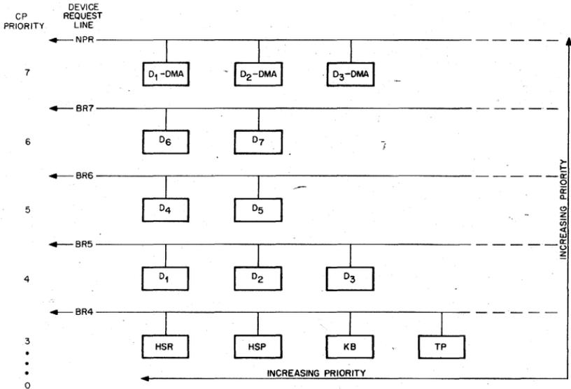
See Table 1-1, page 2, for a summary of the API structures of the various PDP-11's. Bus requests from external devices can be made on one of five request lines. Highest priority is assigned to non-processor request (NPR). These are direct memory access type transfers, and are honored by the processor between bus cycles of an instruction execution.
