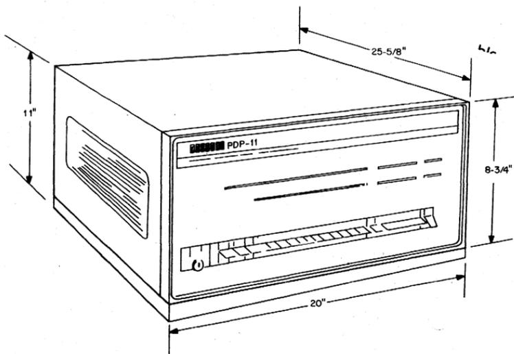
Figure 6.3 Table Top PDP-11 Dimensions
