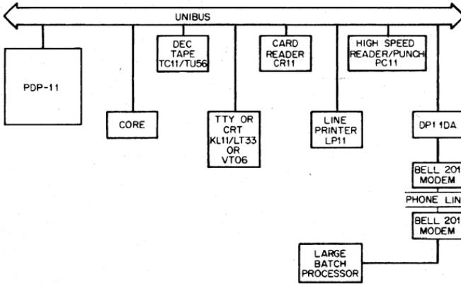
Figure 2-3 Remote Terminal Controller
