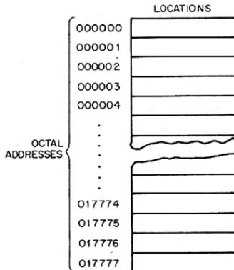
Because PDP-11 memories are designed to accommodate both 16-bit words and 8-bit bytes, the total number of addresses does not correspond to the number of words. A 4096-word memory can contain 8,192 bytes and consists of 017777 octal locations. Words always start at even-numbered locations.
