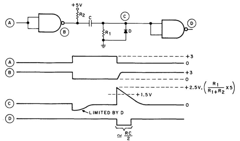
Figure B-10 Negative Edge Triggered One-Shot (Pulser)
