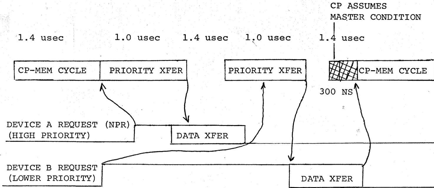
CONDITIONS - Two Devices request just after CP-MEM Transfer starts, Device A does transfer, then Device B, then Control is returned to CP.
