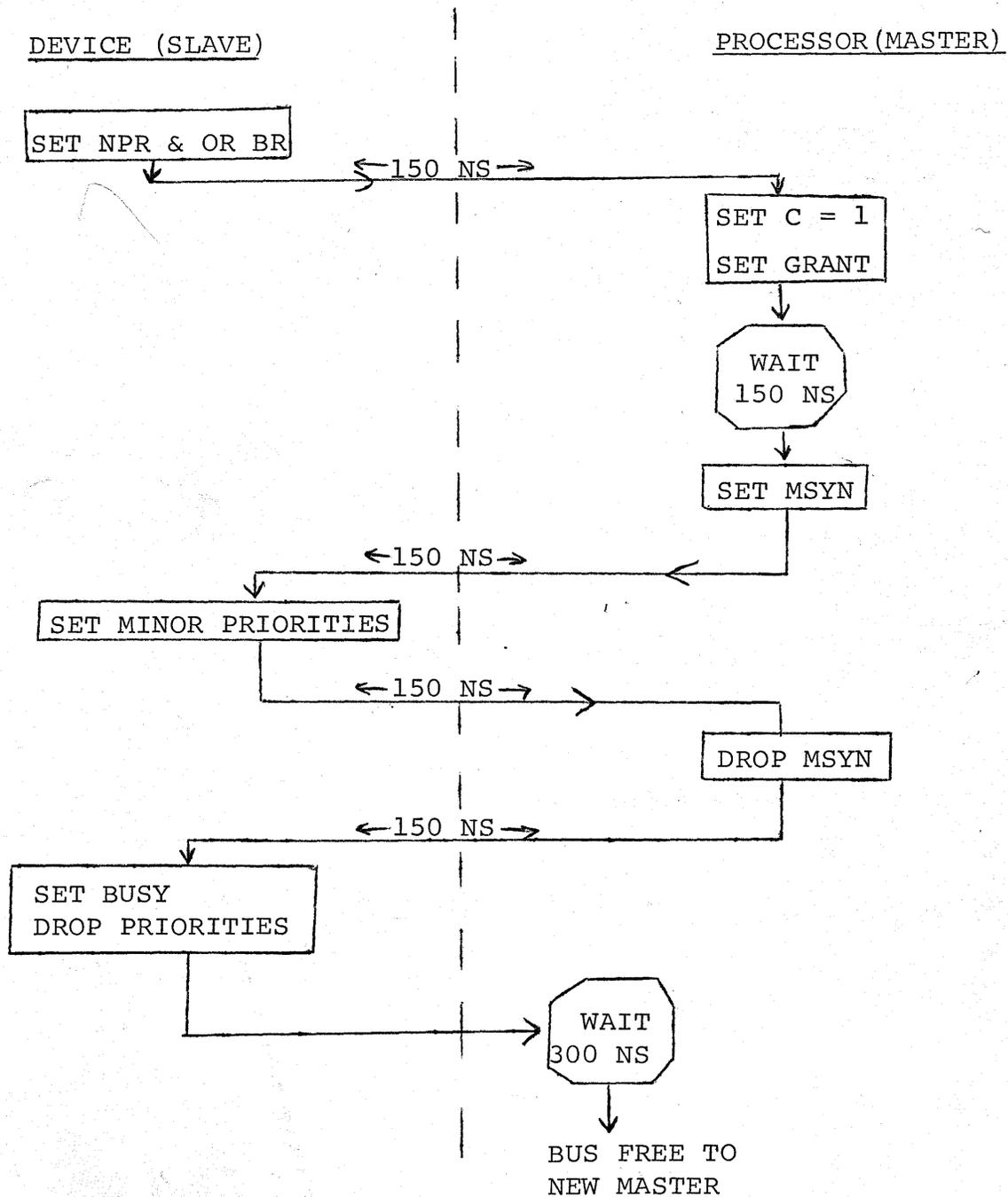
$$\text{PRIORITY BUS TRANSFER} = (5 \times 150 \text{ NS}) + 300 \text{ NS} = 1.05 \text{ usec}$$
