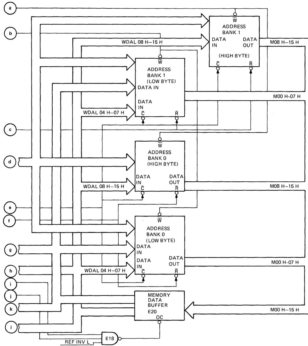
Figure 4-16 RAM Module, Simplified Function Diagram
