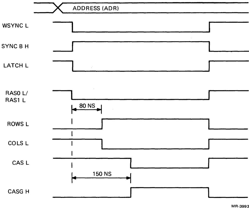
Figure 4-21 Row/Column and Address Multiplexer, Timing Diagram
