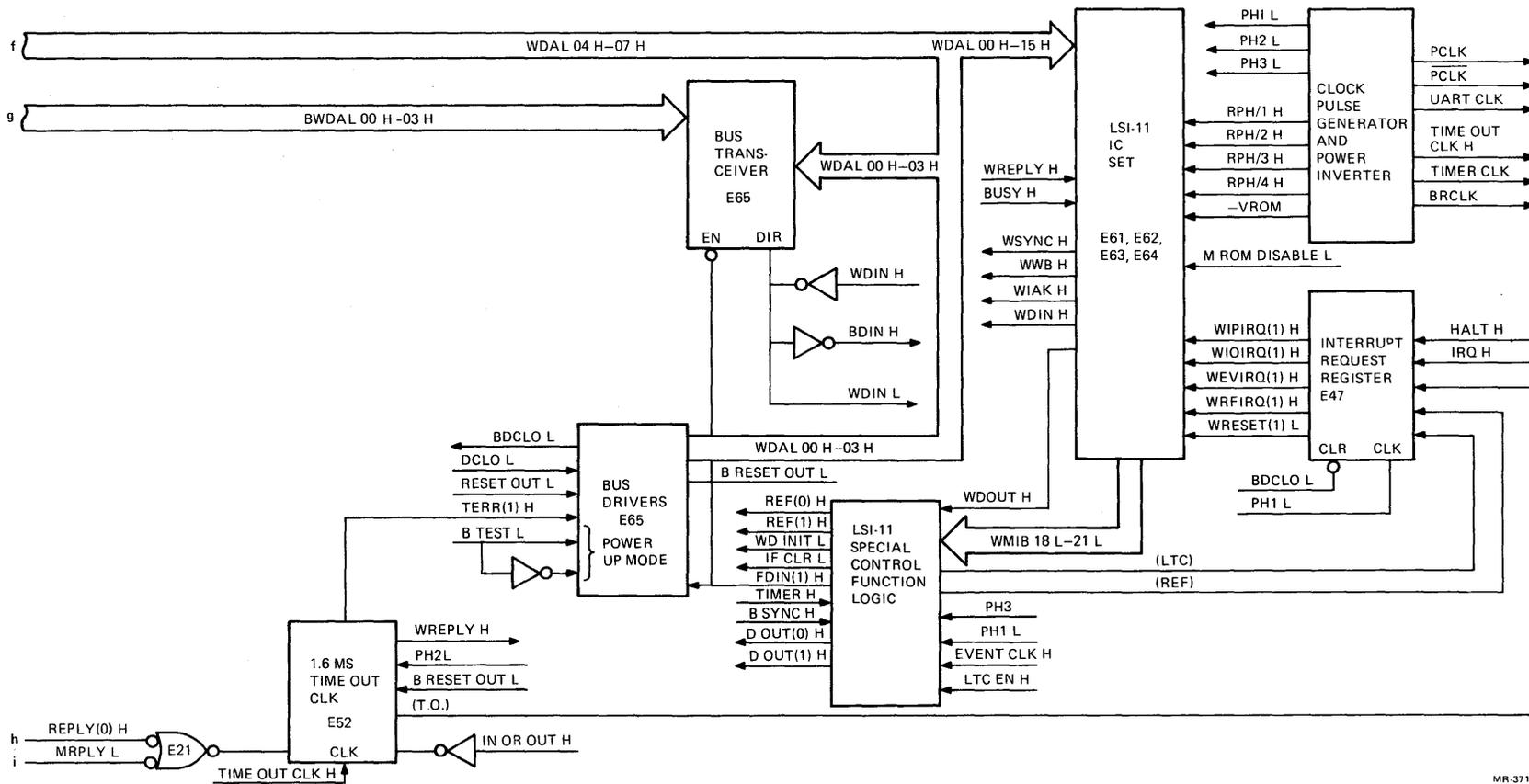
Figure 4-4 Intelligence Module, Simplified Signal Diagram (Sheet 3 of 3)
