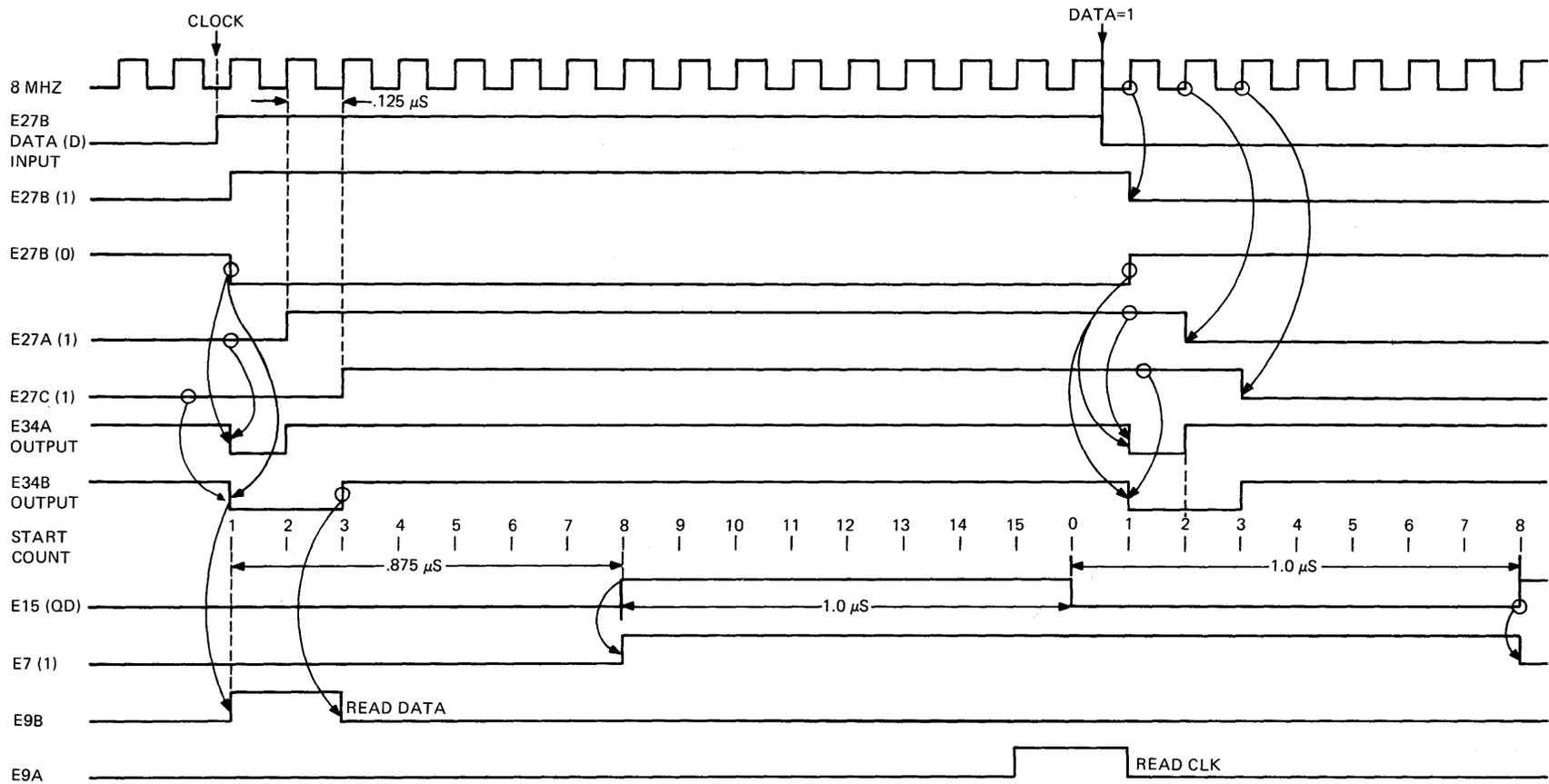
Figure 4-41 Data Separator Circuit (Revision K), Timing Diagram
