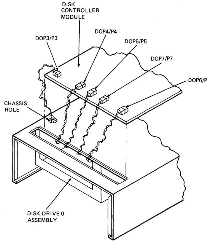
Figure 5-31 Disk Drive Cable Routing
