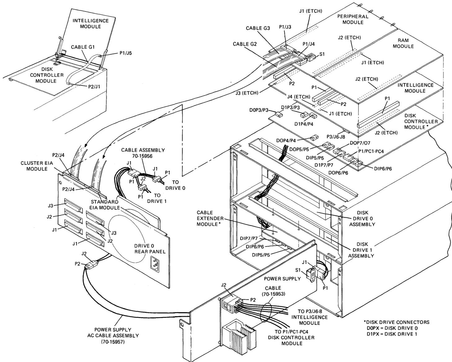
Figure 5-3 PDT-11/150 Internal Cables and Connectors
