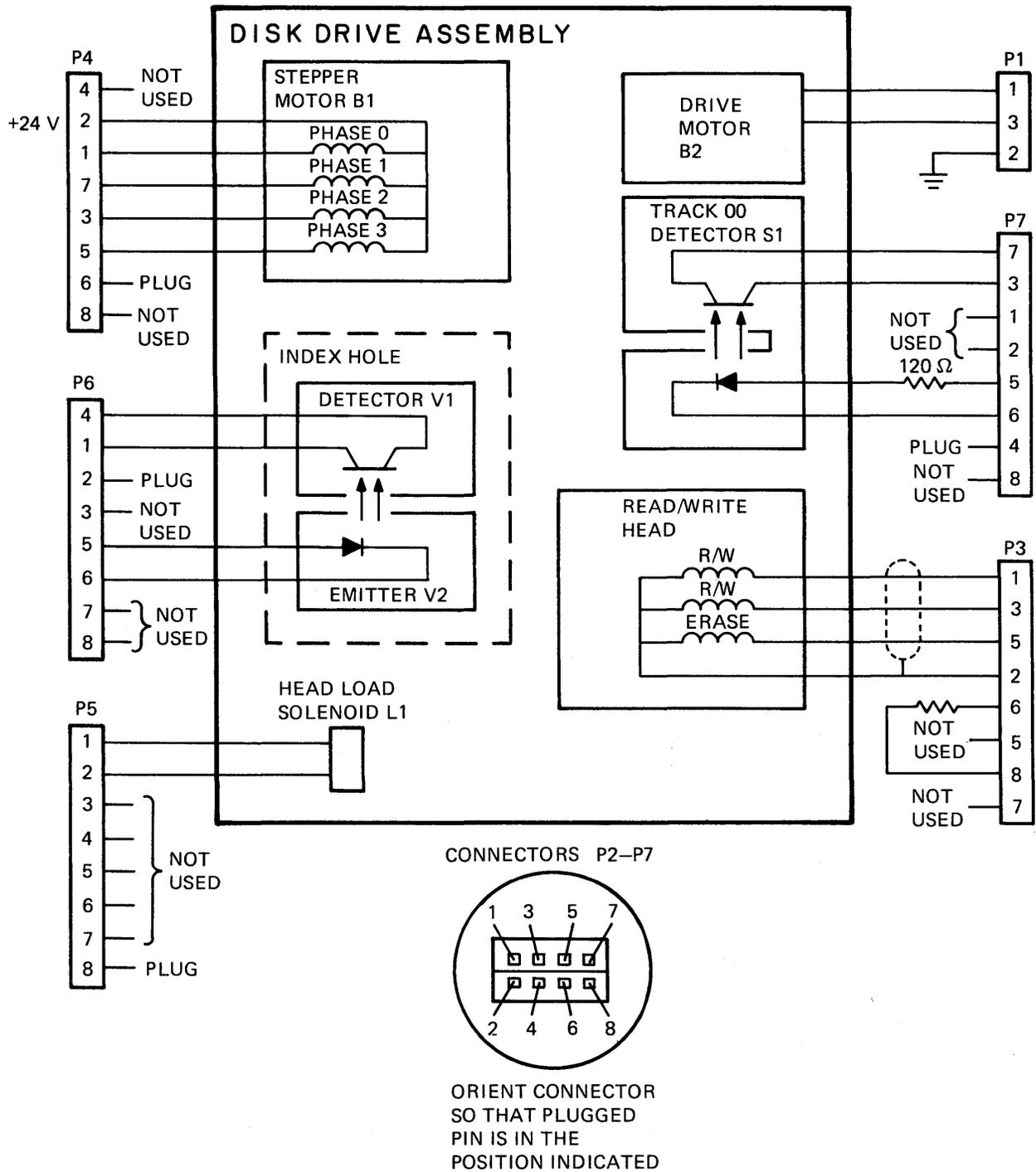
Figure 5-47 Disk Drive Assembly, Wiring Diagram
