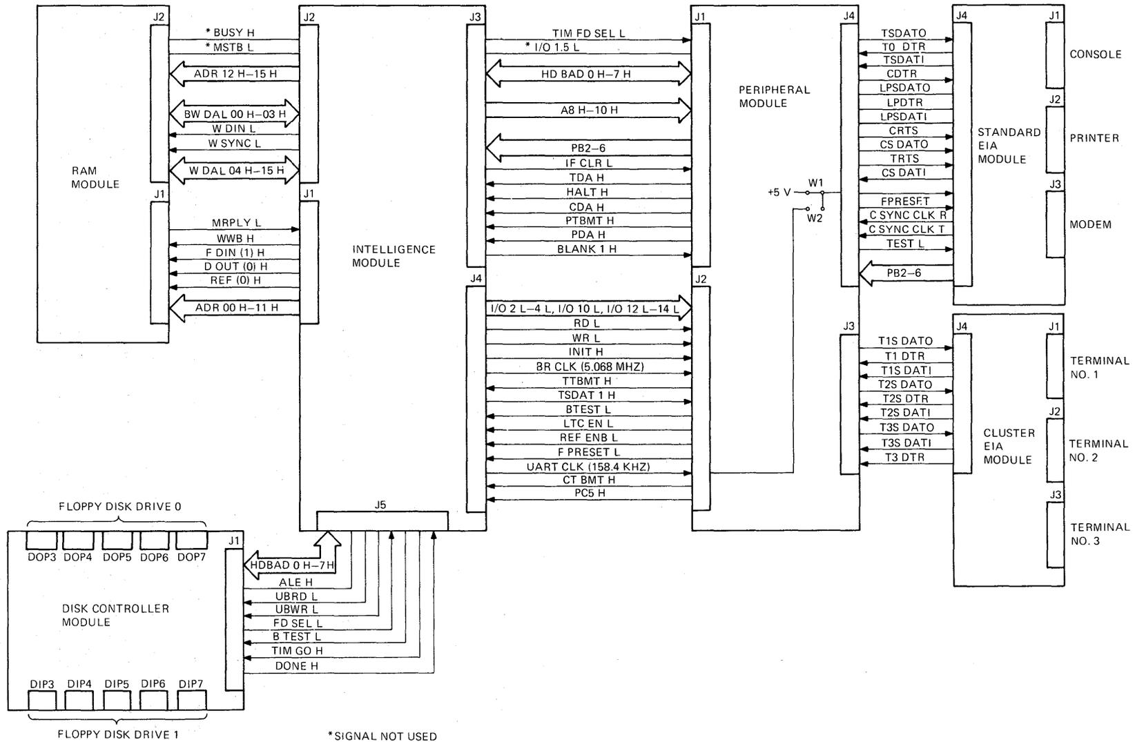
Figure 4-3 PDT-11/150 Internal Signal Distribution
