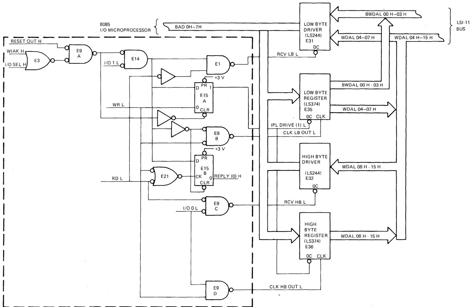
Figure 4-7 IPL and Control Logic, Simplified Diagram
