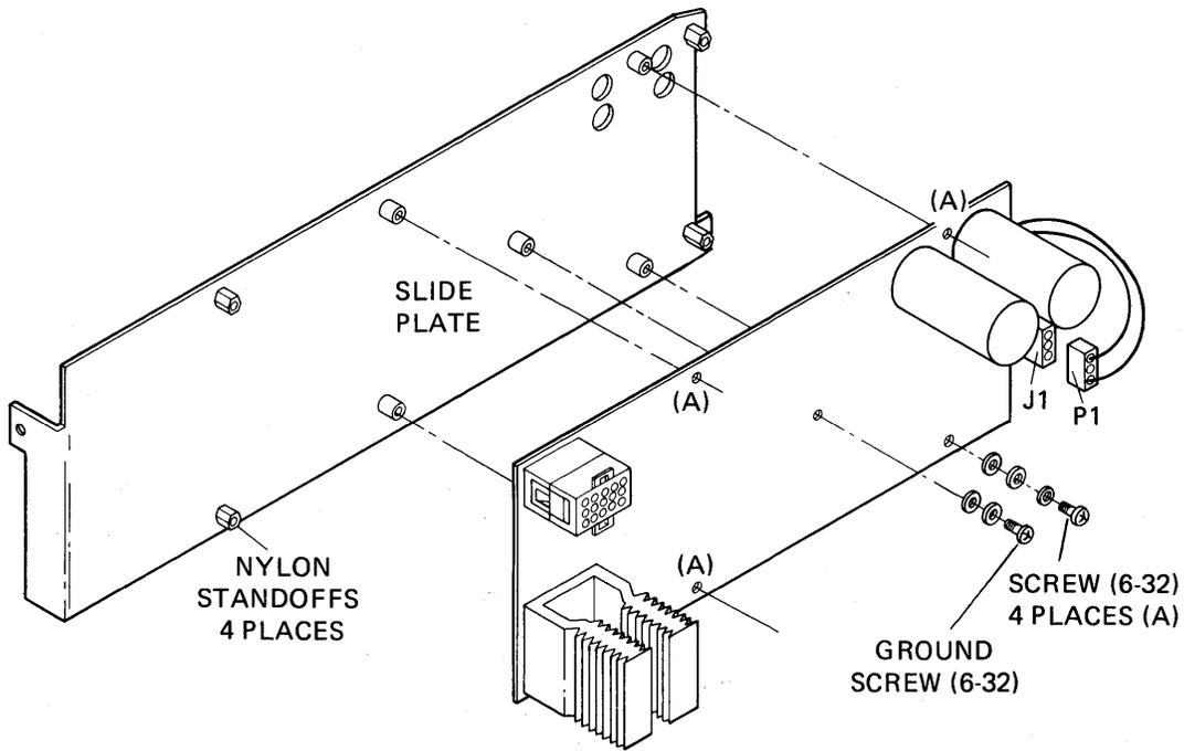
Figure 5-34 Power Supply Module, Removal and Replacement
