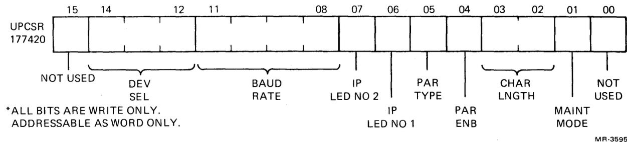
Figure 6-3 USART Parameter Control Register UPCS R Format
