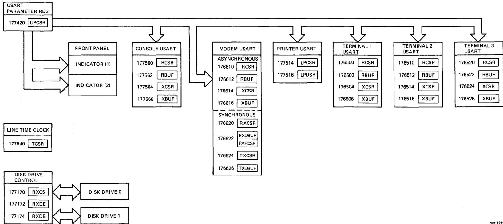
Figure 6-2 PDT-11/150 Device Register Address Assignments
