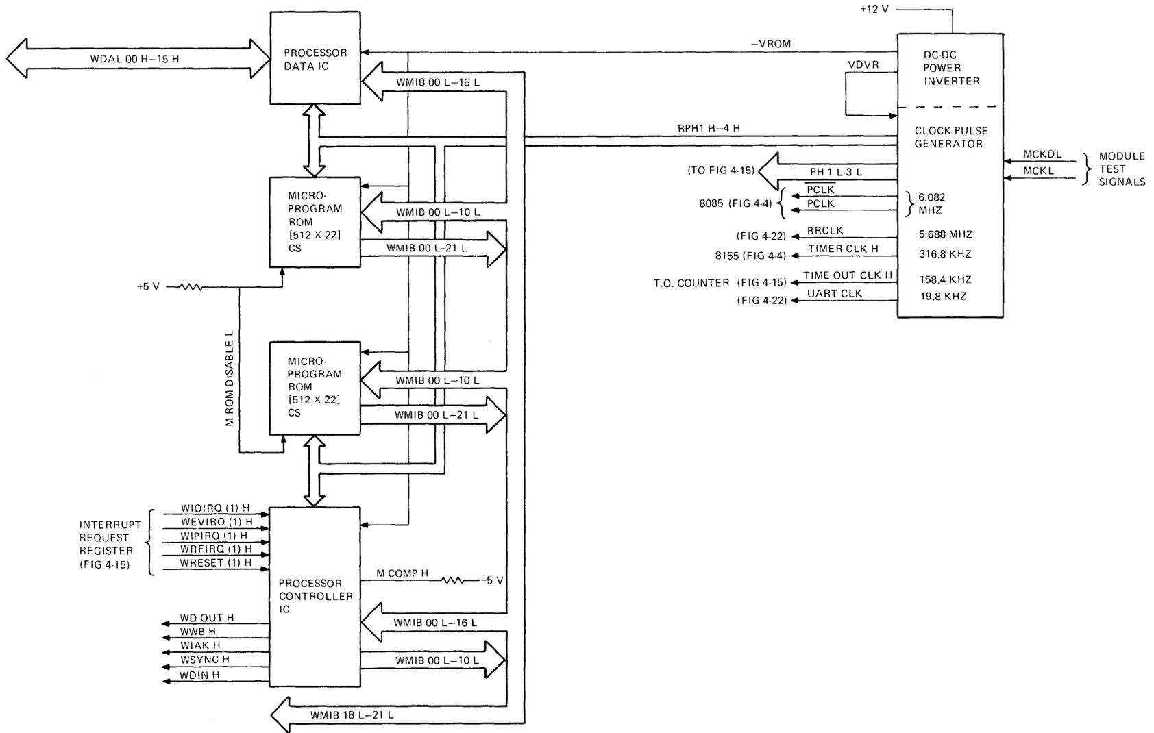
Figure 4-8 LSI-11 Microprocessor, Simplified Block Diagram
