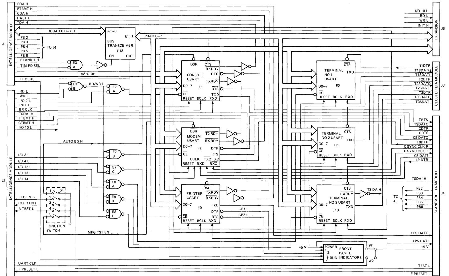
Figure 4-22 Peripheral Module, Simplified Function Diagram
