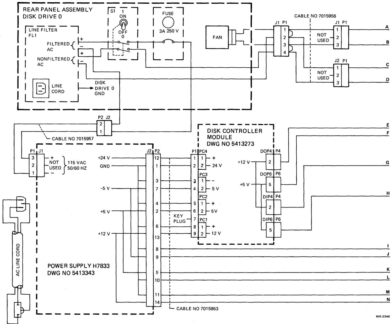
Figure 5-5 AC/DC Power Distribution, 60 Hz Units
