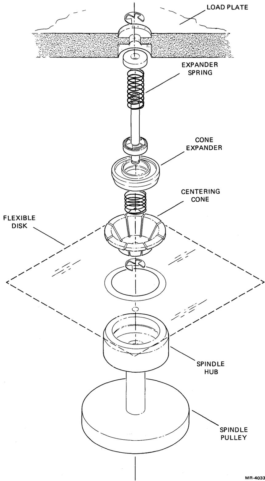
Figure 5-49 Centering Cone and Spindle Drive Components
