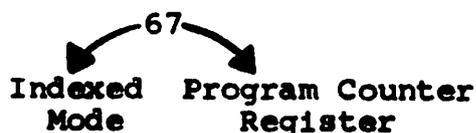
RELATIVE MODE is used whenever direct reference is made to a memory location, and is assembled as Indexed Mode using the Program Counter. Because the content of the Program Counter is used in the address calculation, the address of the operand is not absolute; it is RELATIVE to the address of the instruction.
