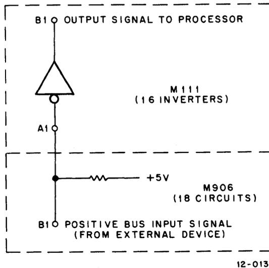
Figure 5-23. Typical M111/M906 Positive Input Circuit
