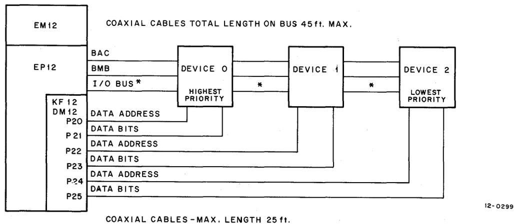
\* If the priority interrupt system is used in the KF12B this cable is connected separately from each device. (ref. BS-KF12-CAB).
