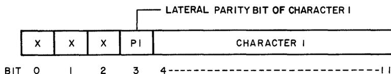
*Read/Compare* – A direct comparison of the characters on tape is made with those in memory. The parity bit is ignored, as are bits 0-3 in each memory word.
