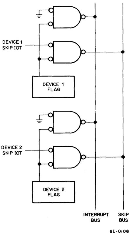
Figure 5-12. Multiple Inputs to IOS and PI Facilities
