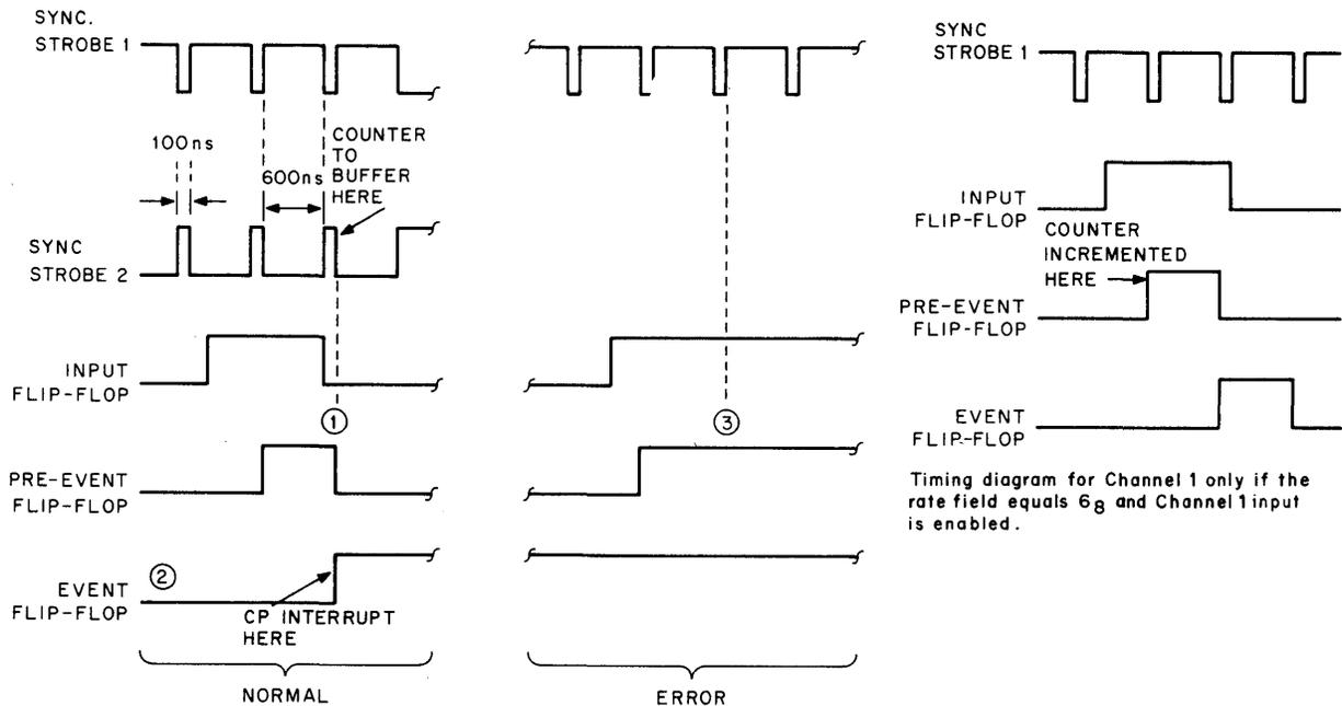
Timing diagram for Channel 1 only if the rate field equals 6g and Channel 1 input is enabled.
