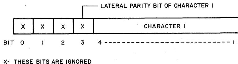
*Read* – A word is read into memory from tape with the following format:
