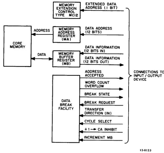
Figure 5-16. Data Break Transfer Interface Block Diagram
