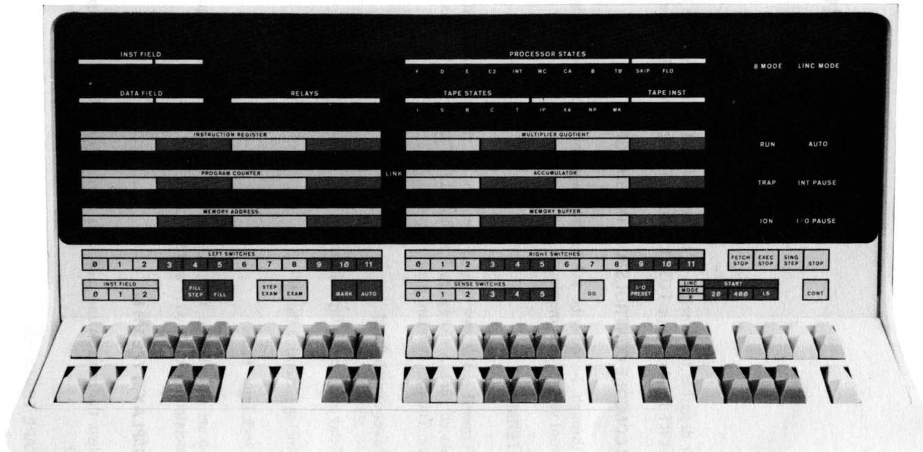
Figure 2-1. PDP-12 Operator console
