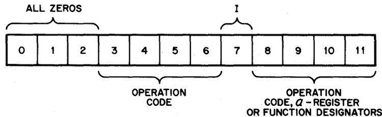
Figure 3-5.  $\alpha$ -Class and Non-Memory Reference Format
