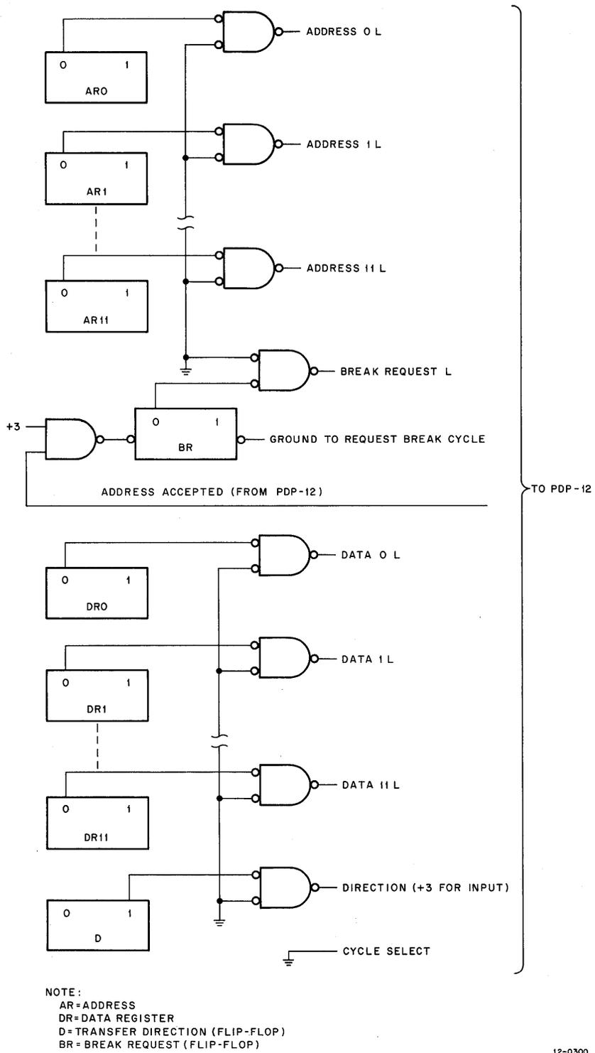
Figure 5-18. Device Interface Logic for Single-Cycle Data Break Input Transfer
