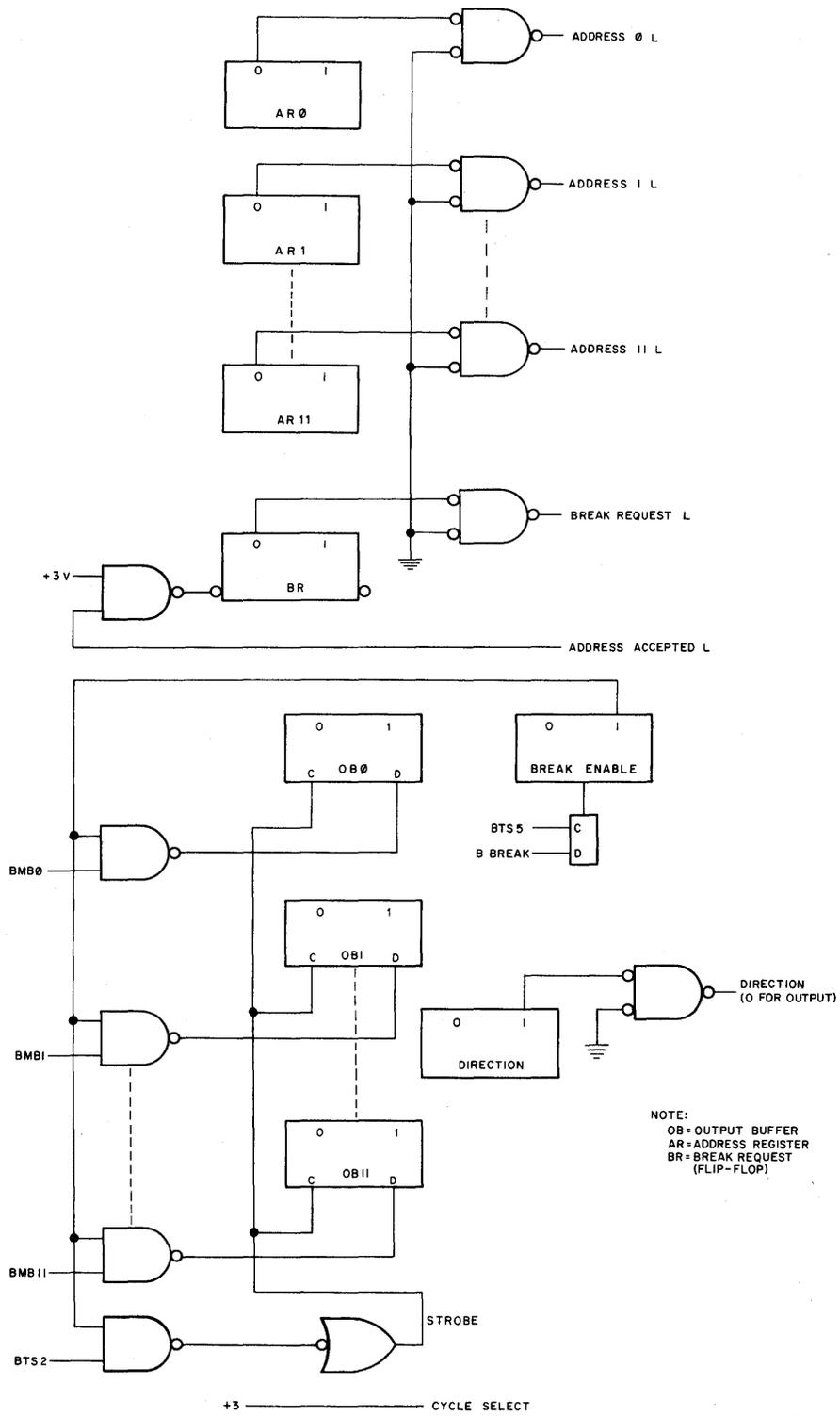
Figure 5-20. Device Interface Logic for Single-Cycle Data Break Output Transfer
