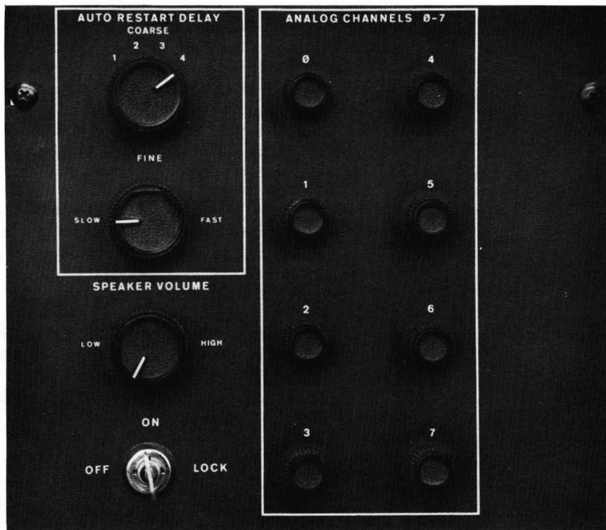
Figure 2-2. Analog Knobs and Power Switch Panel
