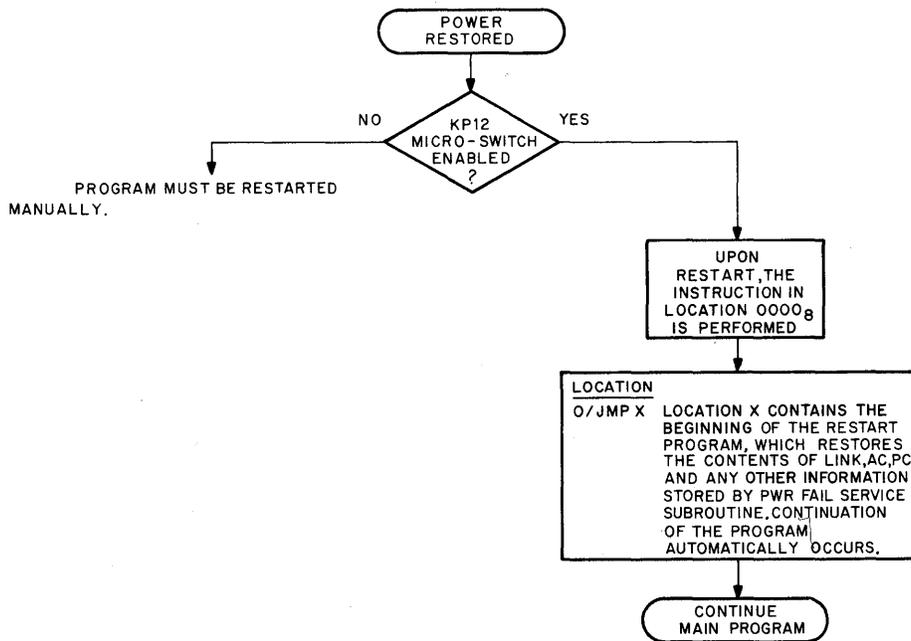
Figure 6-10. Typical Power Failure Program Service Routine
