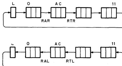
Figure 4-4. Rotation Scheme for RAR, RTR, RAL, RTL
