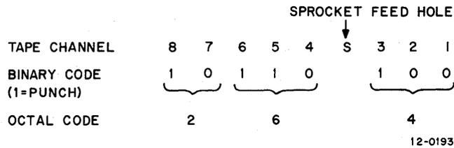
Figure 6-2. Punched Paper Tape Format for the Number 4
