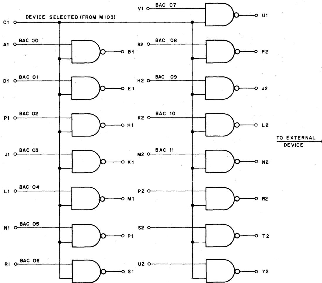
Figure 5-28. M101 Bus Data Interface Logic Circuit
