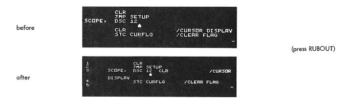
In the same manner, characters may be inserted in a line of text. Turn Knob 3 to locate the cursor under the character that is to immediately precede the first new character. As the additions are typed, they are echoed on the Teletype and scope.
