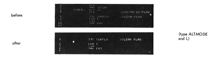
To delete a large section of code that can not be displayed on the scope all at once use the following procedure:
