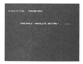
allows the user to specify a minimum value of intensity below which no peak will be looked at.
