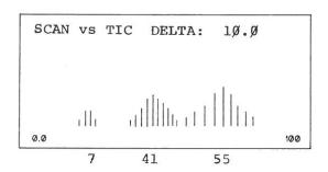
Assuming a gas chromatograph was used, scans 7, 41, and 55 would be representative of the three chromatograph peaks. The files ("SAMPLE.7" "SAMPLE.41" and "SAMPLE.55") could then each be examined in turn. In this way, much spurious data can be eliminated.
