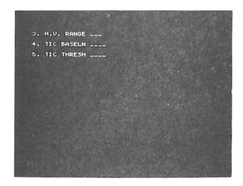
Question 3: The range of values is Ø-999. This number is a measure of the tolerable drift for Hall Voltages between successive calibrations; a good value is 5 for a 12 bit A/D, 20 for A 15 bit A/D.
