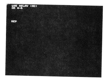
where REP is an abbreviation for REPLY. All input for the remainder of SETUP is echoed on the Teletype and displayed opposite the word REP on the scope. All questions are displayed in the top left of the scope face. The format of the reply to RELAY is
