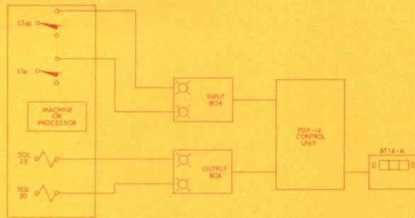
STEP 1. If the indicator lamp for Solenoid 25 on the O-Box is *off*, look at the indicator lamps on the input box for LS<sub>10</sub> and LS<sub>16</sub>.
