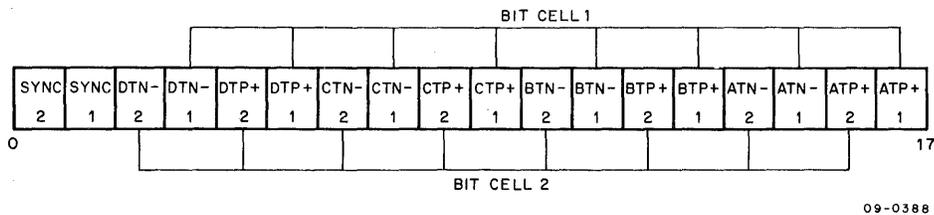
Figure 2-7 AC Bit Usage for IOT DGSS
