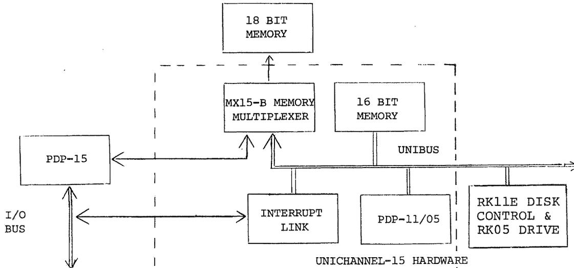
Figure 1-2 Unichannel-15 Hardware
