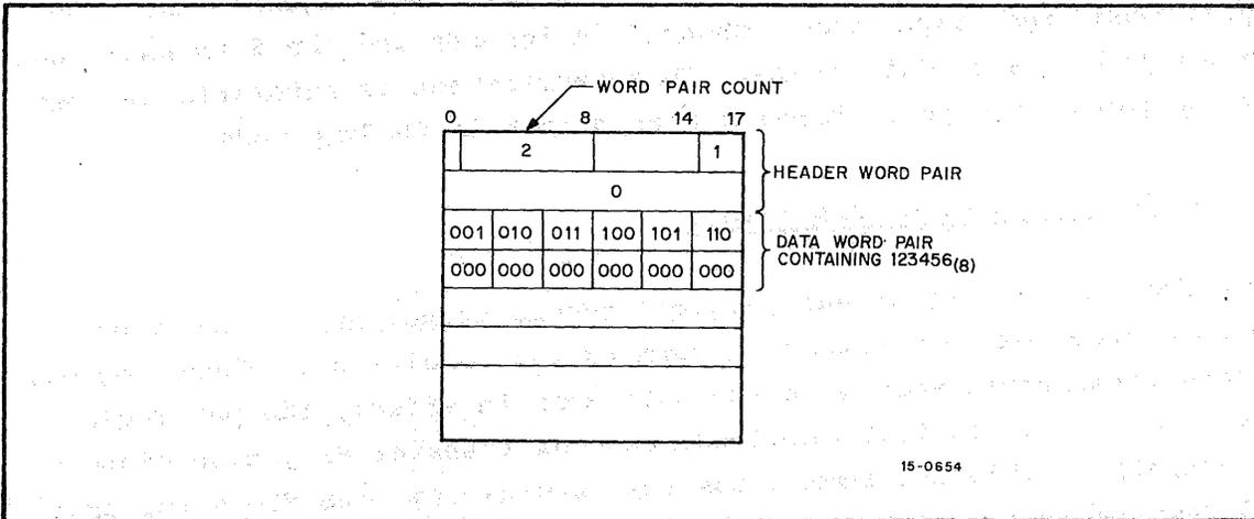
Figure 6-10 Image Binary in I/O Buffers and on Mass Storage Devices
