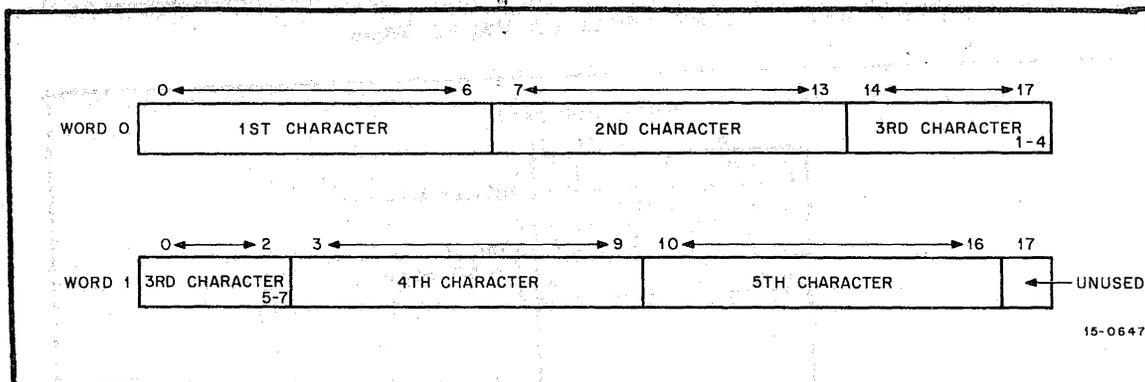
Figure 6-3 5/7 ASCII Packing Scheme
