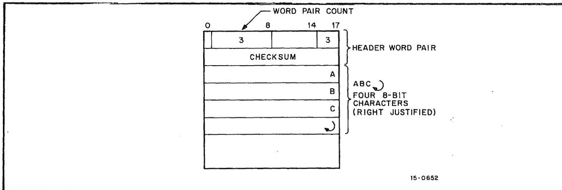
Figure 6-8 Image Alphanumeric Data in I/O Buffers and on Mass Storage Devices
