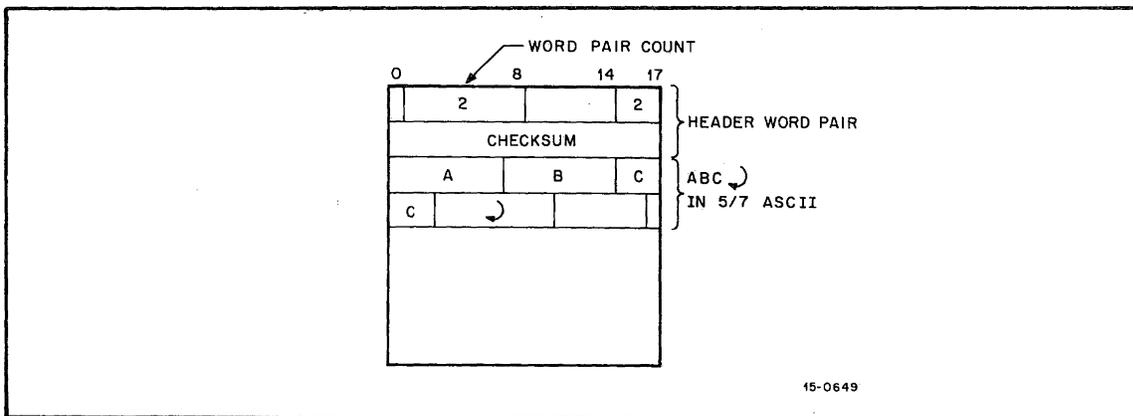
Figure 6-5 IOPS ASCII in I/O Buffers and on Mass Storage Devices
