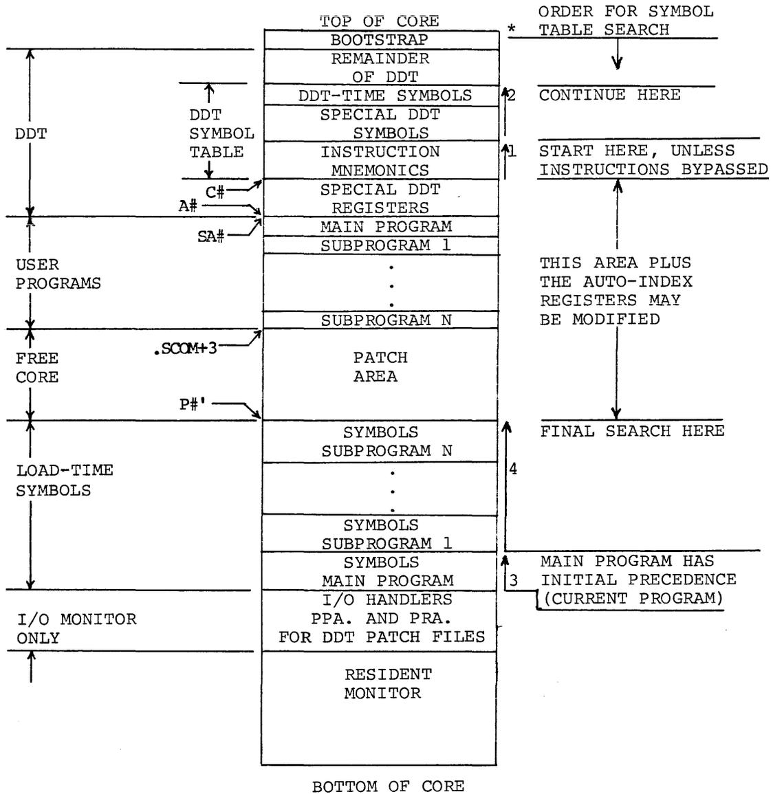
\*On a PDP-15 with 12K, 20K or 28K or core, the bootstrap is located at the top of the next to highest 4K page.
