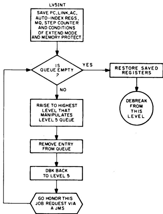
Figure 4-1. Structure of API Software Level Handler
