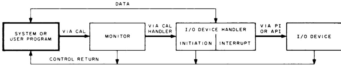
Figure 1-1. General I/O Communication in Monitor Environment
