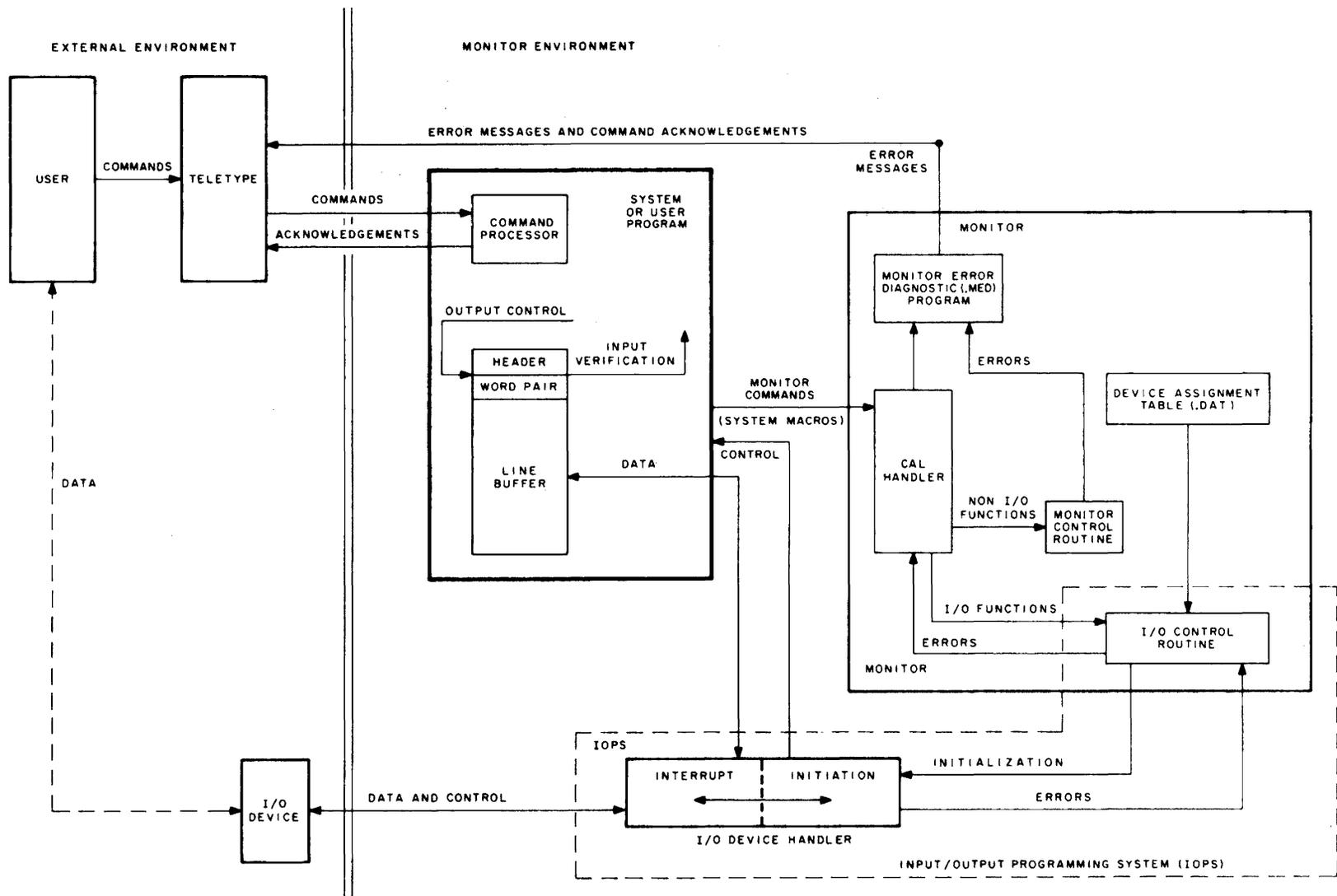
Figure 1-2. Command, Control, and Data Flow in the Basic I/O Monitor Environment
