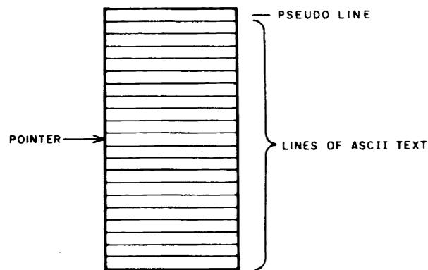
Figure 2-1. Line Buffer and Software Pointer
