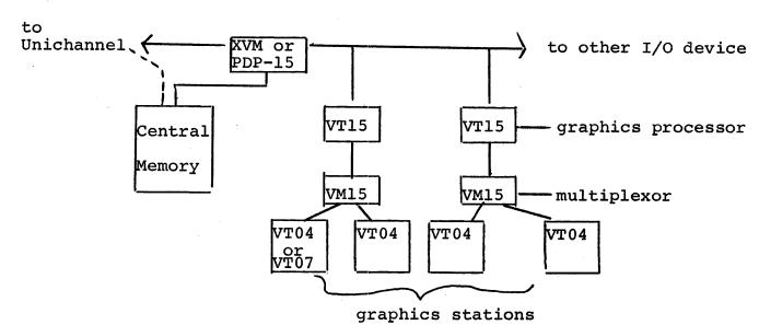
The display terminals are independently programmed from four separate tasks. Each task uses its own copy of VTPRIM, a set of FORTRAN-callable routines for drawing lines, text, and other pictoral representations on a VT04 or VT07.
