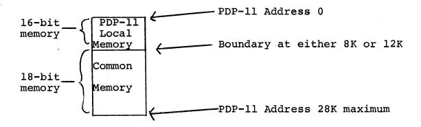
Use of a larger PDP-11 having memory management removes several constraints and allows the PDP-11 physical address space to look like this:
