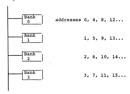
Interleaving increases throughput by maximizing the amount of time the memory bus is available for data transfers. A core memory passes through two distinct states when reading a location:
