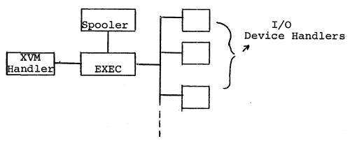
The executive is a multi-tasking monitor for the PDP-11/10 which interfaces identically through its XVM handler to either XVM/RSX or XVM/DOS. This allows the XVM central processor to be switched from either operating system to the other without disturbing Unichannel operation.
