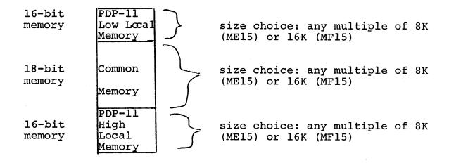
That is, the size of local memory can be configured over a broad range; the starting address and size of common memory can be similarly varied; and the balance of the central processor's physical address space (124K maximum rather than 28K maximum as with the PDP-11/10 can be reassigned to Unibus memory private to the PDP-11 (PDP-11 high local memory). In turn, the PDP-11 memory management registers allow PDP-11 virtual addresses to be mapped onto physical addresses in a variety of ways.
