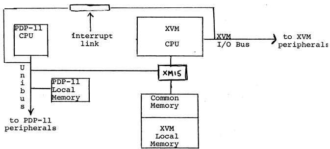
The systems are joined first by an interrupt link which allows either CPU to interrupt the other, and second through sharing of common memory. Common memory is 18 bits wide and the RKII-E Unichannel disk controller reads and writes 18-bit data when transferring into or out of common memory. This allows Unichannel to be used as a system disk or file disk for the XVM system.
