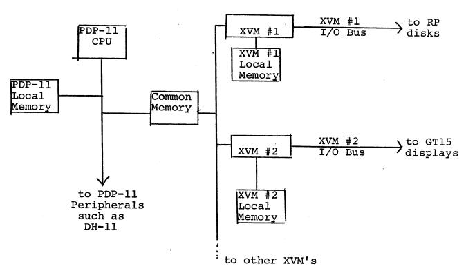
In this example XVM #1 serves as a disk-based multi-task computation system; XVM #2 serves as a controller for multiple GT15 interactive displays and joins these to the computational system, and the PDP-11 serves as a terminal concentrator and line printer and plotting subsystems.
