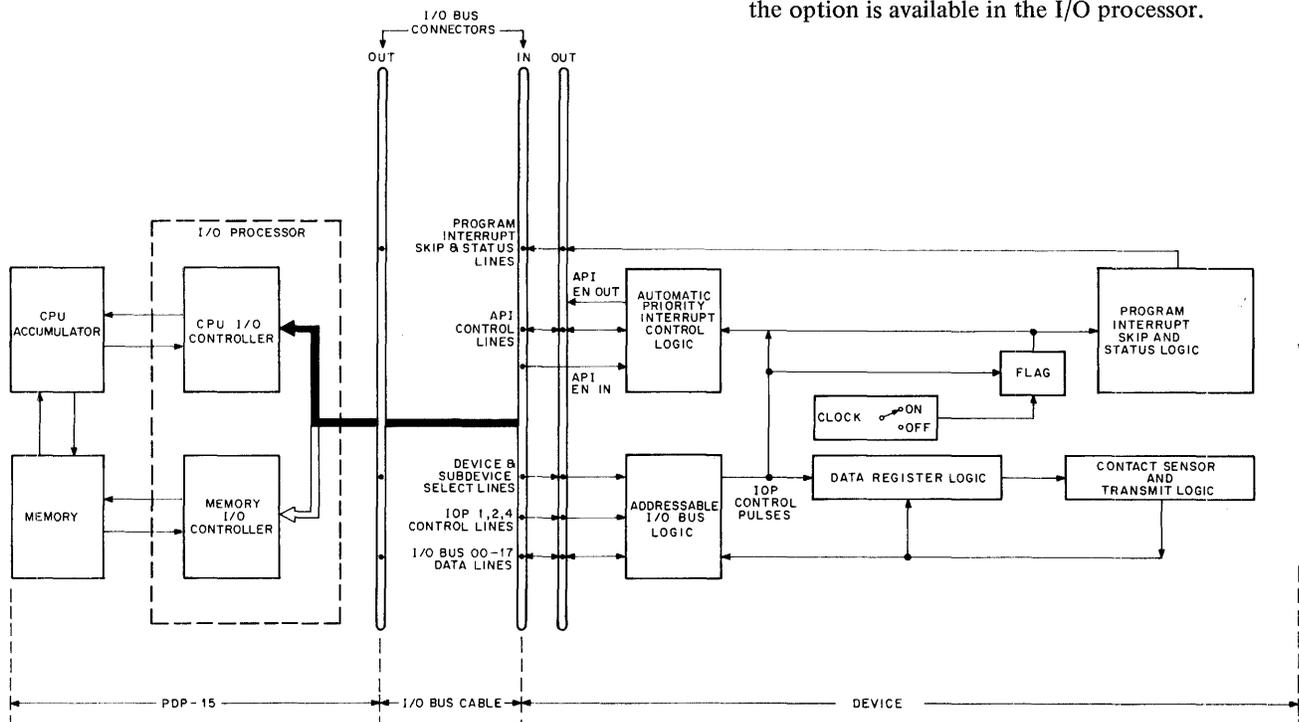
Figure 4-2 Block Diagram of CPU Device with API
