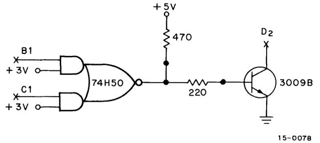
Figure 2-13 M622 Schematic
