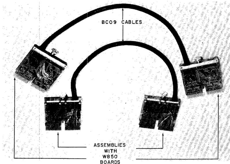
**Figure 6-2** BC09A Cable Assembly
