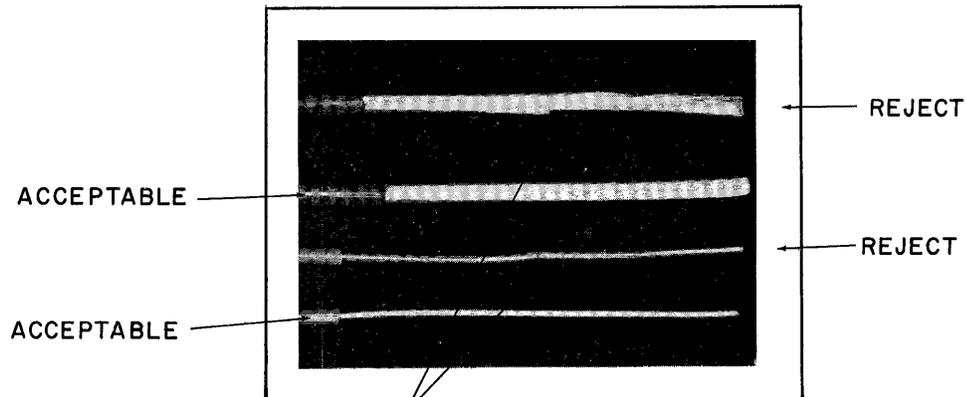
CONDUCTOR IS NICKED BY AN IMPROPERLY ADJUSTED WIRE STRIPPER.
