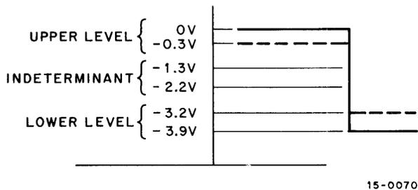
Figure 2-1 Voltage Spectrum of Negative Logic Systems
