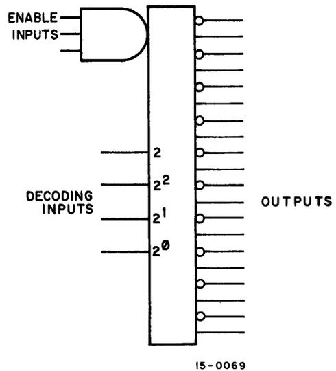
Figure 1-14 Binary to Decimal Decoder
