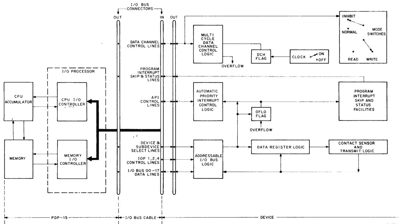
Figure 4-5 Block Diagram for Multicycle Data Channel Device
