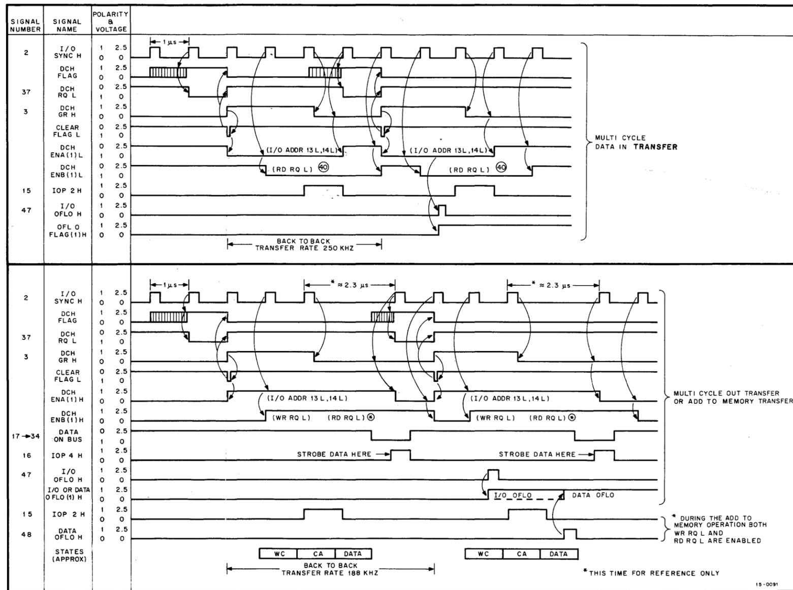
Figure 4-7 Multi-Cycle Data Channel Timing
