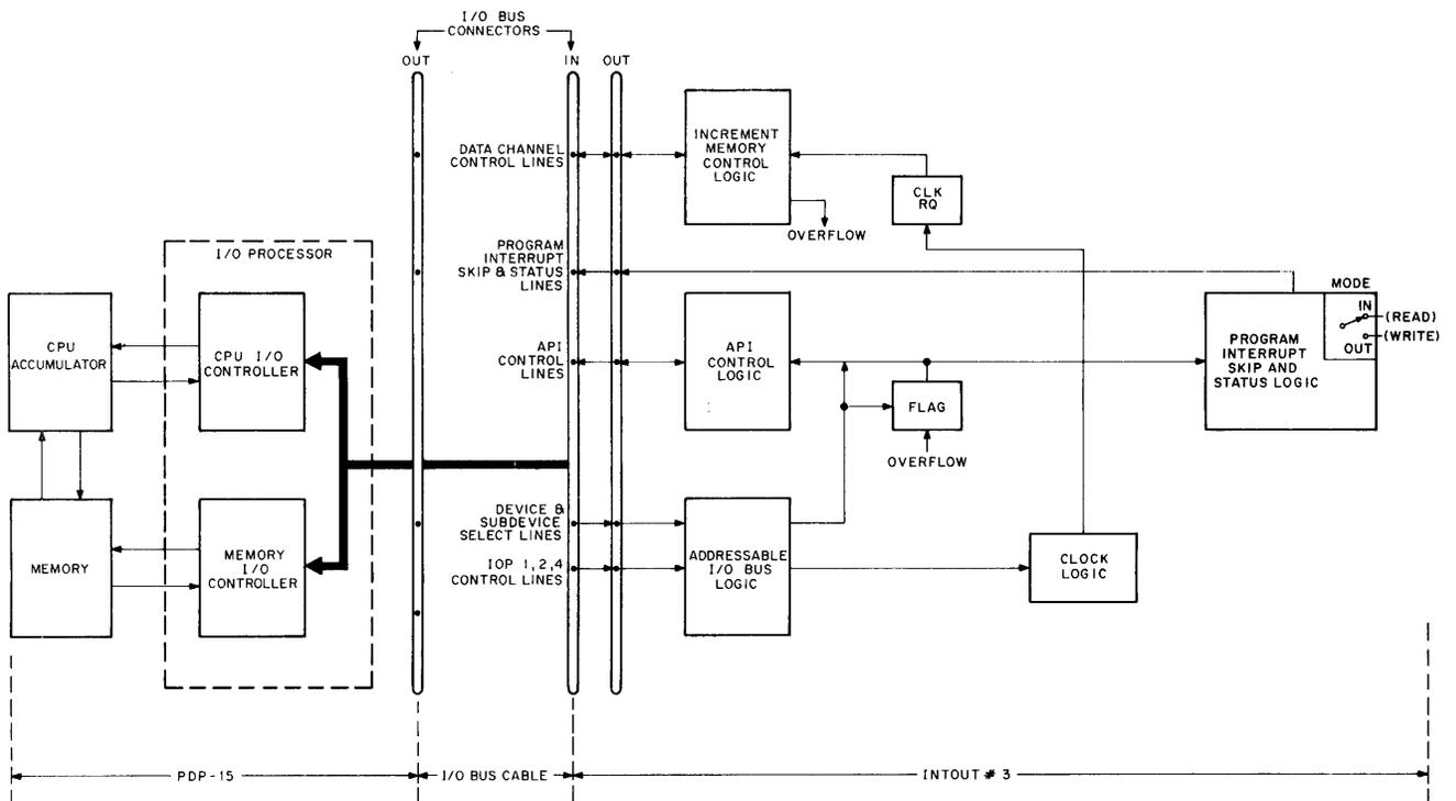
Figure 4-8 Block Diagram for Increment Memory
