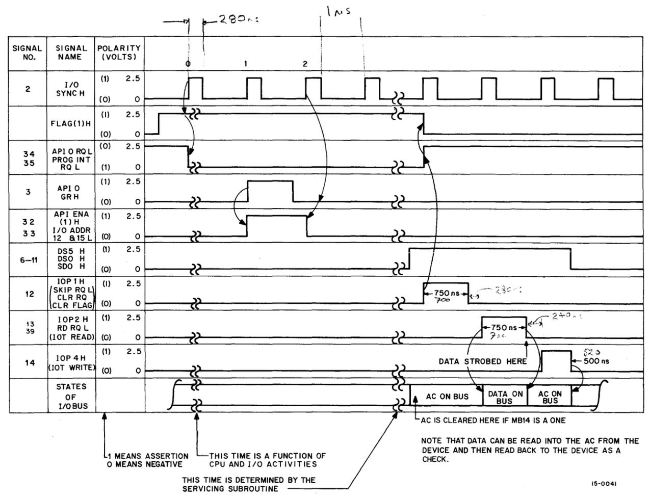
Figure 4-4 Timing Diagram of the CPU Device with API
