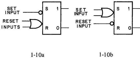
Figure 1-10 R-S Flip-Flop
