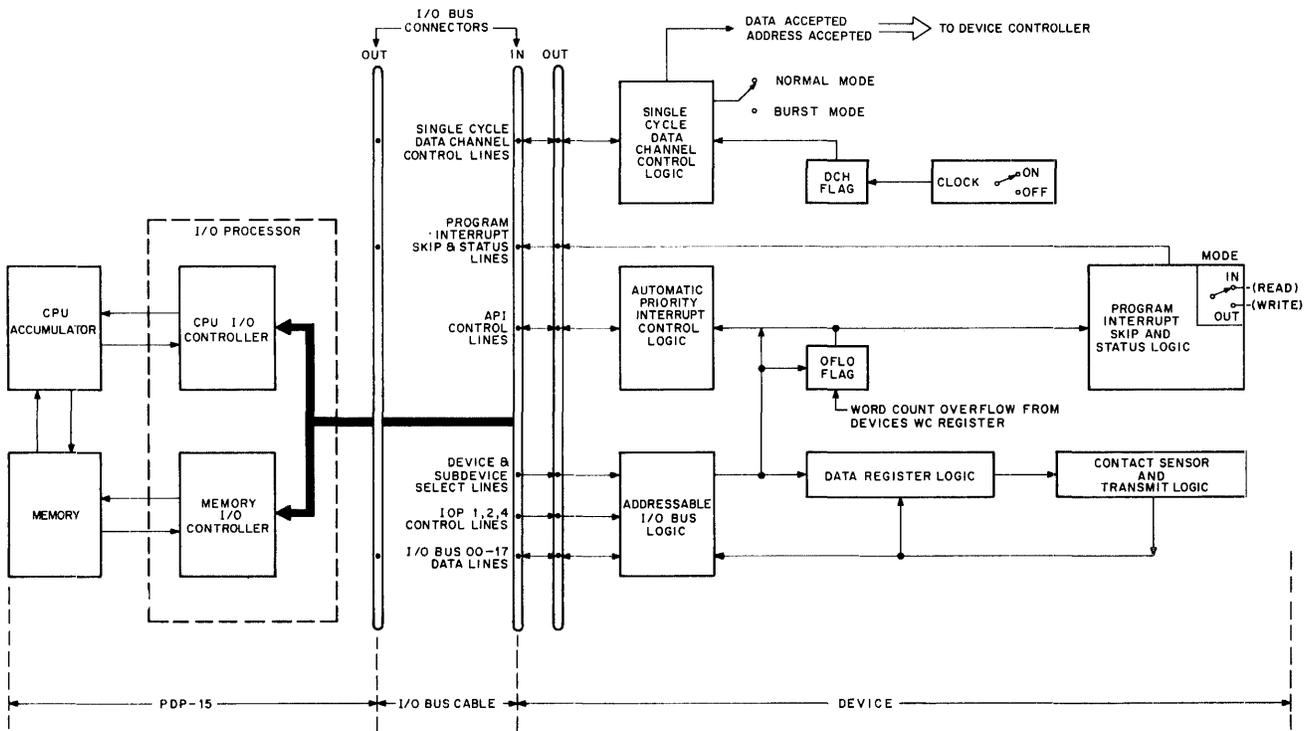
Figure 4-11 Block Diagram of Single-Cycle Data Channel Device
