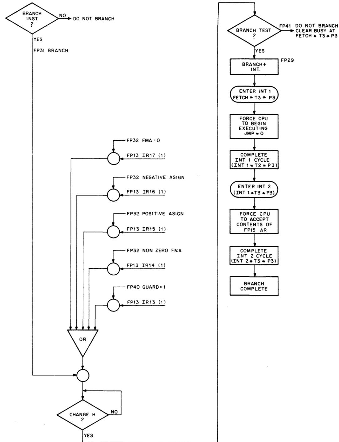
Figure 4-9 Branch Instruction Flow Diagram
