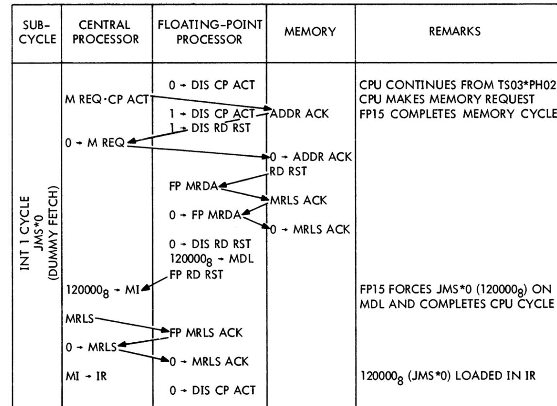
Figure 3-5 INT 1 Cycle Interface Diagram
