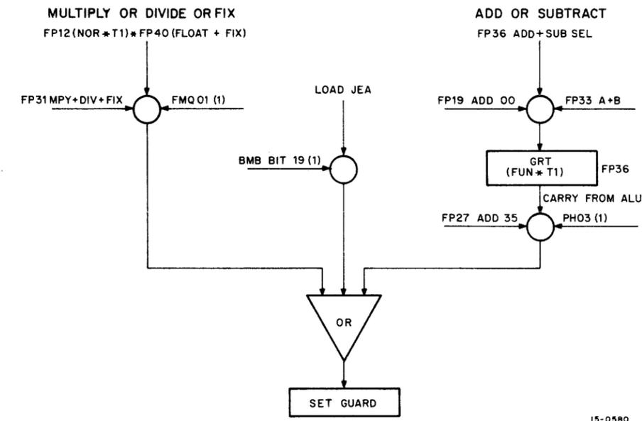
Figure 4-3 Flow Diagram for Setting Guard
