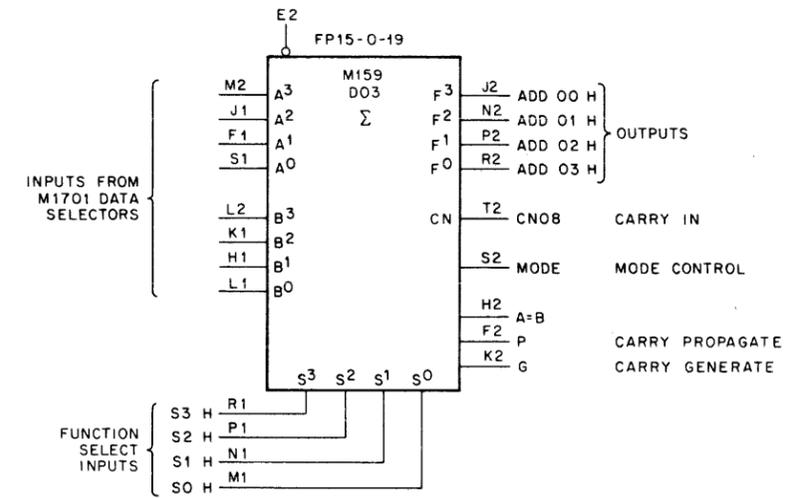
Figure 2-2 M159 Arithmetic Logic Unit
