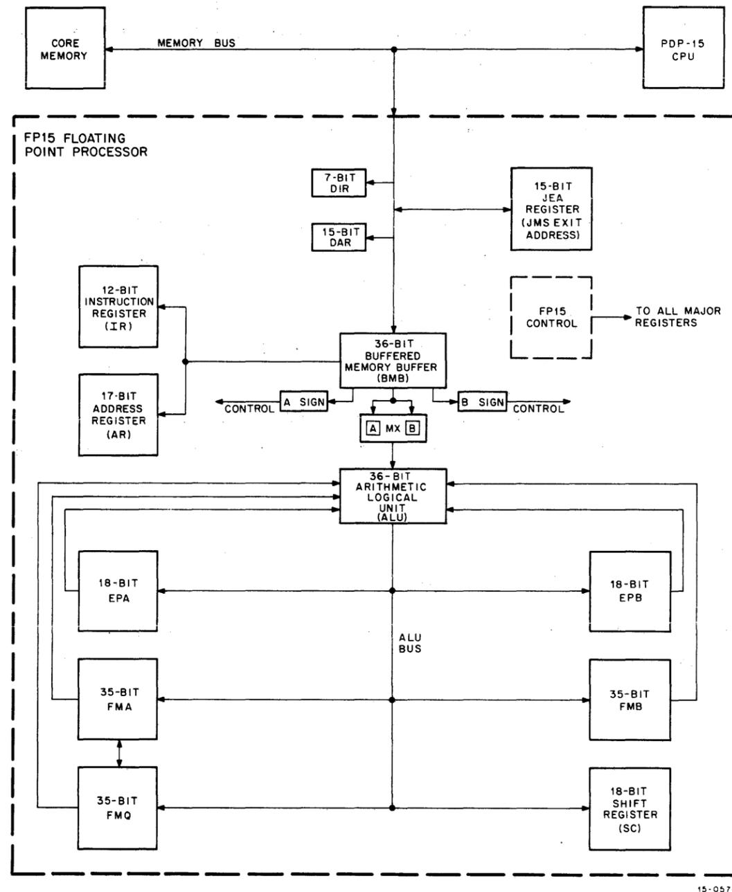
Figure 1-3 FP15 Functional Block Diagram
