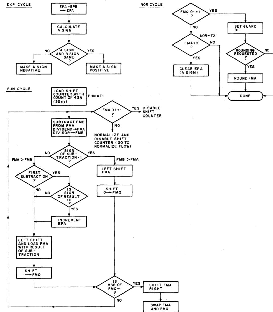
Figure 4-6 Floating-Point Divide Simplified Flow Diagram
