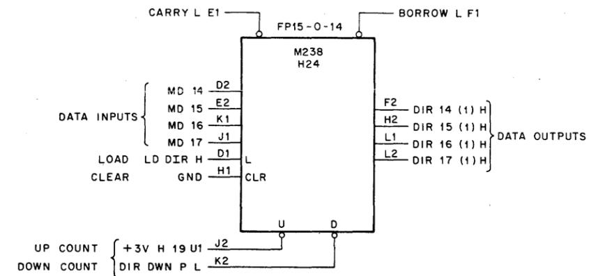
Figure 2-1 M238 Synchronous Up/Down Counter
