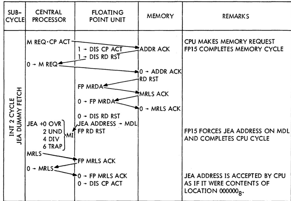
Figure 3-6 INT 2 Cycle Interface Diagram
