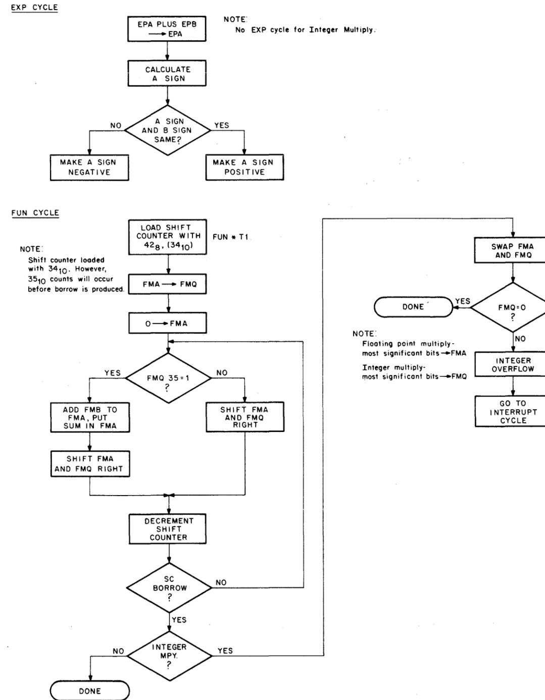
Figure 4-4 Multiply Simplified Flow Diagram
