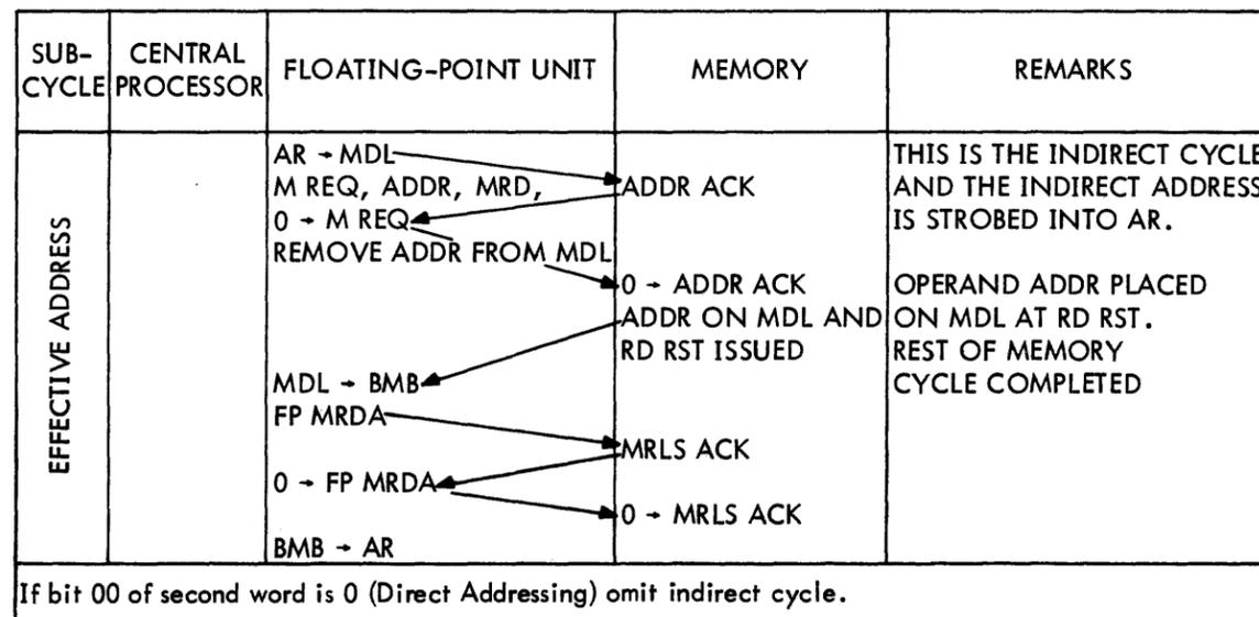
Figure 3-3 Memory Interface--FETCH Cycle (Indirect)
