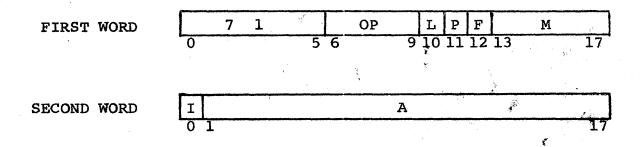
BITS 00-05 OF THE FIRST WORD CONTAIN AN OCTAL "71" TO SPECIFY A FPU INSTRUCTION. THE "71" APPEARS AS A NO-OPERATION IN THE CPU.
