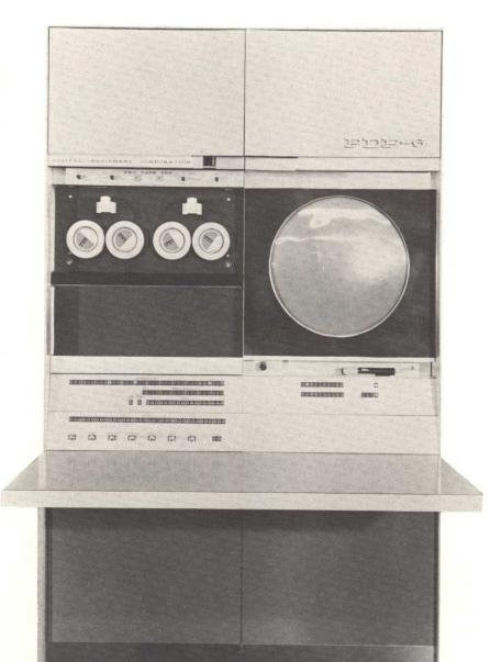
Programmed Data Processor-6 is a medium scale general purpose computer with a high operating speed, unique logical organization, and growth capability. It is designed for use as a research tool in controlling experiments, collecting data, and automatically analyzing data. In addition, the computer is exceptionally well suited for use in scientific computation centers. The PDP-6 prototype is now under construction, and production deliveries will begin in early 1964.
