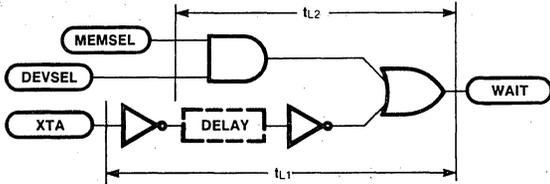
Figure 23: Memory And Input Transfer Wait Circuit
