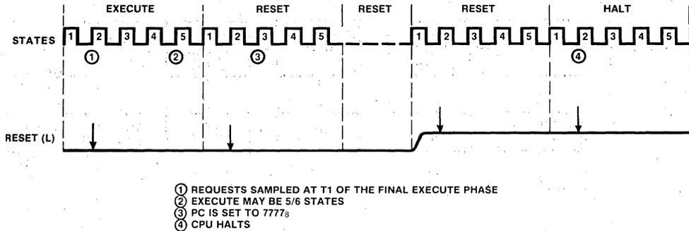
Figure 19: Reset Timing
