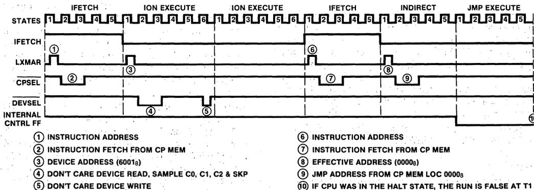
Figure 16: "ION; JMP I 0000" In Control Panel Routine
