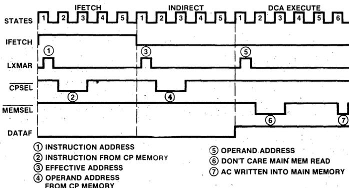
Figure 15: "DCA Indirect" In Control Panel Routine
