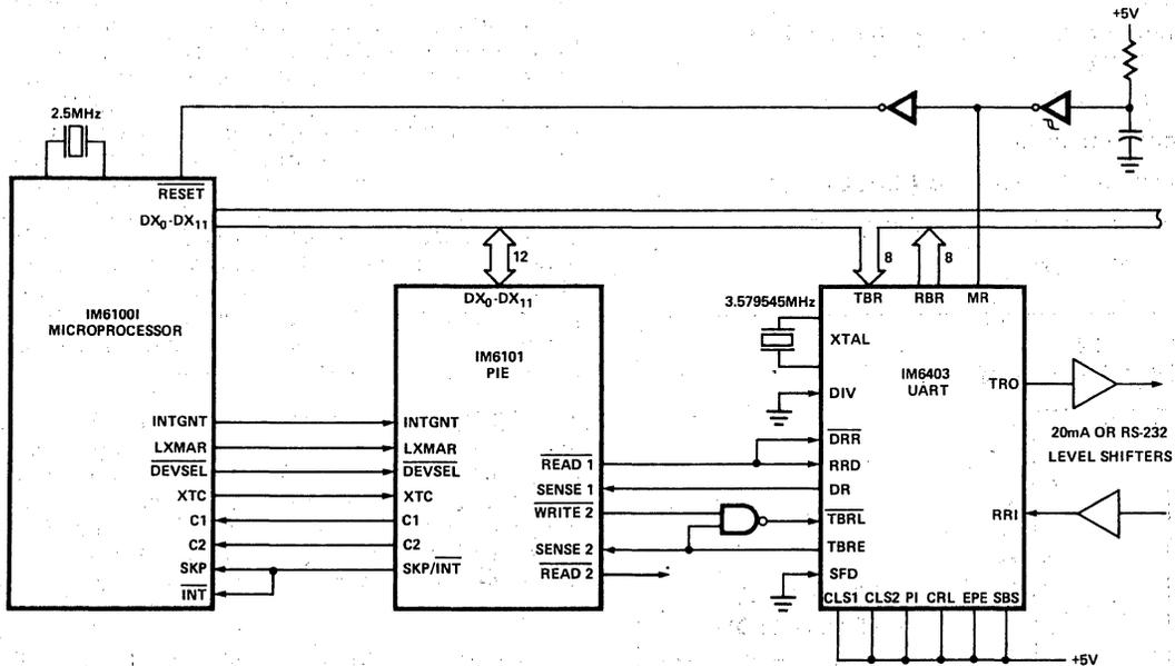
FIGURE 11. 110 Baud Serial Interface for IM6100 System
