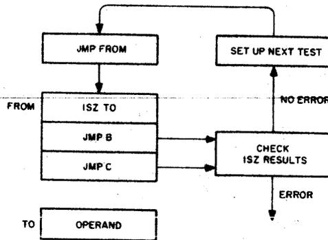
Part 1 of the program uses a random number generator to select the FROM, TO, and OPERAND numbers. Once selected, the OPERAND is incremented until it reaches zero. Each ISZ is checked by duplicating ISZ with TAD, IAC, DCA. Each iteration is also checked for the proper skip or no-skip condition.
