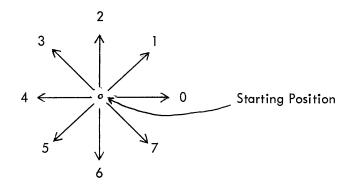
The letter "A" is programmed in subroutine form as an illustration of the use of increment mode.
