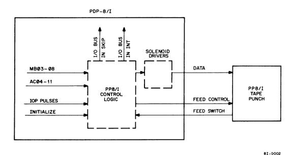
Figure 2 Block Diagram PP8/I Paper-Tape Punch
