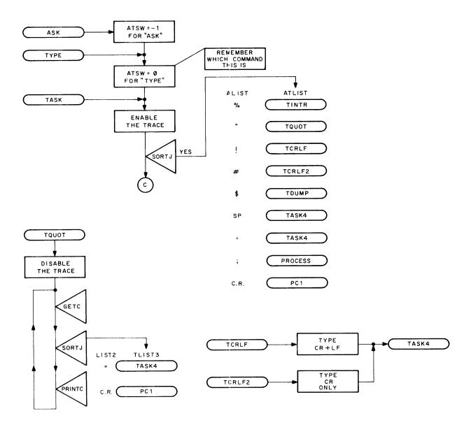
Figure G-5 (Sheet 1) Input/Output Commands
