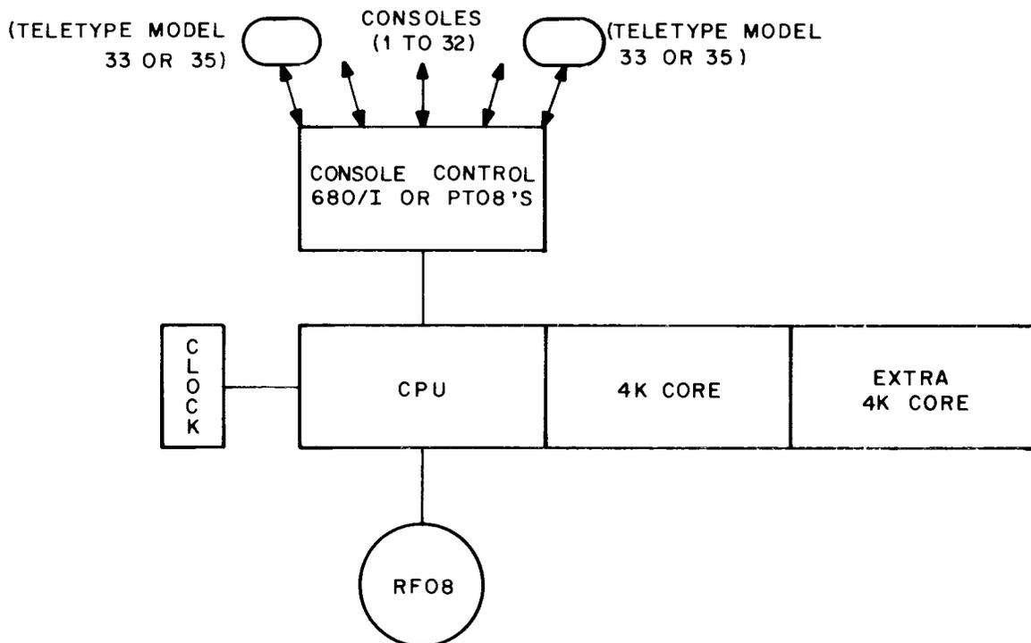
Figure 1-3 System Configuration
