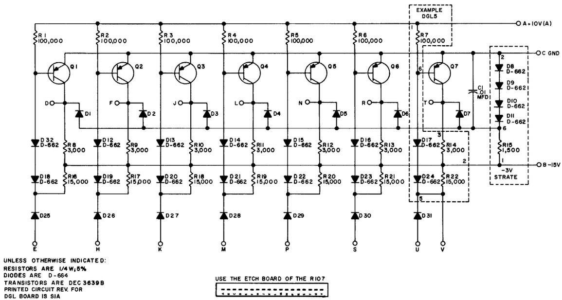
B-CS-S107-0-1 Inverter S107, Circuit Schematic
