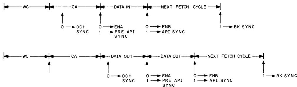
Figure 3-2 API Break Timing Following a DCH Break
