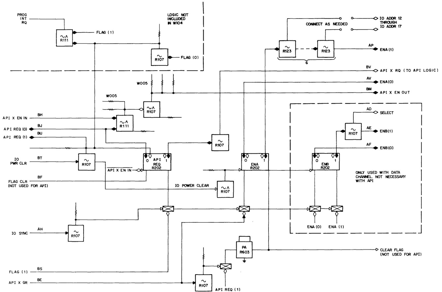
Figure 3-1 Multiplexer W104, Block Diagram
