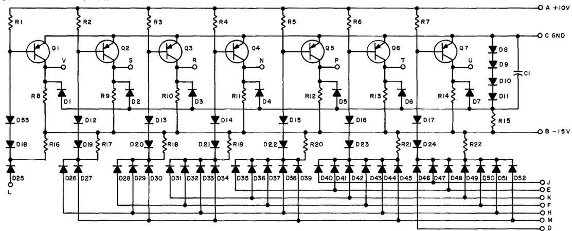
B-CS-S181-0-1 DC Carry Chain S181, Circuit Schematic
