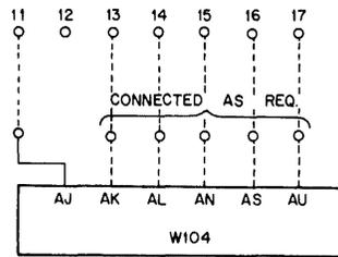
Figure 2-2 Connections for Trap Addresses Between  $100_8$  and  $137_8$
