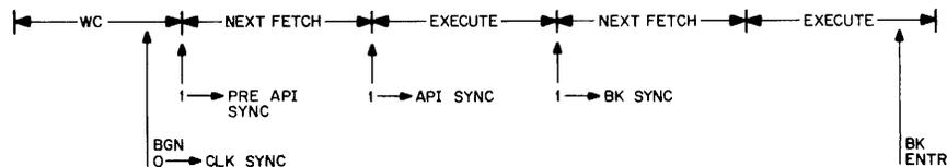
Figure 3-3 API Break Timing following an RTC Break
