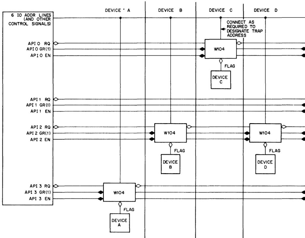
Figure 2-1 Devices on the Automatic Priority Interrupt System
