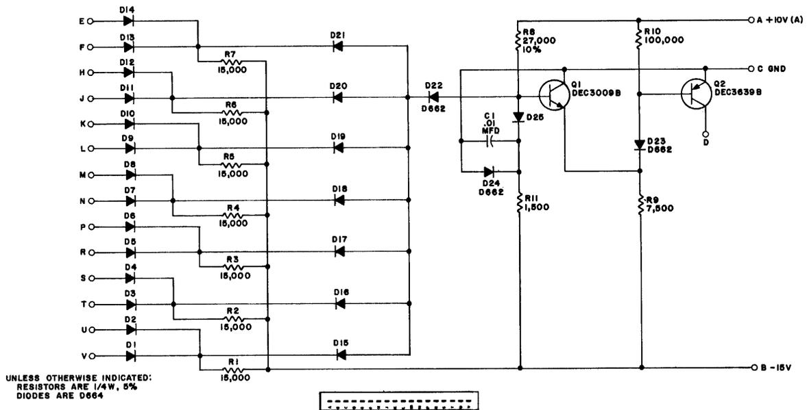
B-CS-R141-0-1 AND/OR Gate R141, Circuit Schematic
