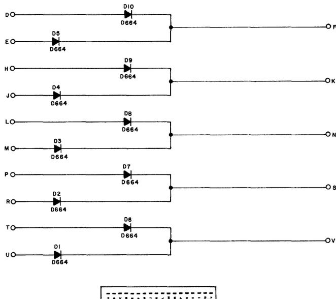
B-CS-R002-0-1 Diode Network R002, Circuit Schematic
