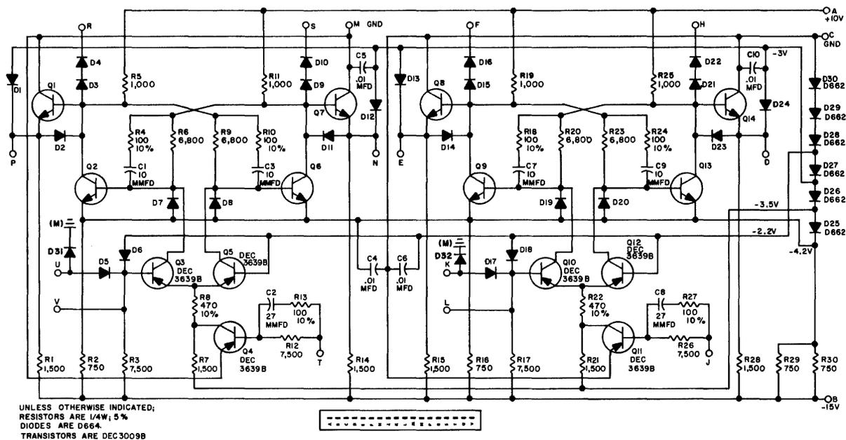
B-CS-B213-0-1 Dual Flip-Flop B213, Circuit Schematic
