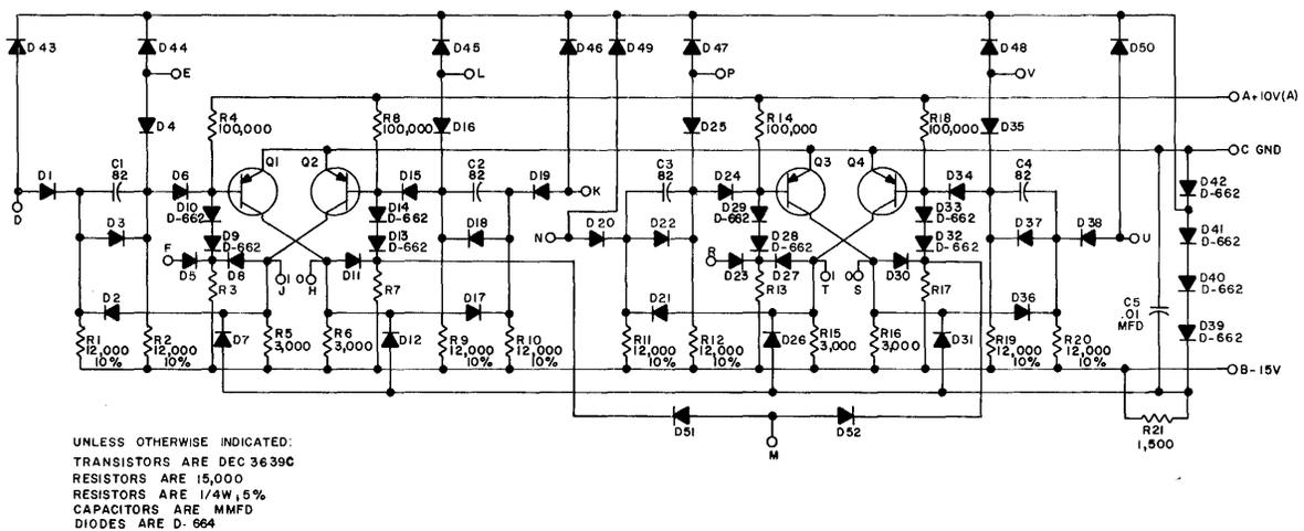
B-CS-S202-0-1 Dual Flip-Flop S202, Circuit Schematic
