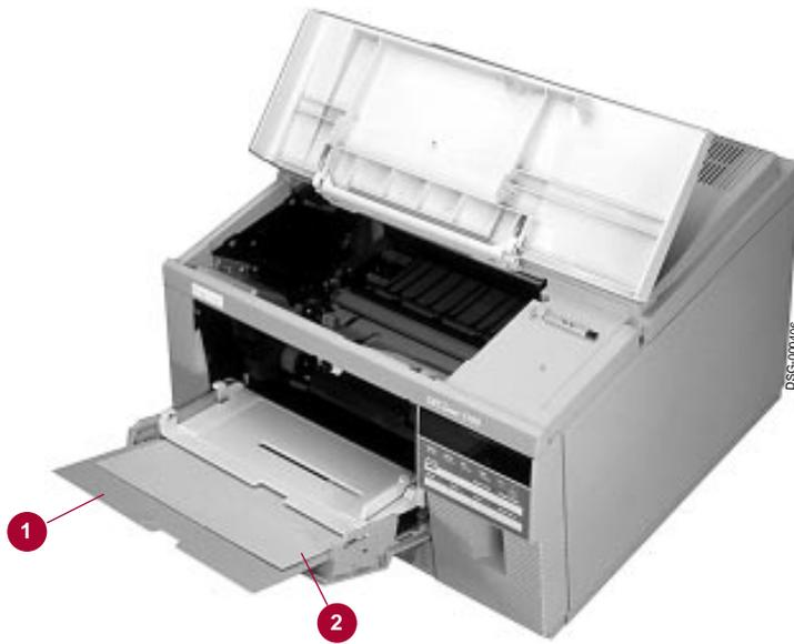
6. Slide the internal tray out all the way from the printer.
