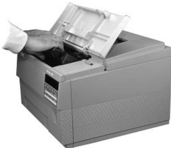
2. Lift the transfer guide up (using the green lever **1**) and remove the jammed paper from the transfer area (or from the tray area **2** if the paper is accessible).
