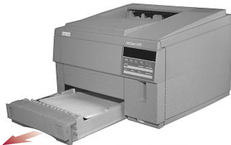
2. Place a stack of paper in the tray ensuring that it lies flat and is below the paper retainers and maximum height arrows.
