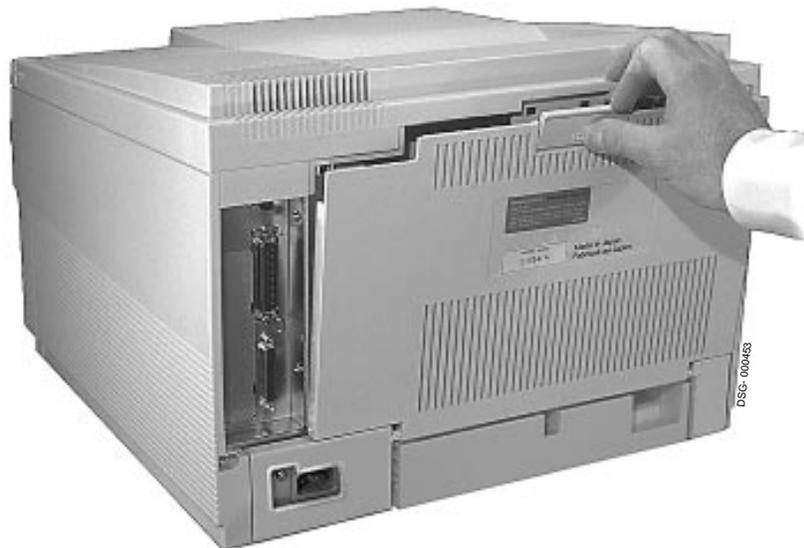
2. Press the green lever ❶ to release the paper then remove the jammed paper from the printer.
