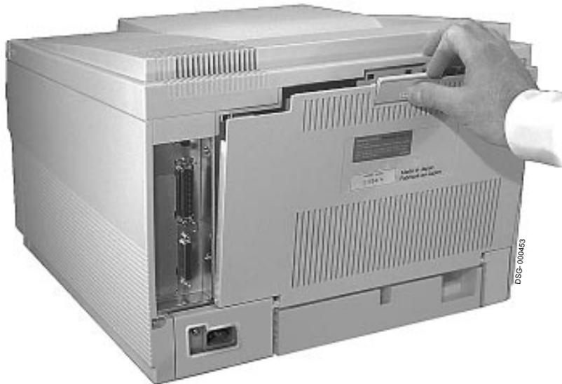
2. Push down on the fusing unit cover ❶ and remove the jammed paper.
