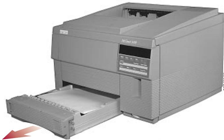
2. Remove jammed paper from the feed rollers in the tray area.
