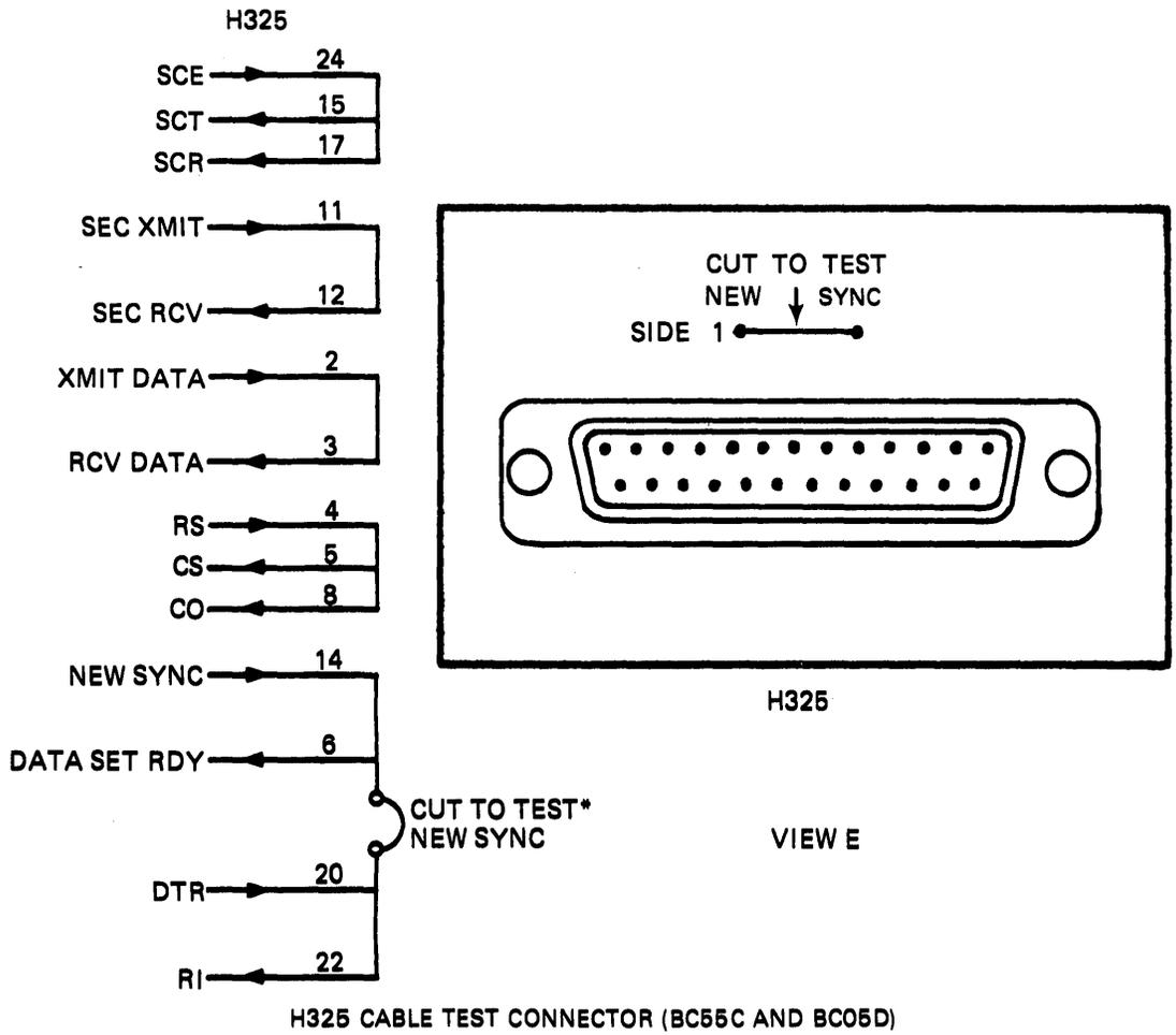
Figure 2-8 DMV11 Test Connectors (Sheet 4 of 4)
