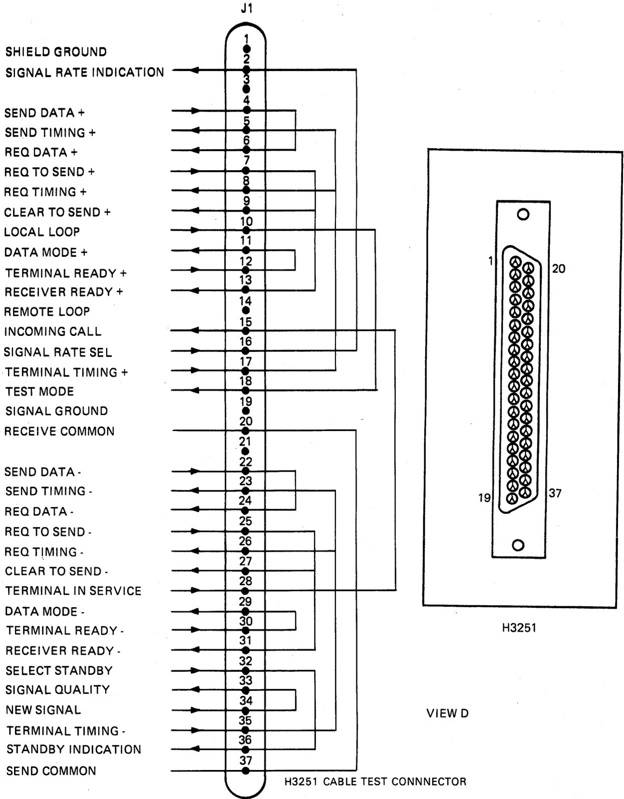
Figure 2-8 DMV11 Test Connectors (Sheet 3 of 4)
