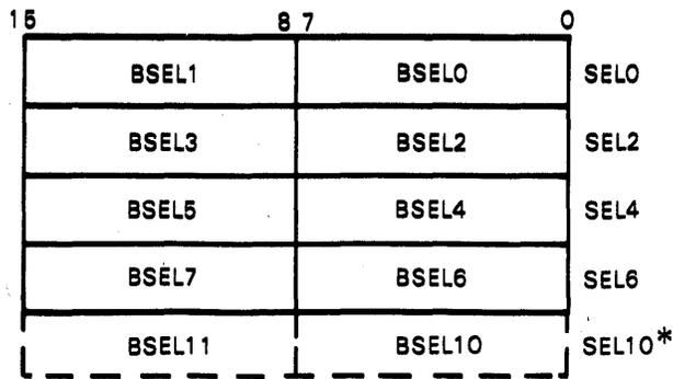
\*SEL10 IS ONLY USED IN 22 BIT ADDRESS MODE
