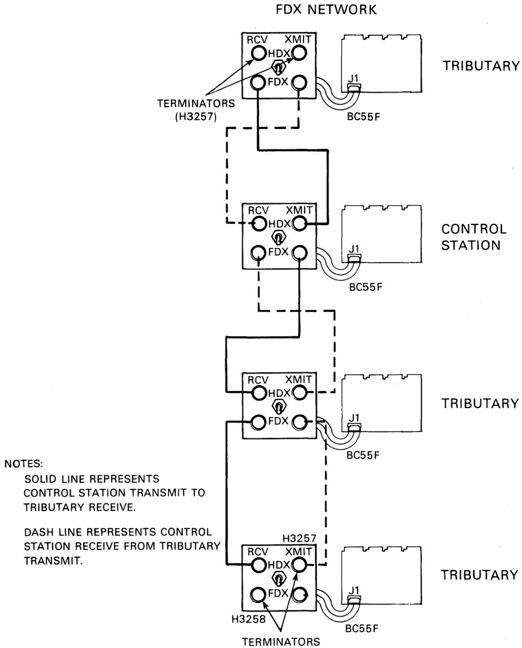
SINCE THE CONTROL STATION IS NOT AN END MODE, THERE IS NEED TO TERMINATE TWO SETS OF TRANSMIT LINES FROM THE CONTROL STATION, ADDITIONALLY BOTH ENDS OF THE TRANSMIT LINE FROM THE TRIBUTARIES
