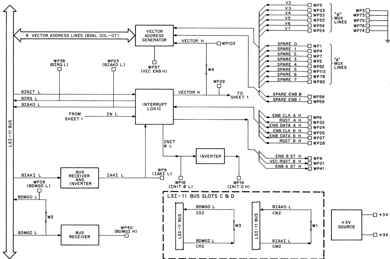
Figure 2 DRV11-P Block Diagram (Vector Address Generator and Interrupt Logic)
