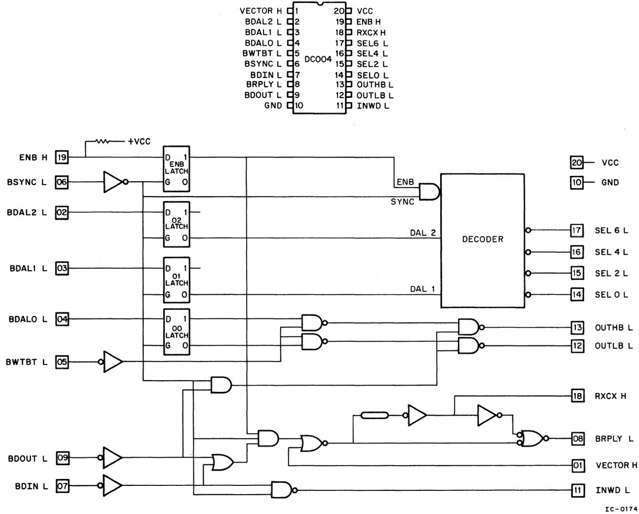
Figure A-4 DC004 Simplified Logic Diagram
