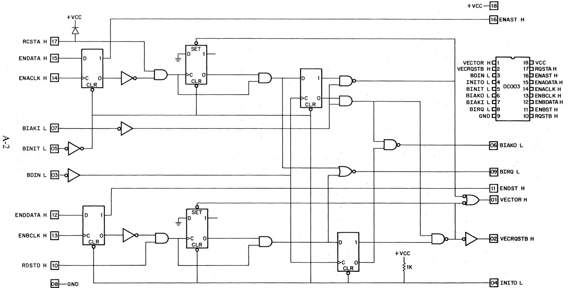
Figure A-1 DC003 Simplified Logic Diagram
