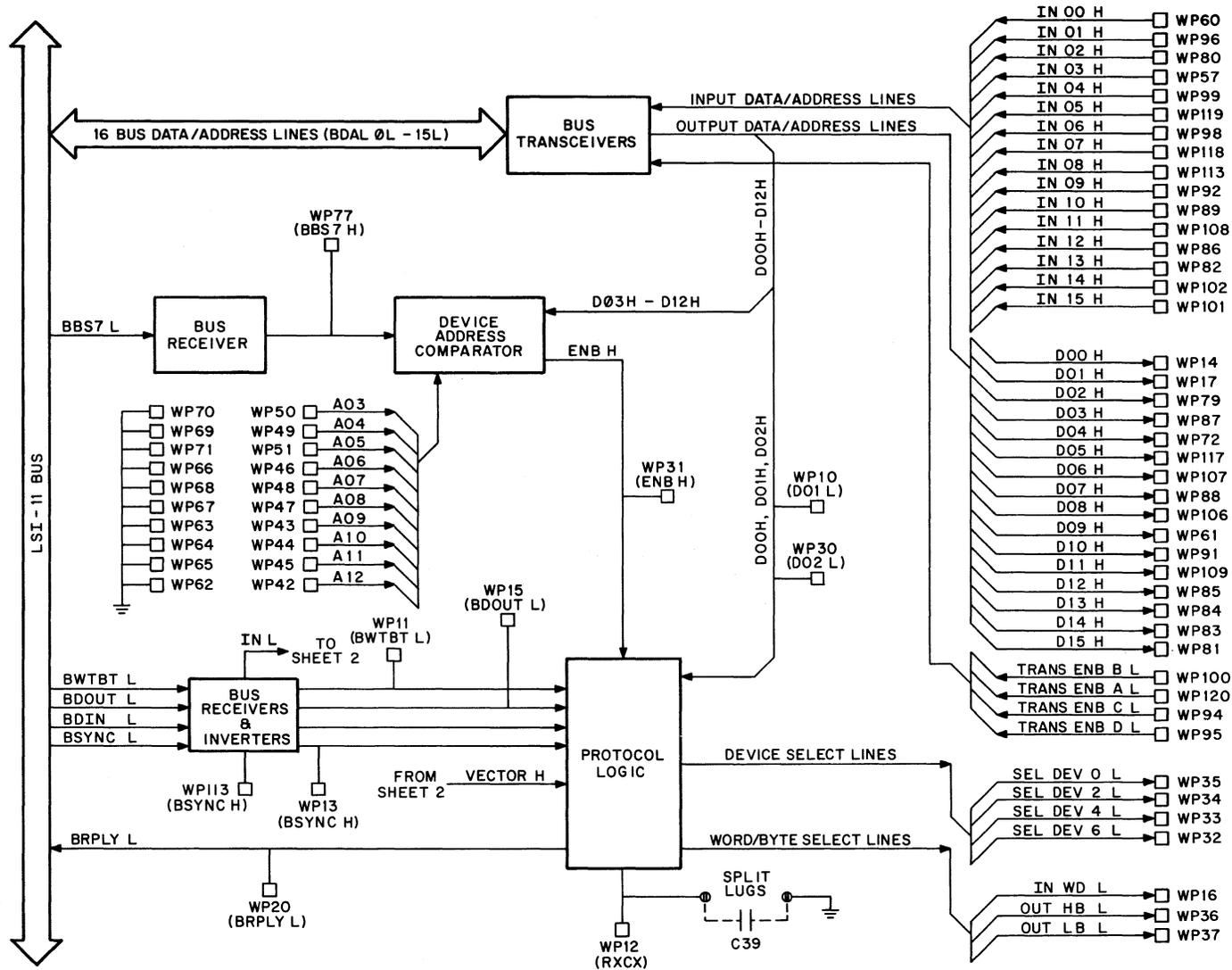
Figure 2 DRV11-P Block Diagram (Bus Transceivers, Device Address Comparator, and Protocol Logic) (Sheet 1 of 2)
