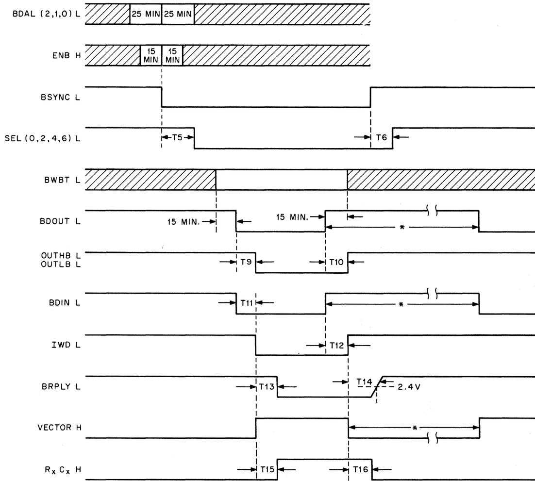
\* TIME REQUIRED TO DISCHARGE R<sub>x</sub> C<sub>x</sub> FROM ANY CONDITION ASSERTED = 150 ns
