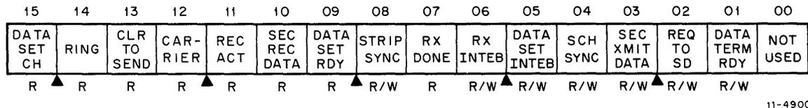
Figure 3-2 Receiver Status Register (RXCSR)
