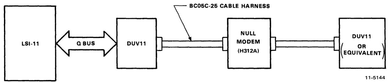
Figure 2-4 DUV11 to Null Modem Connection
