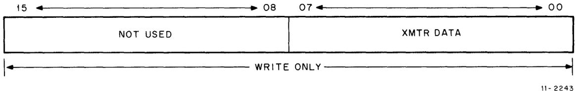
Transmitter Data Buffer Register (TXDBUF)
