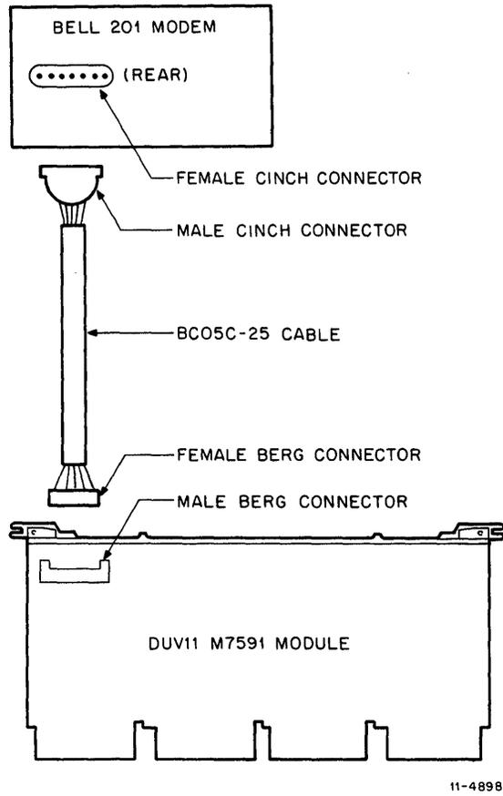
Figure 2-3 DUV11 to Modem Connection
